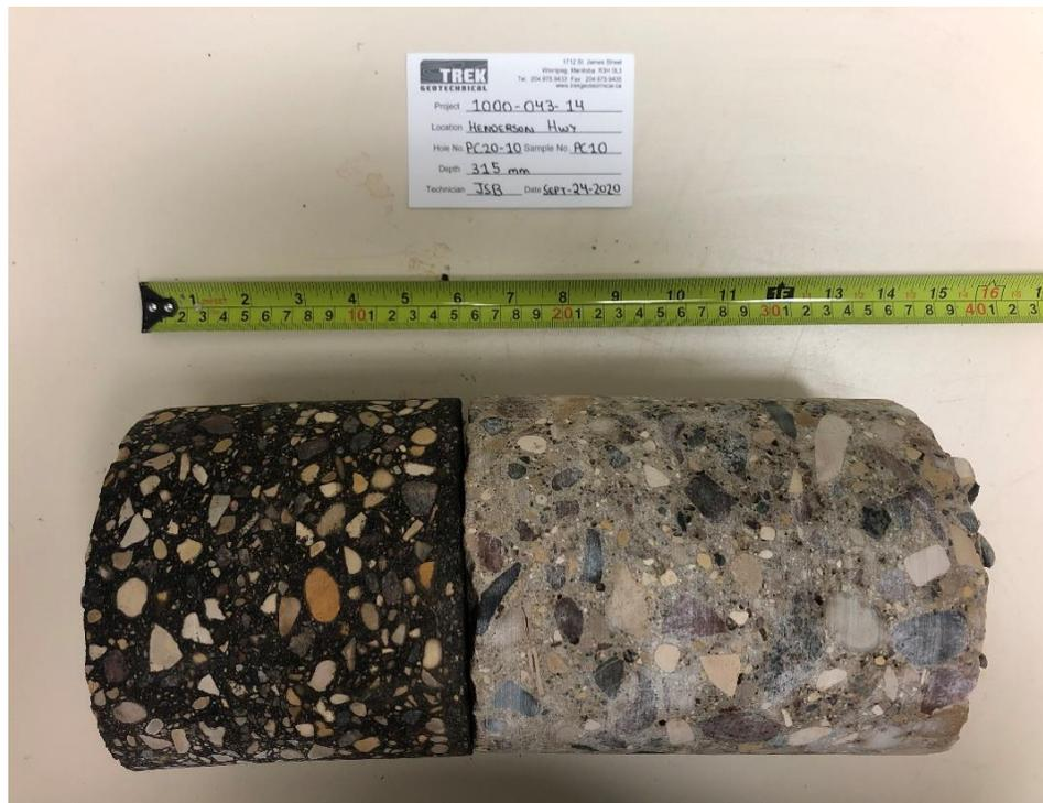
Photo 10: Pavement Core Sample at Pavement Hole PC20-010
