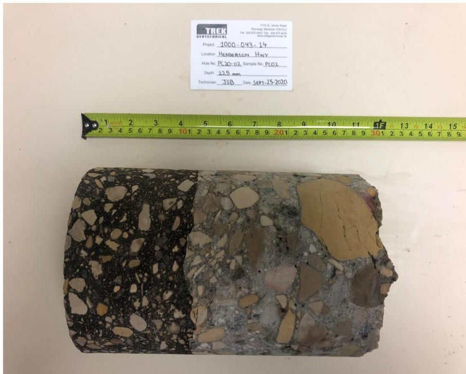
Photo 2: Pavement Core Sample at Pavement Hole PC20-02
