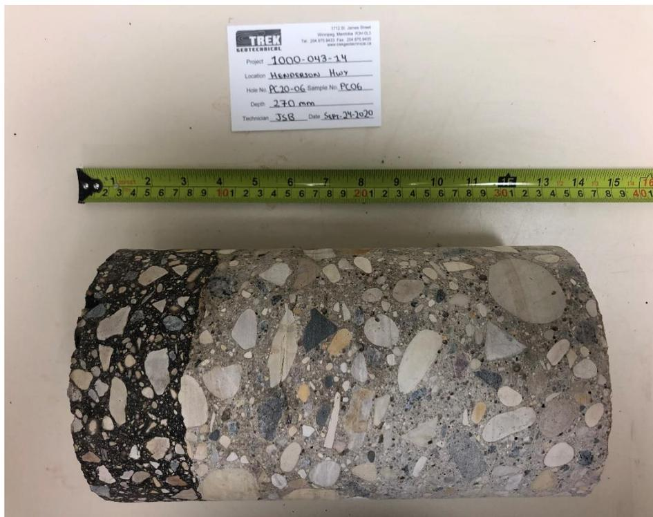
Photo 6: Pavement Core Sample at Pavement Hole PC20-06
