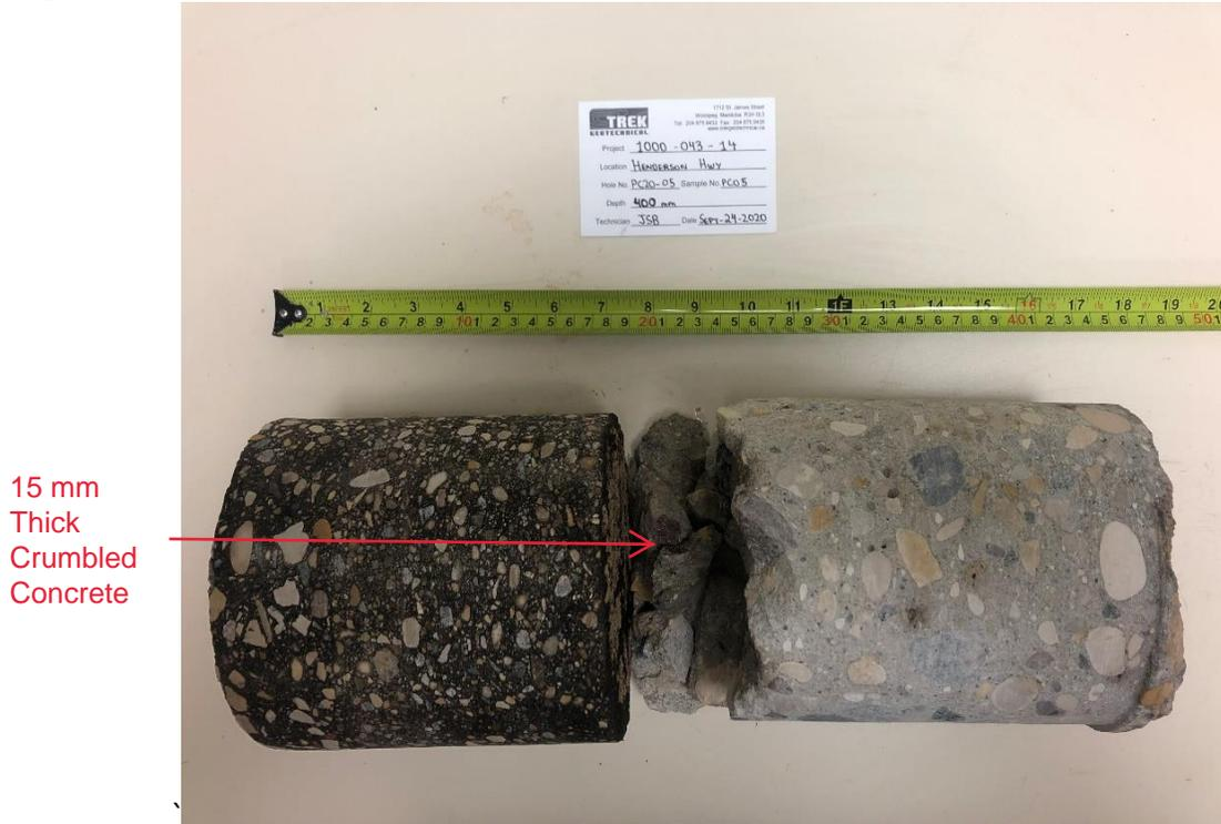
Photo 5: Pavement Core Sample at Pavement Hole PC20-05
