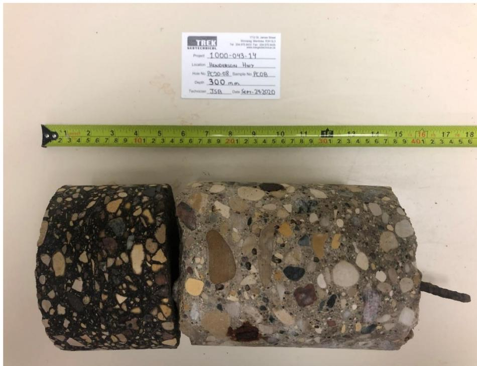
Photo 8: Pavement Core Sample at Pavement Hole PC20-08
