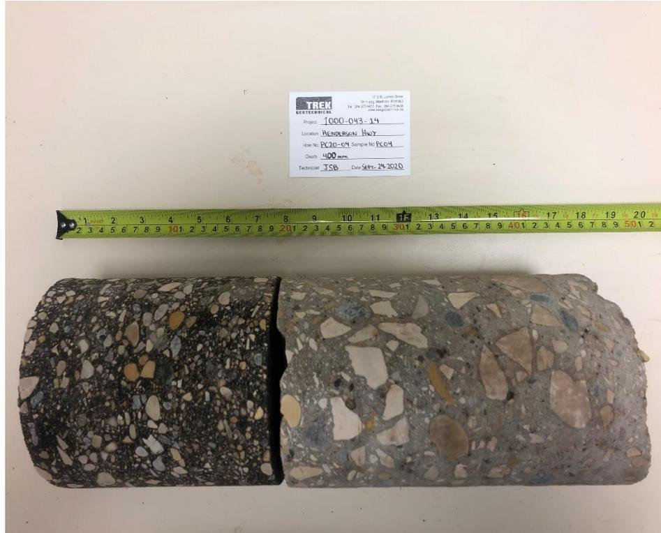
Photo 4: Pavement Core Sample at Pavement Hole PC20-04
