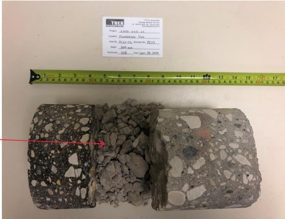
Photo 1: Pavement Core Sample at Pavement Hole PC20-01
