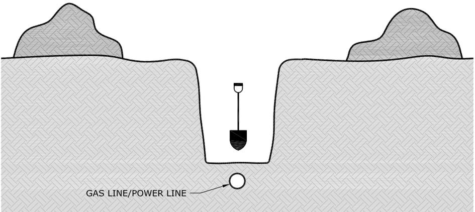
Dig a hole with a shovel directly above the line location until the line is exposed. Take care not to damage the line or coating. Mechanical excavation equipment **MUST NOT** be used to widen or deepen the hole before exposing the line.
