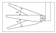
RM - Optional rigid knuckle mount for downward facing, fixed applications. Available in standard optic orientation only.
