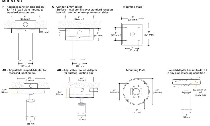
Adjustable Sloped Adapter that can mount in any axis due to ball and socket joint. Available for recessed junction box or surface junction box.
