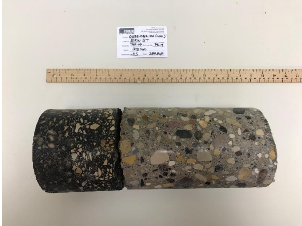
Photo 7: Pavement Core Sample at Test Hole TH19-07
