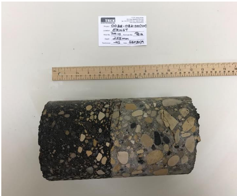
Photo 10: Pavement Core Sample at Test Hole TH19-10
