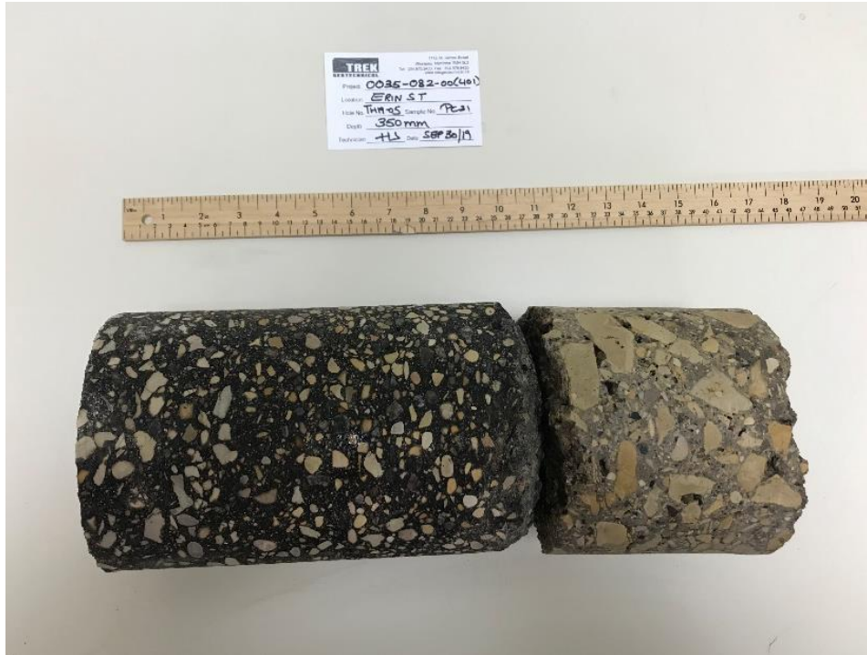
Photo 5: Pavement Core Sample at Test Hole TH19-05
