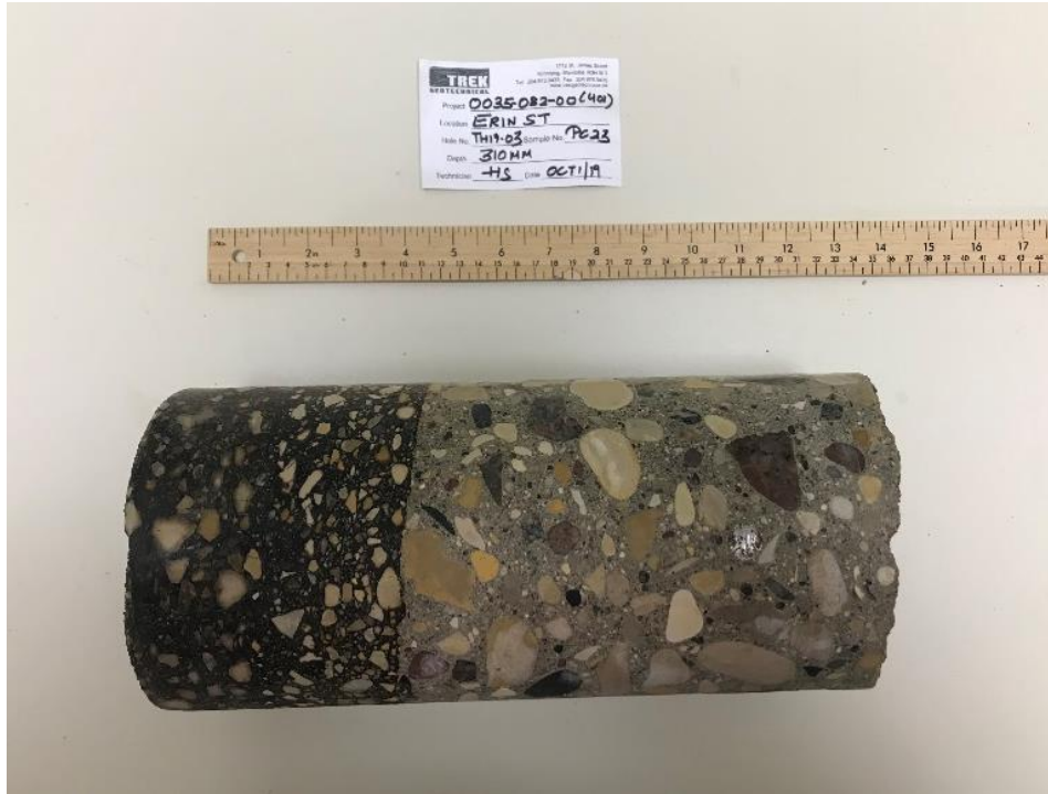
Photo 3: Pavement Core Sample at Test Hole TH19-03
