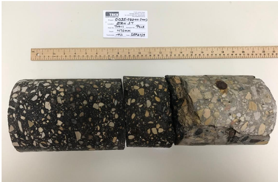
Photo 11: Pavement Core Sample at Test Hole TH19-11
