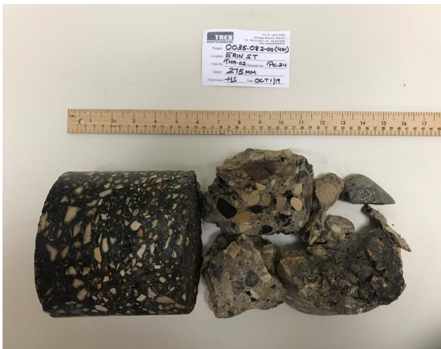
Photo 2: Pavement Core Sample at Test Hole TH19-02
