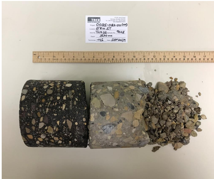
Photo 23: Pavement Core Sample at Test Hole TH19-23
