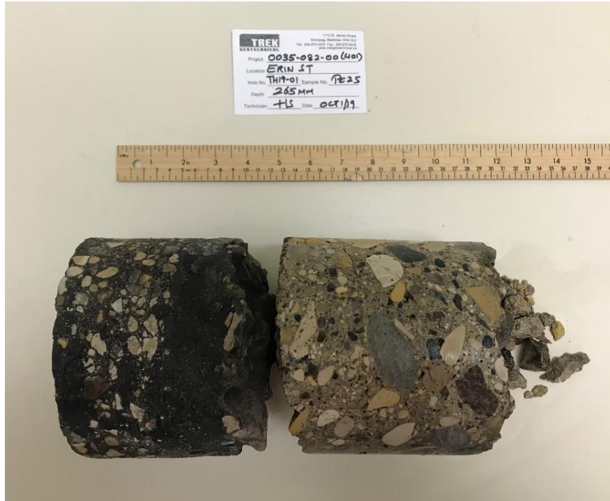
Photo 1: Pavement Core Sample at Test Hole TH19-01
