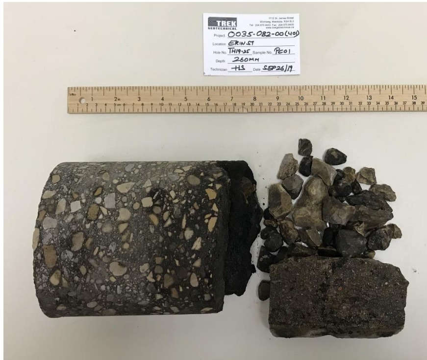
Photo 25: Pavement Core Sample at Test Hole TH19-25
