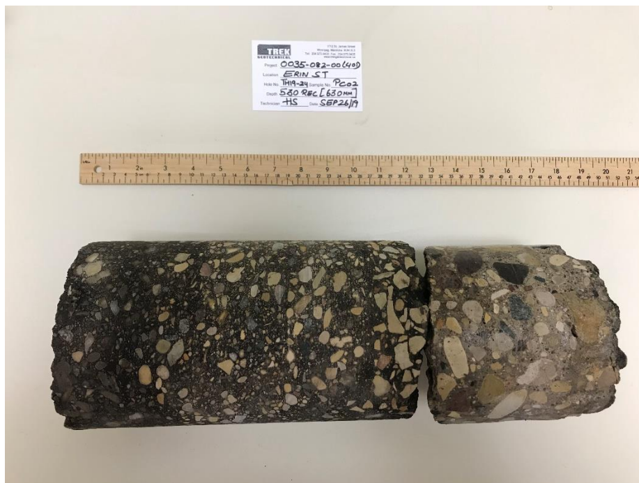
Photo 24: Pavement Core Sample at Test Hole TH19-24
