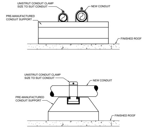
**7 TYPICAL ROOF CONDUIT SUPPORT DETAIL (ELECTRICAL)**
