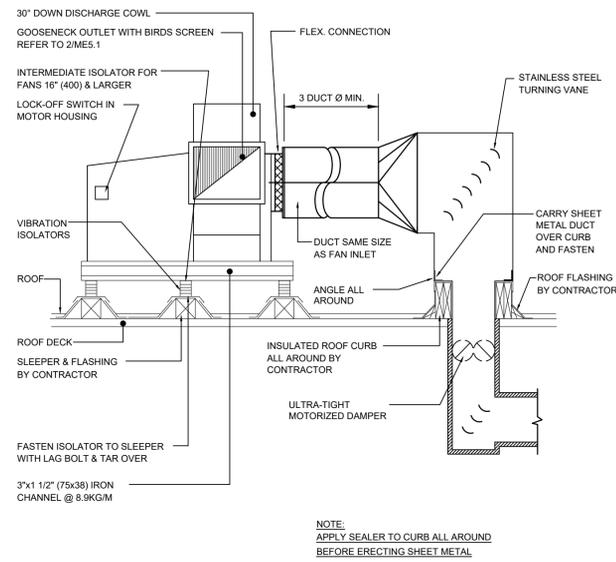
**1 CENTRIFUGAL ROOF EXHAUST FAN (MECHANICAL)**
