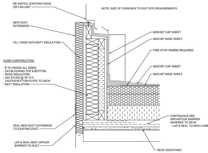
**4 ROOF CURB @ EXHAUST DUCT DETAIL (MECHANICAL)**
