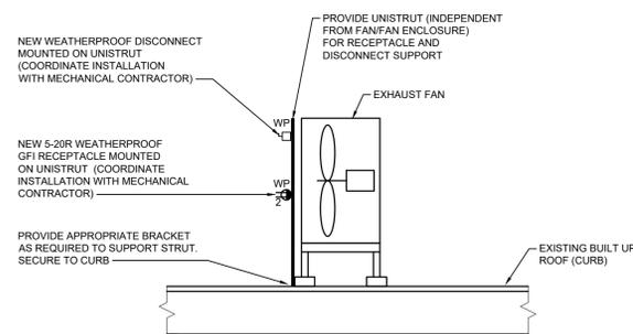
**6 TYPICAL ROOF RECEPTACLE AND DISCONNECT MOUNTING DETAIL (ELECTRICAL)**
