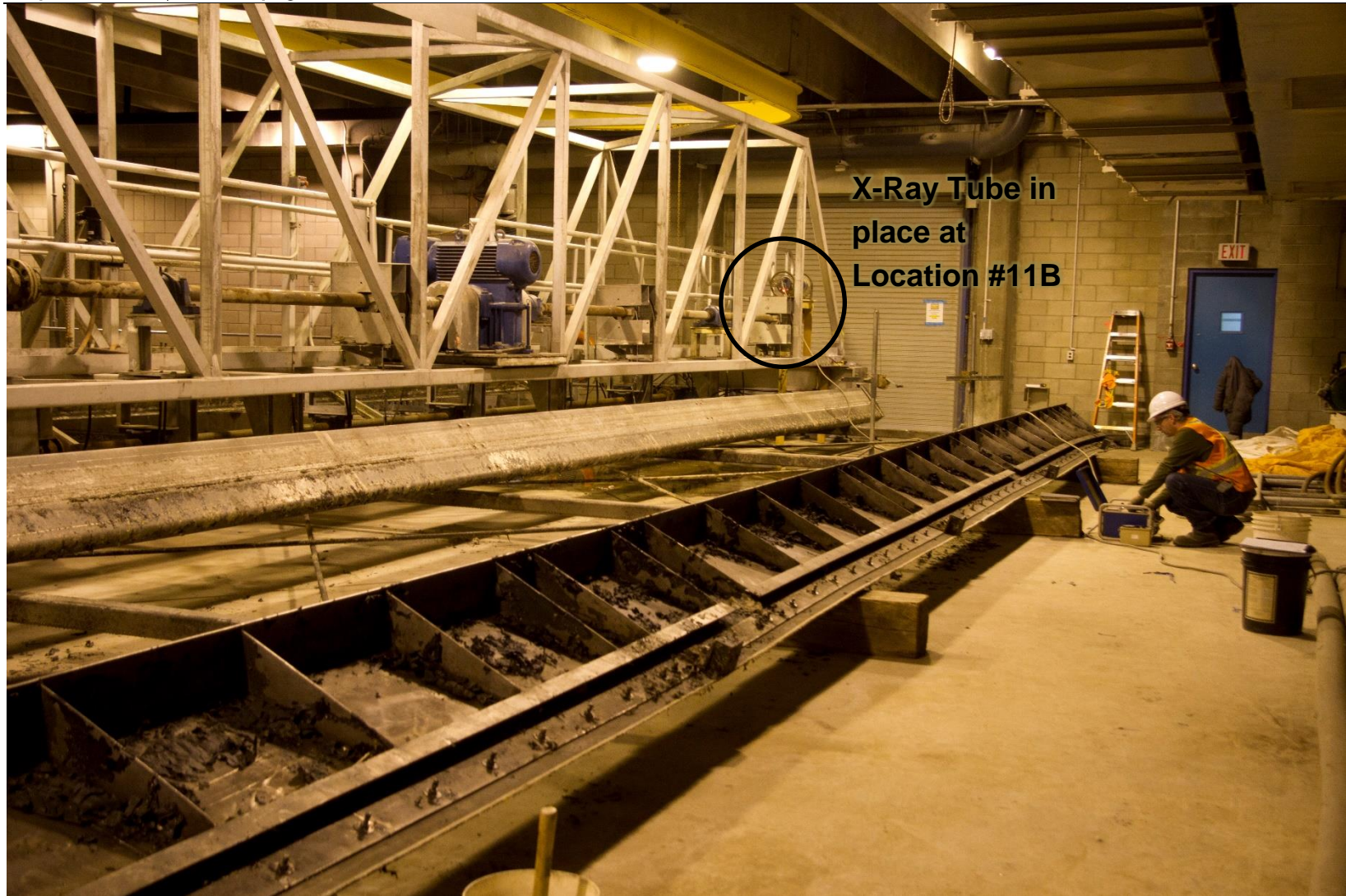
Fig. 14 (cont'd): Radiography at South-West Corner of Bridge
