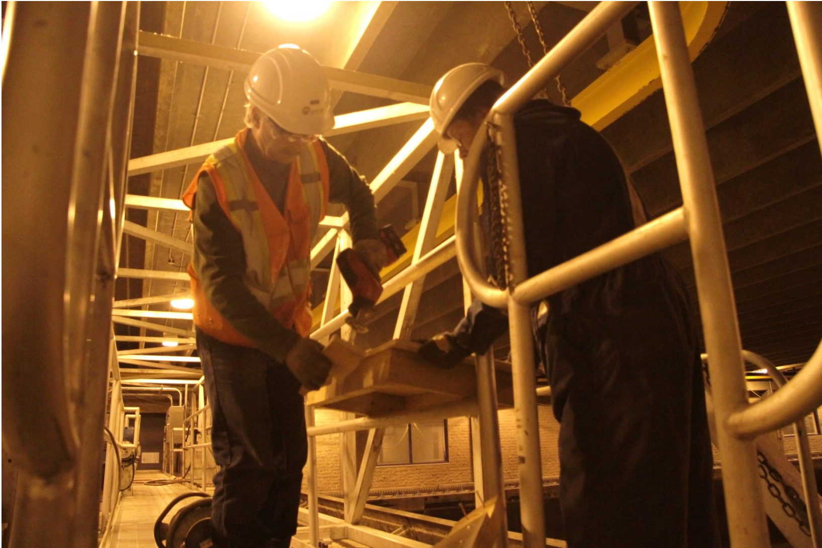
Fig. B-2: X-ray technician using a Sawzall to cut the wooden platform to fit different locations at either end of the bridge. Wooden legs were disassembled and re-positioned to get the x-ray tube into the correct position for the x-ray “shot”
