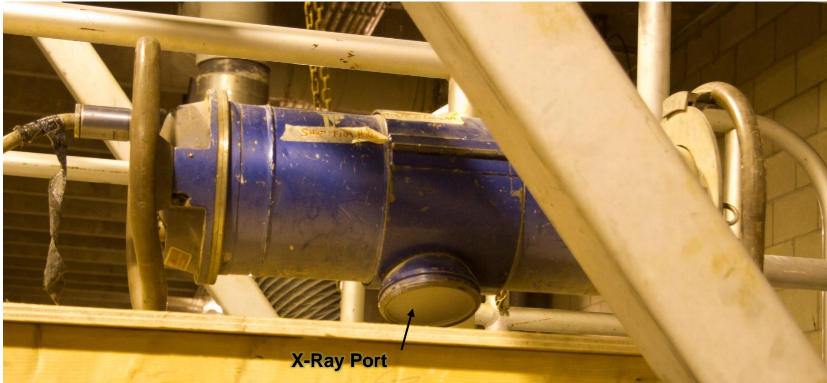
Fig. B-1: View of 100lbs X-ray camera used for radiography of aluminum
