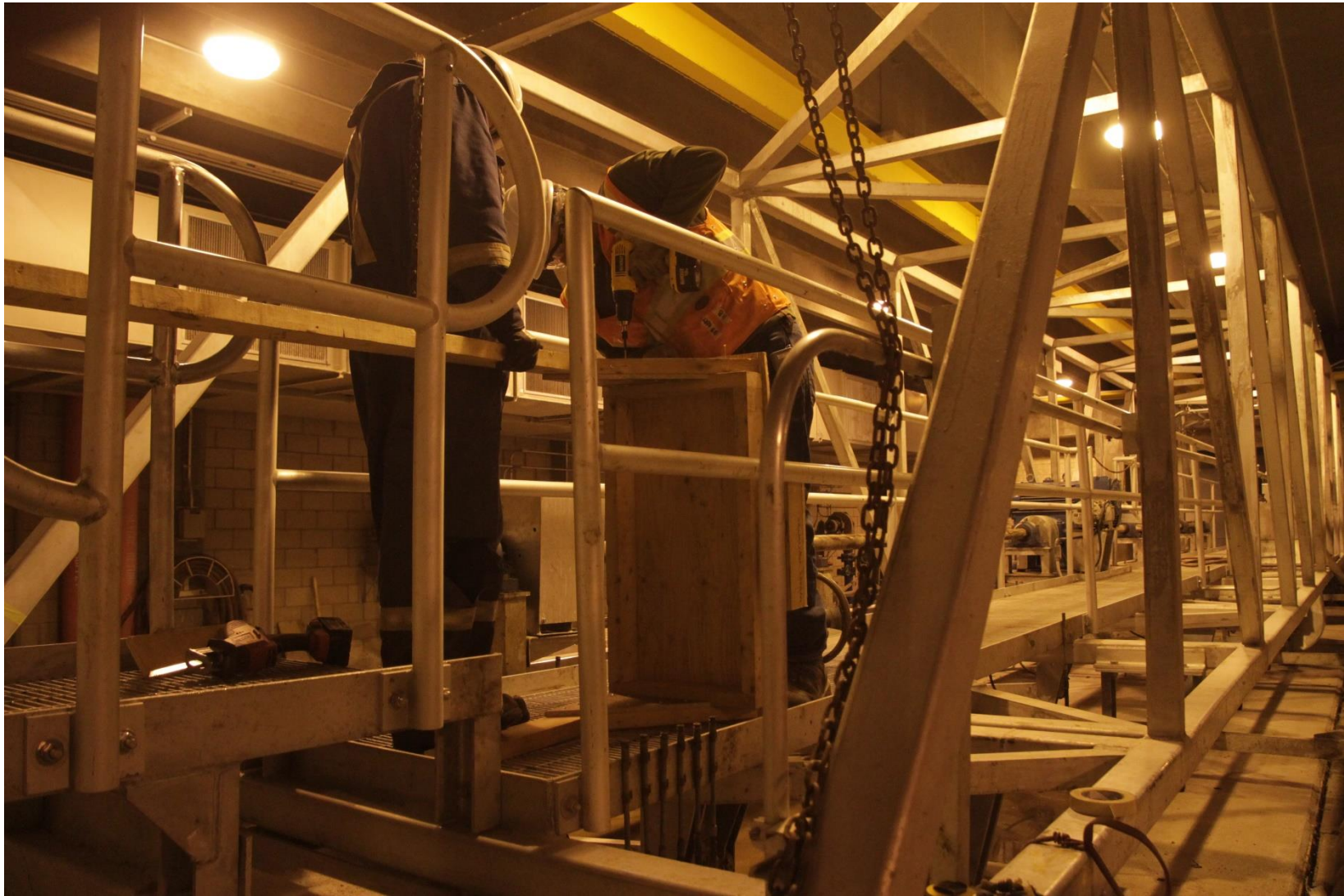
Fig. B-3: X-ray technician re-positioning the legs of the wooden platform to support the electric x-ray tube
