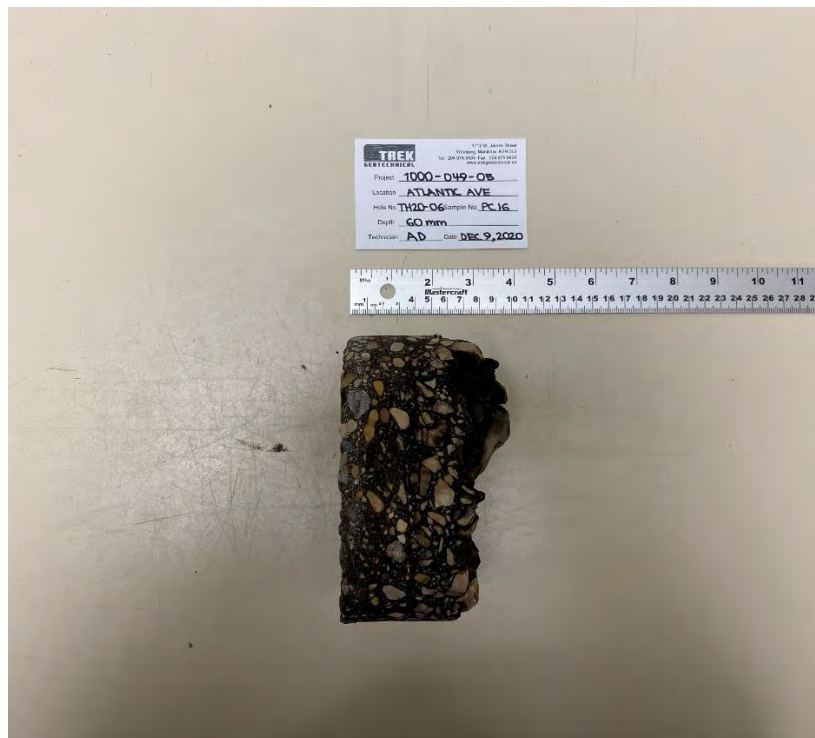
Photo 6: Pavement Core Sample at Test Hole TH20-06
