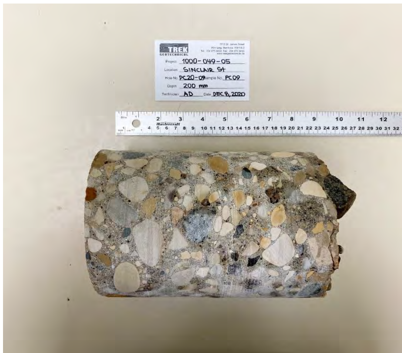
Photo 2: Pavement Core Sample at PC20-09
