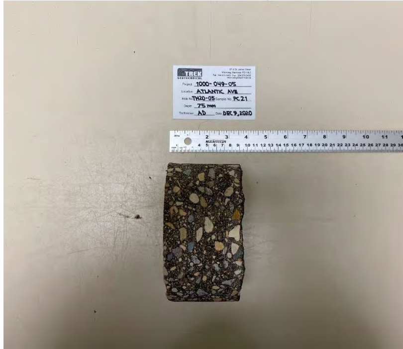
Photo 5: Pavement Core Sample at Test Hole TH20-05
