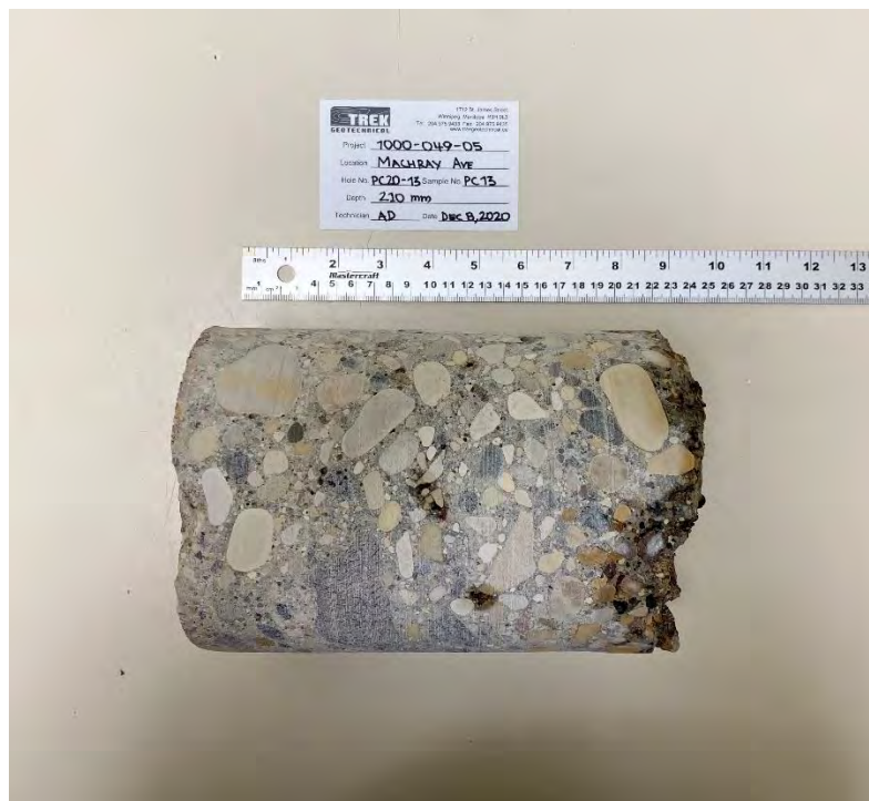
Photo 6: Pavement Core Sample at PC20-13
