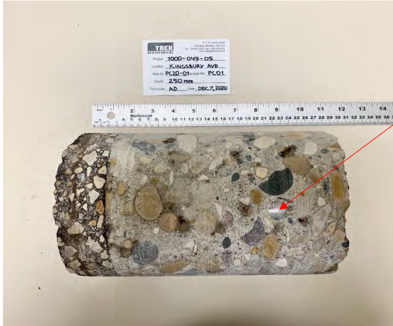
Photo 1: Pavement Core Sample at PC20-01
