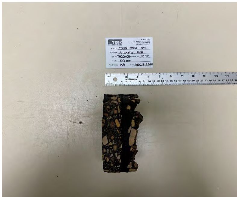
Photo 4: Pavement Core Sample at Test Hole TH20-04
