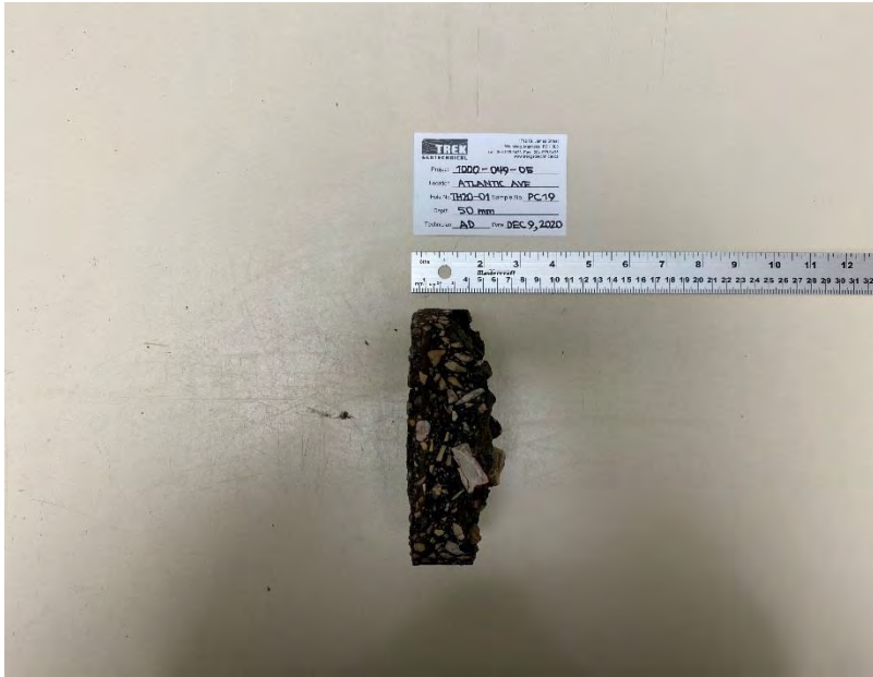
Photo 1: Pavement Core Sample at Test Hole TH20-01
