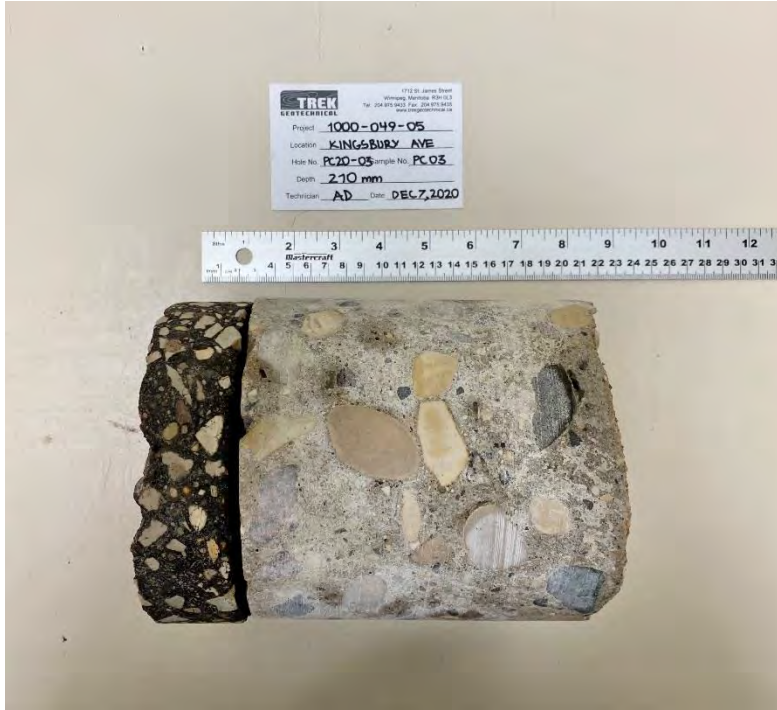
Photo 3: Pavement Core Sample at PC20-03
