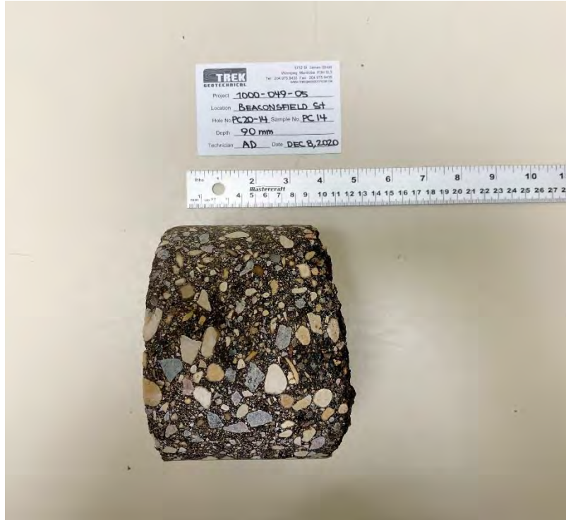
Photo 1: Pavement Core Sample at PC20-14
