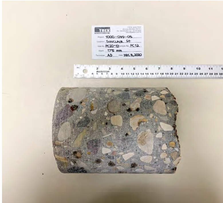
Photo 5: Pavement Core Sample at PC20-12
