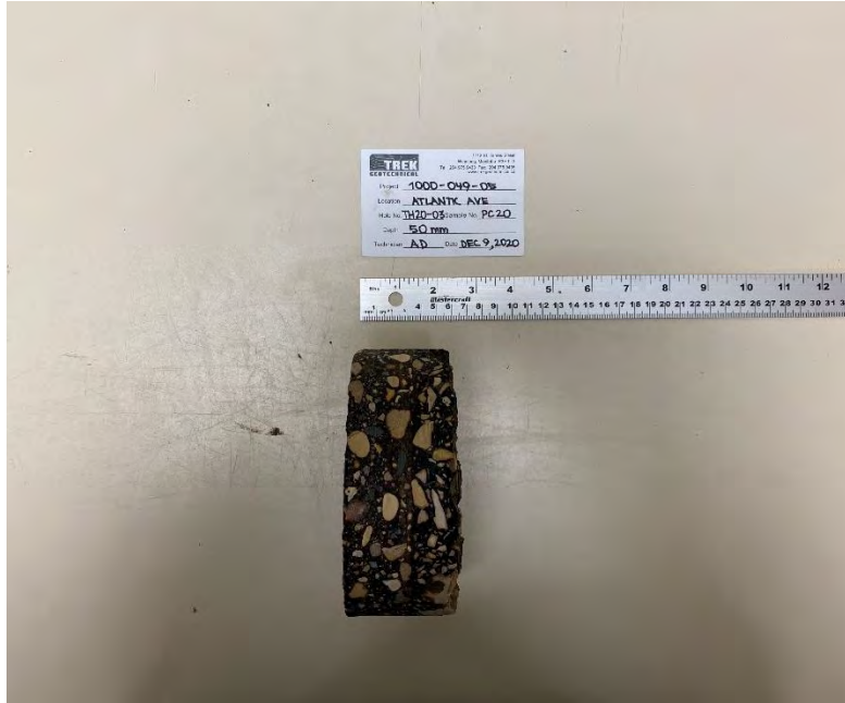
Photo 3: Pavement Core Sample at Test Hole TH20-03
