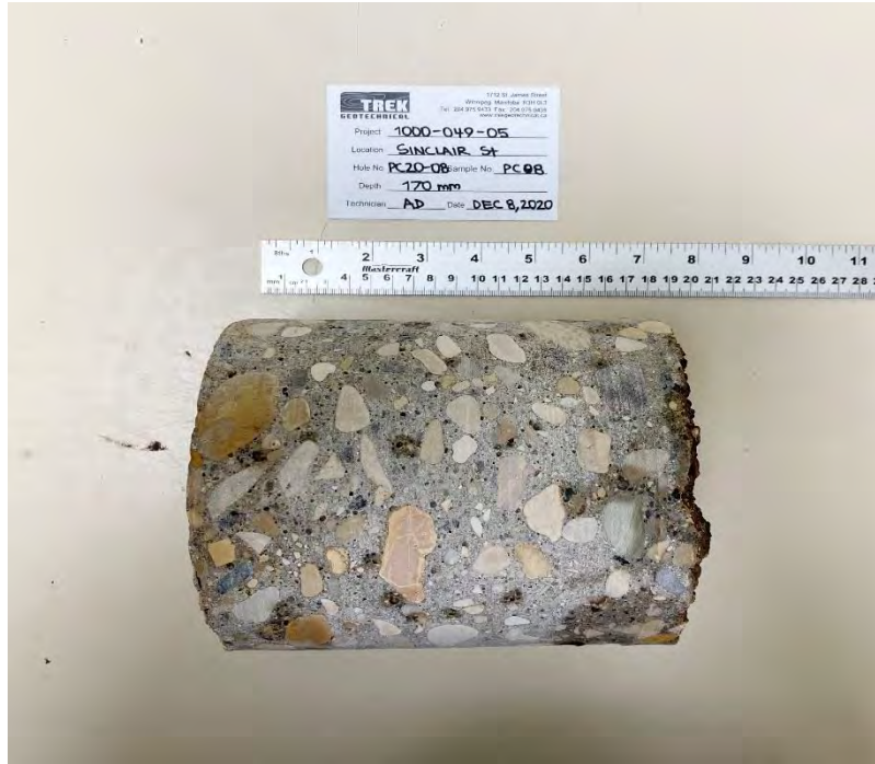
Photo 1: Pavement Core Sample at PC20-08
