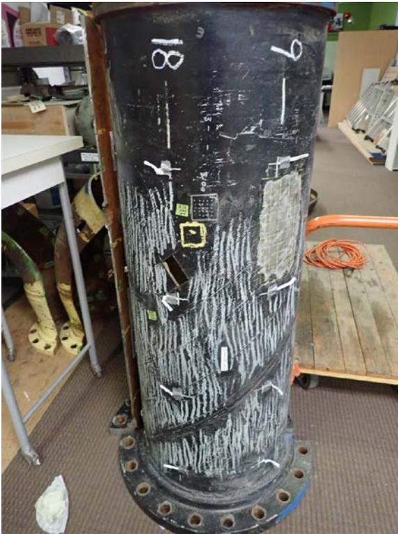
Photo 5. Paint Sample S-04 location (black piping system; RAS 2 HPO Reactor Inlet) from off-site pipe located at Testlabs International.
