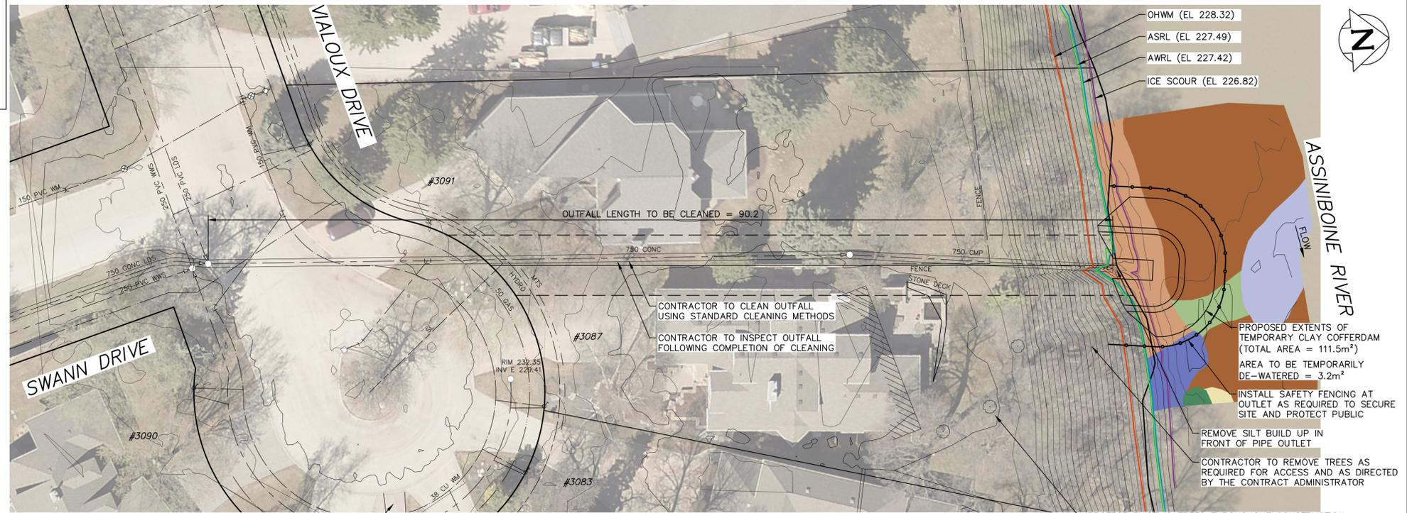
AS REQUIRED TO FACILITATE CLEANING, THE CONTRACTOR SHALL DEVELOP ACCESS THROUGH EXISTING PARK SPACE TO ACCESS OUTLET (SEE NOTES 5 & 6)
