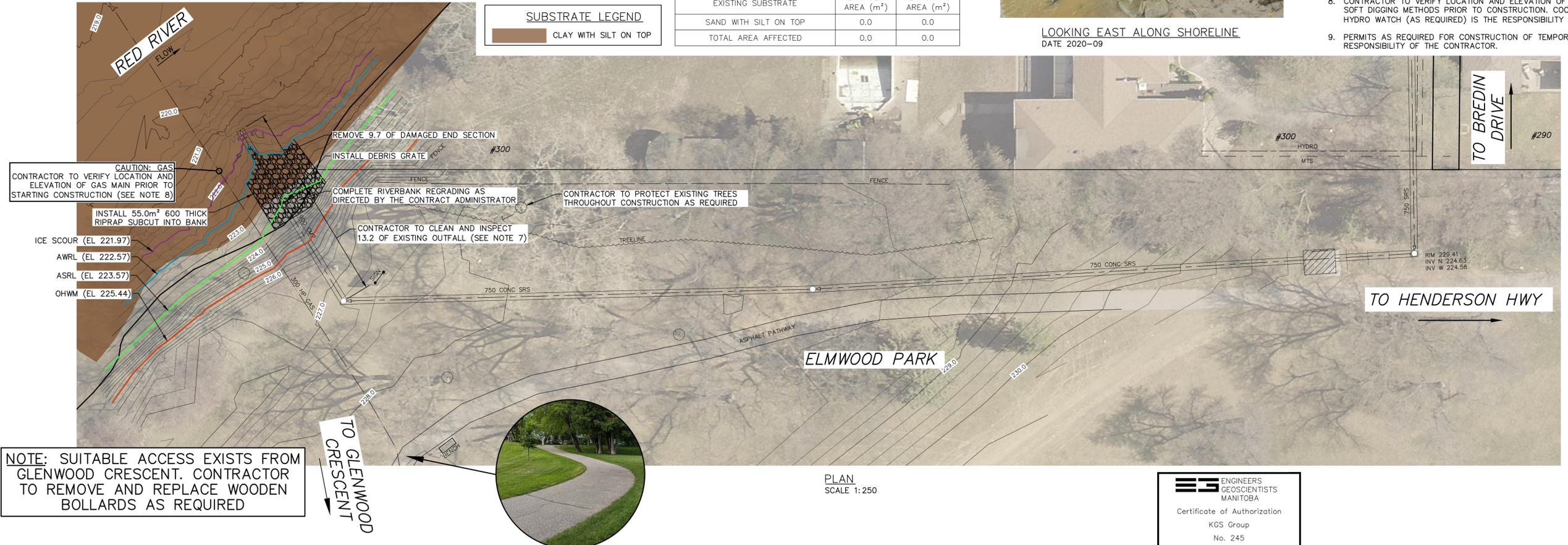
NOTE: SUITABLE ACCESS EXISTS FROM GLENWOOD CRESCENT. CONTRACTOR TO REMOVE AND REPLACE WOODEN BOLLARDS AS REQUIRED
