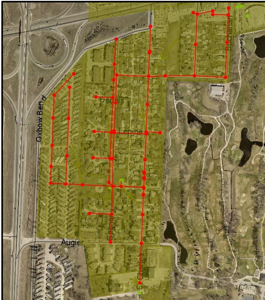
Figure 1: St. Charles Separated Sewer District
