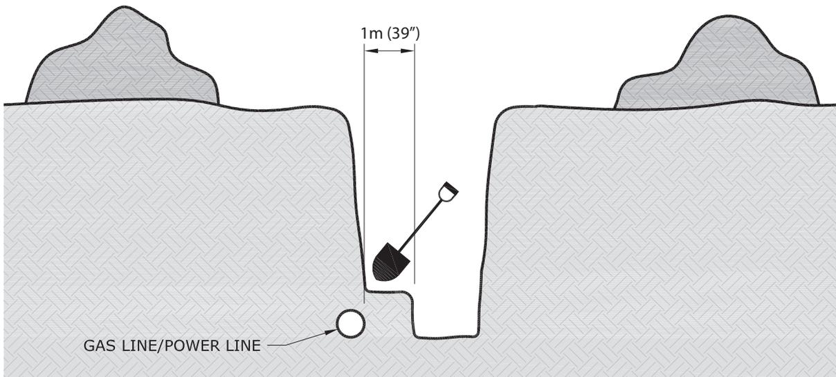
Dig a trench or bell hole 1 metre from the line location, parallel to the line, then hand dig laterally to expose the line.
