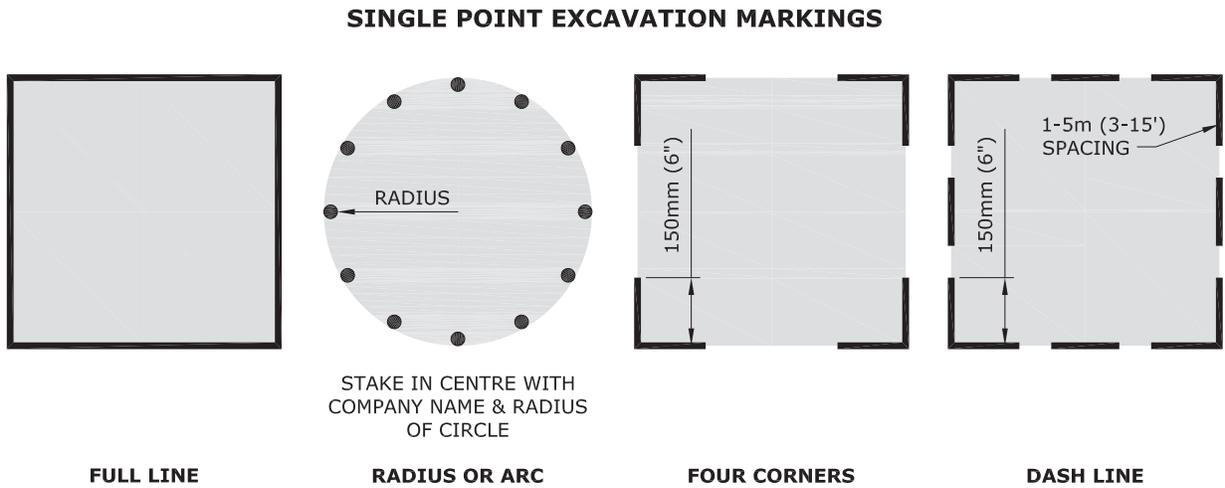
If an excavation is contained within a 5 metre maximum radius then it can be marked with a single white stake at the centre of the excavation. The stake must clearly state the company identifier and the radius of the excavation in black lettering. This information must be conveyed to Manitoba Hydro.
