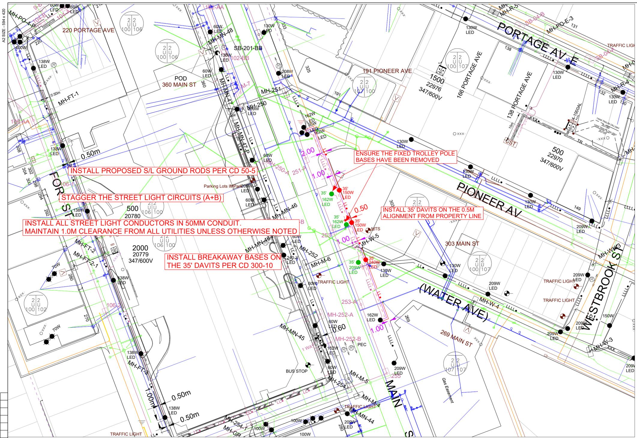
**INSTALL PROPOSED S/L GROUND RODS PER CD 50-5**
