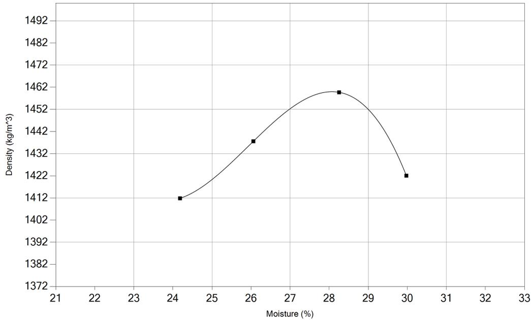
**Moisture Density Relationship: (ASTM D698-12) Method: A**
