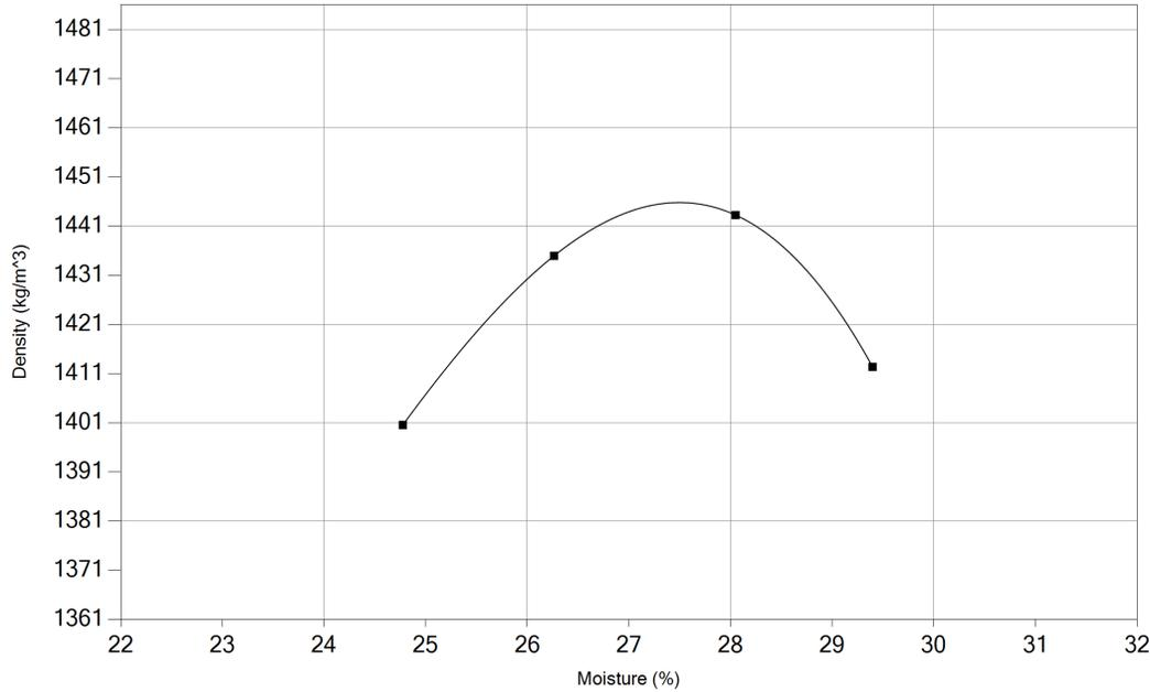
**Moisture Density Relationship: (ASTM D698-12) Method: A**
