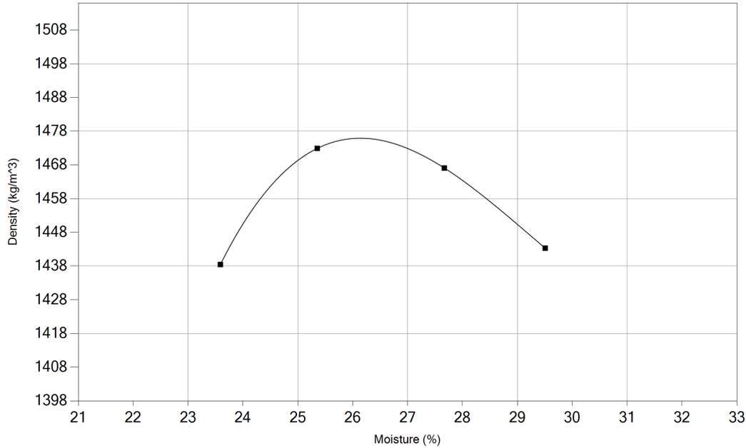
**Moisture Density Relationship: (ASTM D698-12) Method: A**
