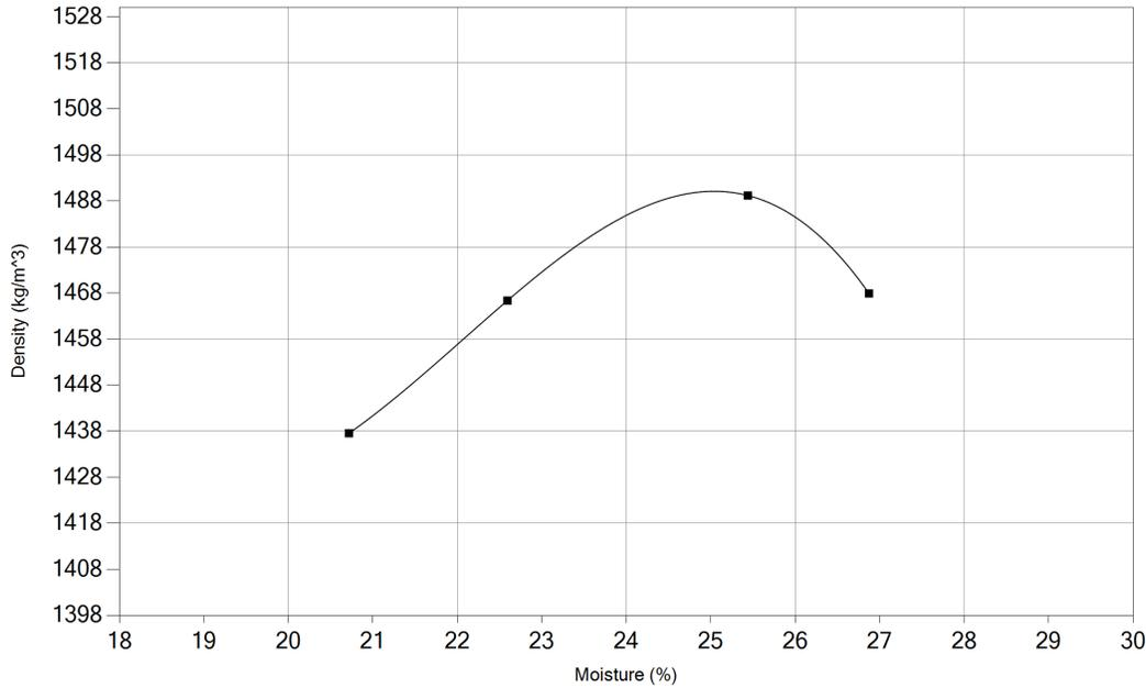
**Moisture Density Relationship: (ASTM D698-12) Method: A**
