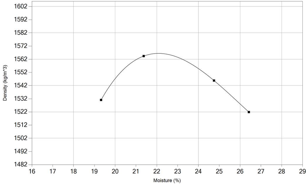
**Moisture Density Relationship: (ASTM D698-12) Method: A**
