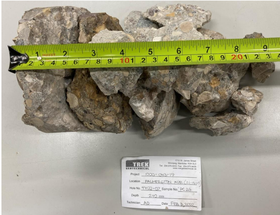
Photo 1: Pavement Core Sample at Test Hole TH22-07
