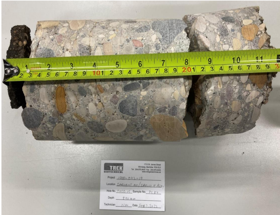
Photo 3: Pavement Core Sample at Test Hole TH22-15
