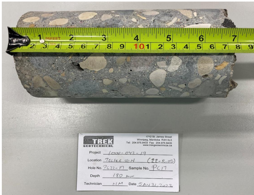
Photo 6: Pavement Core Sample at PC22-17
