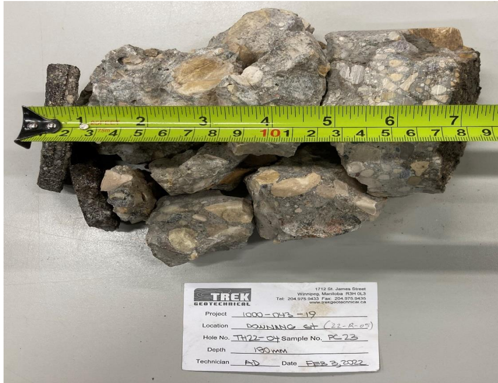
Photo 1: Pavement Core Sample at Test Hole TH22-04
