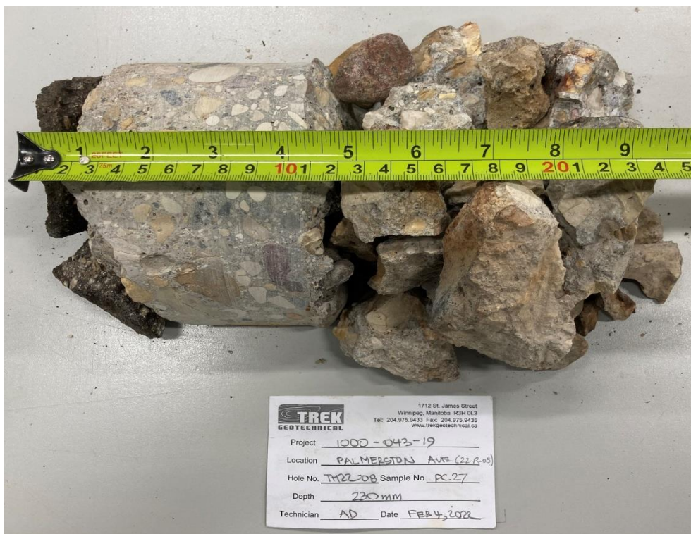
Photo 2: Pavement Core Sample at Test Hole TH22-08
