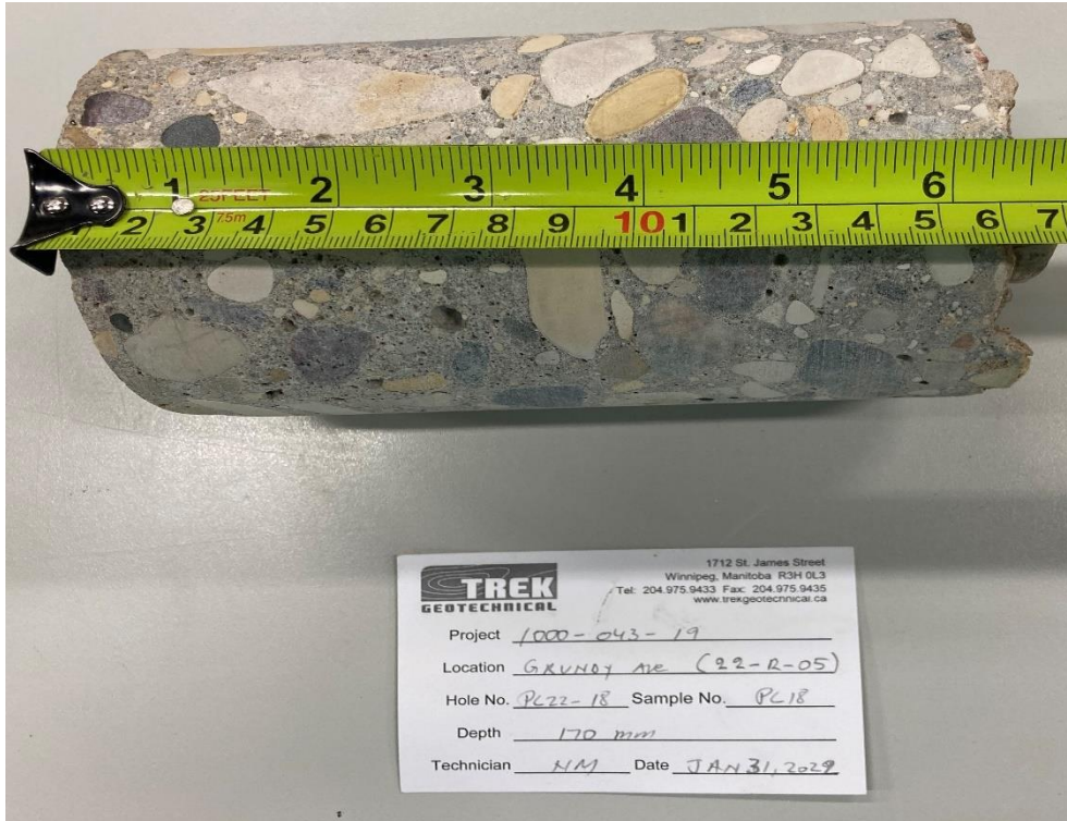
Photo 1: Pavement Core Sample at PC22-18
