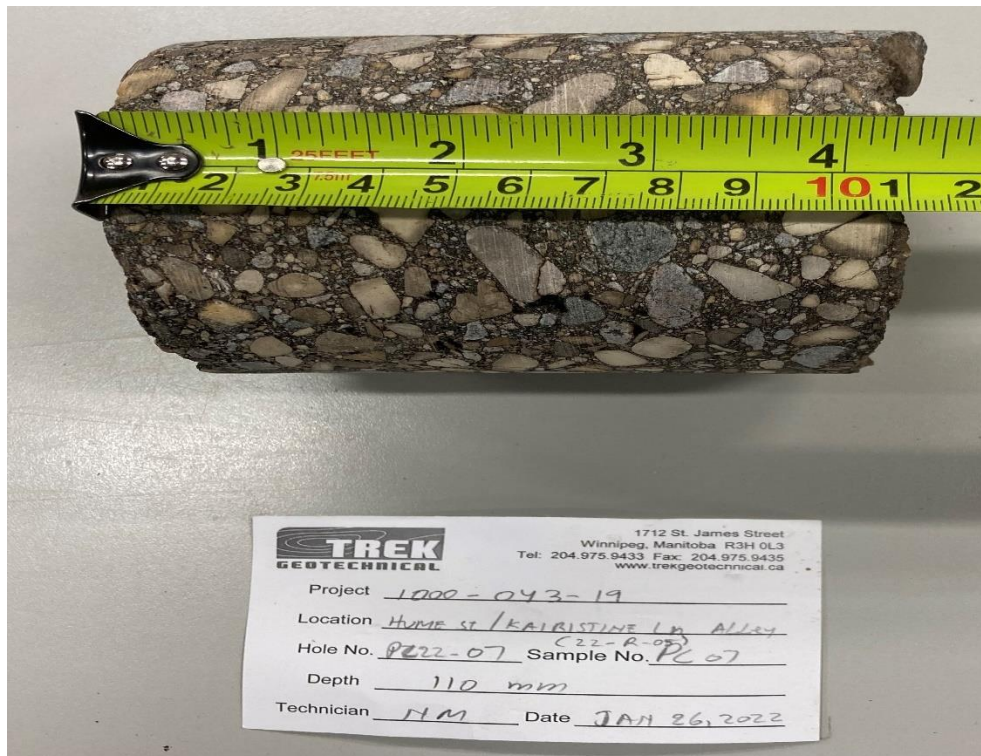
Photo 2: Pavement Core Sample at PC22-07
