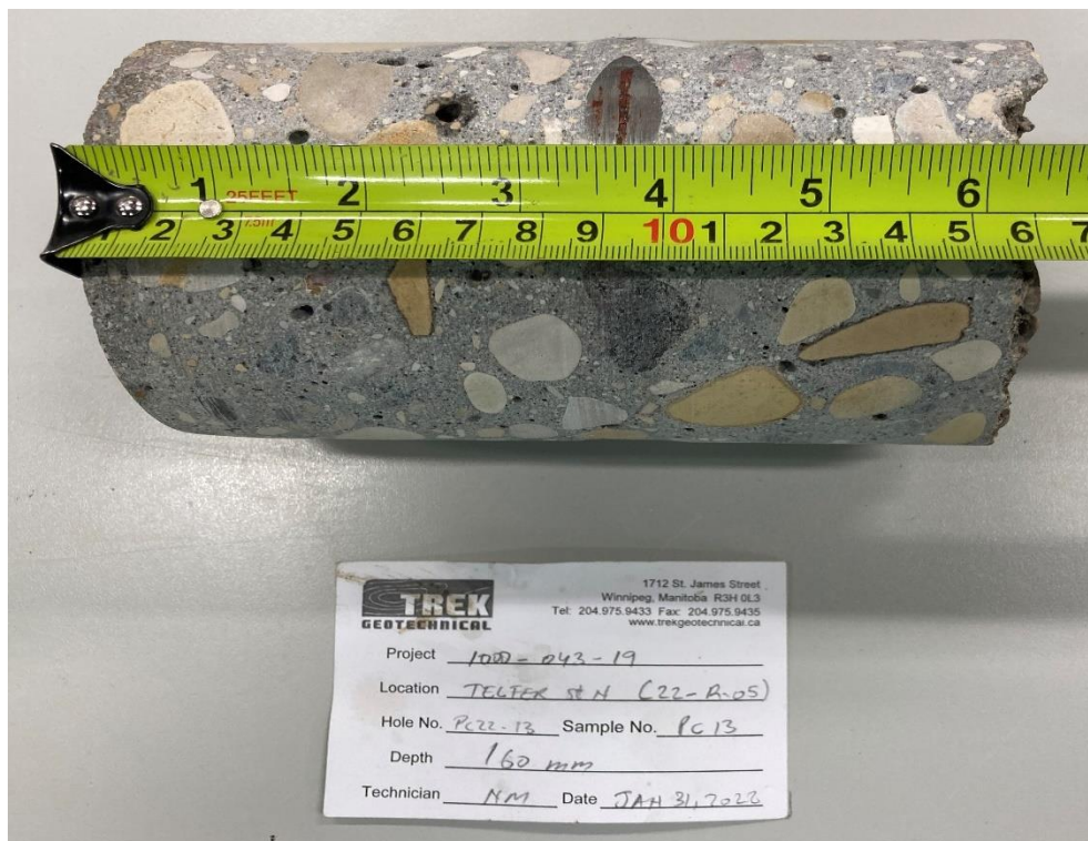
Photo 2: Pavement Core Sample at PC22-13
