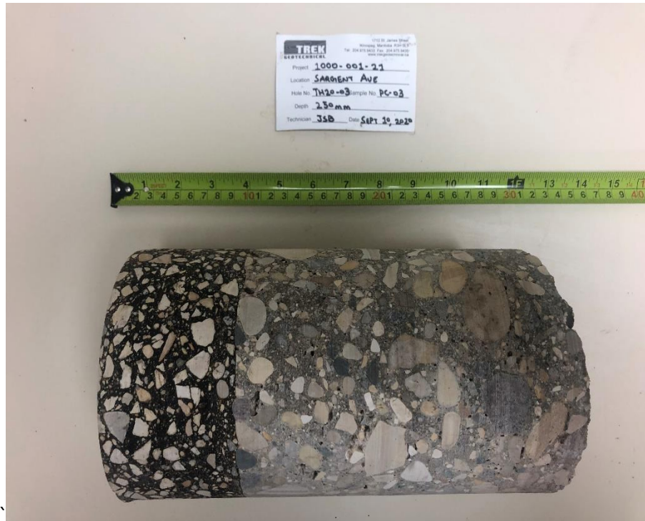
Photo 3: Pavement Core Sample at Test Hole TH20-03
