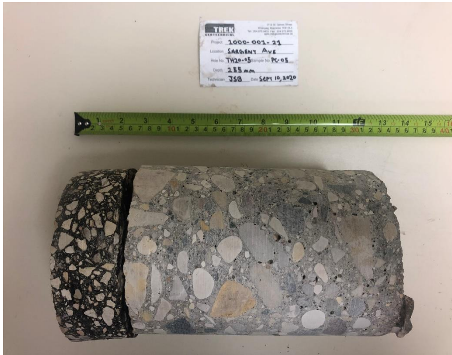
Photo 5: Pavement Core Sample at Test Hole TH20-05
