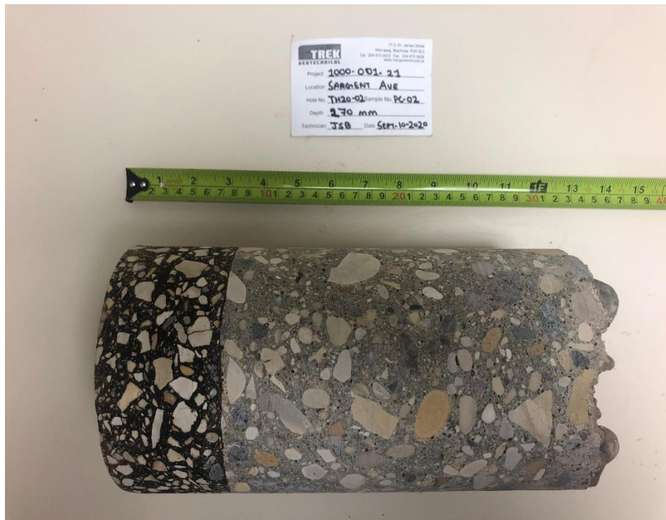
Photo 2: Pavement Core Sample at Test Hole TH20-02
