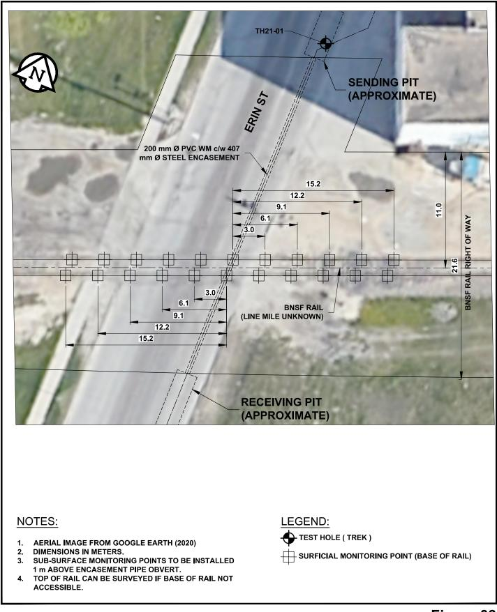
0 2.5 5 7.5 10 12.5 m SCALE = 1 : 250 (219 mm x 279 mm) Figure 03 Monitoring Point Detail Plan on BNSF RAIL Track
