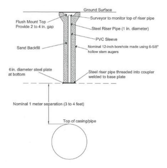
Figure B - Typical Subsurface Settlement Point Detail
