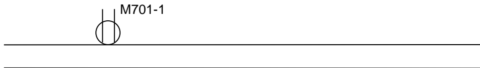
Figure 6-1 : Receptacle Identification on Plan Drawings
