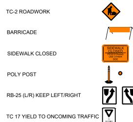
6. TC-2 ROADWORK SIGNAGE TO BE PLACED 50.0m IN ADVANCE OF CONSTRUCTION.
