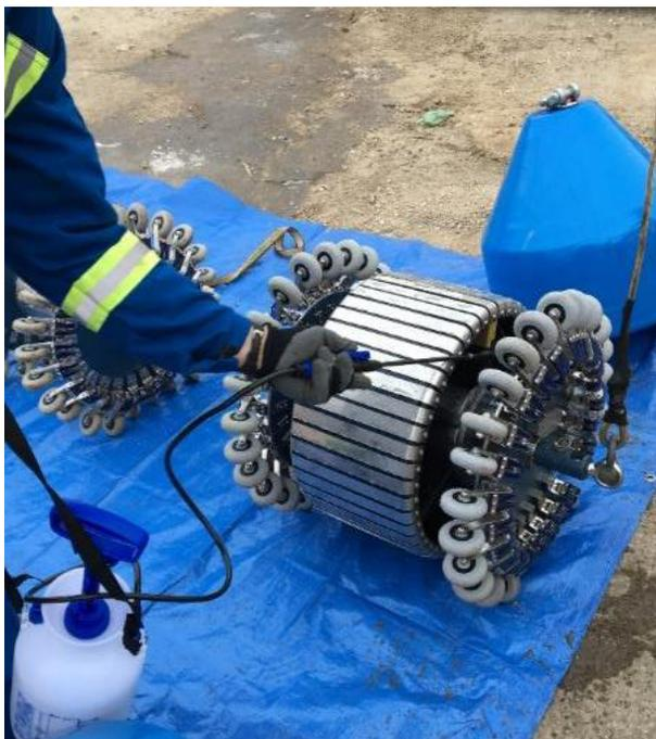
Figure 5. Disinfecting the Chimera assembly using a 200 mg/L free chlorine solution
