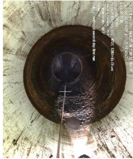
Figure 13. Looking into pipe from the East Chamber towards first downward deflection.
