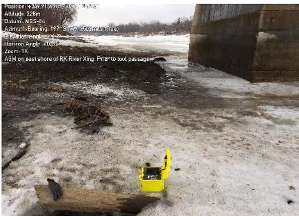
Figure 14. AGM unit on the east side of the Red River, recording tool passage
