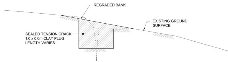
**TYPICAL TENSION CRACK SEALING DETAIL**
