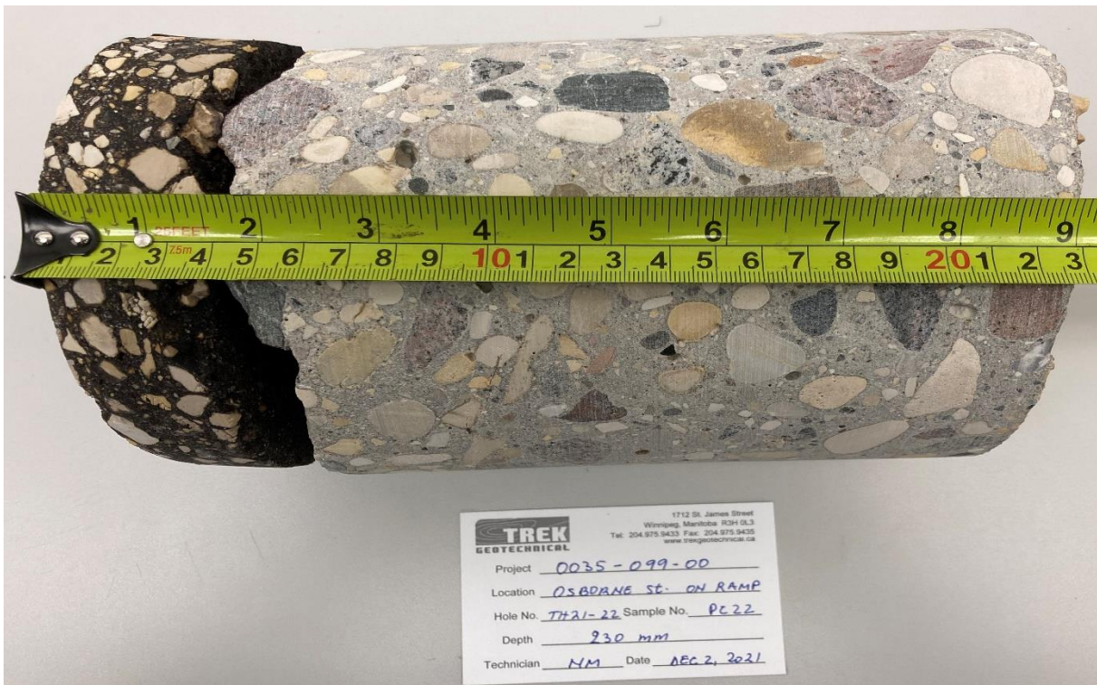
Photo 22: Pavement Core Sample at Test Hole TH21-22
