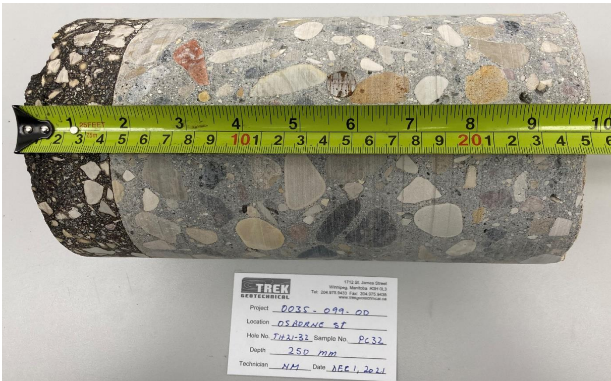
Photo 32: Pavement Core Sample at Test Hole TH21-32
