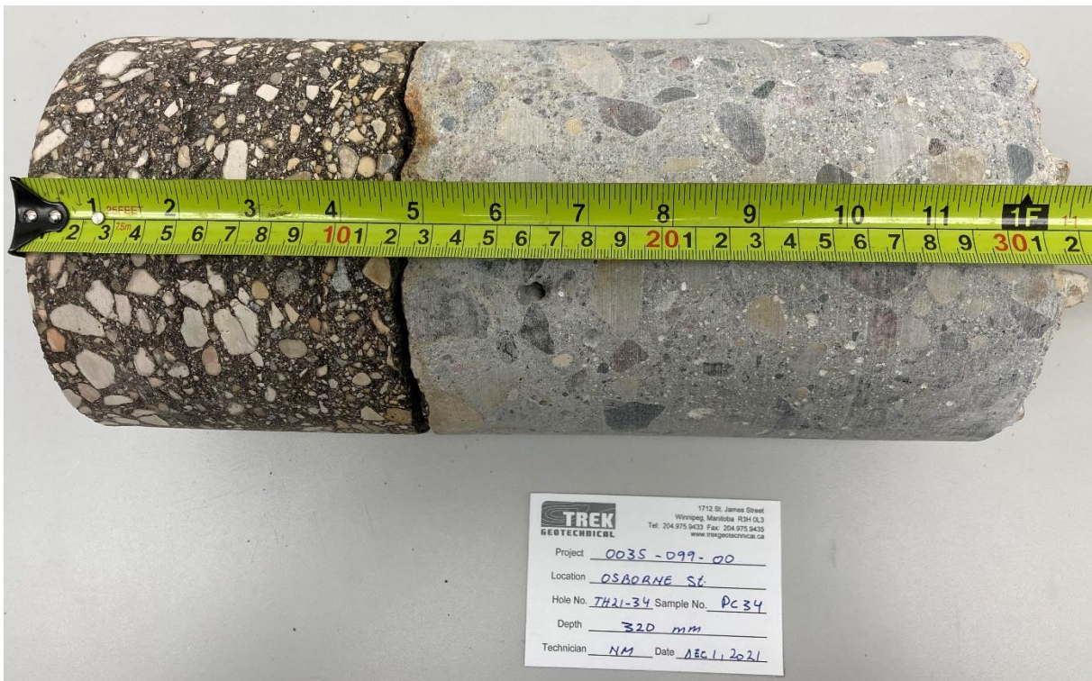
Photo 34: Pavement Core Sample at Test Hole TH21-34
