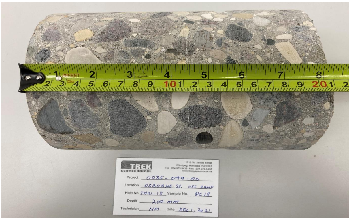
Photo 18: Pavement Core Sample at Test Hole TH21-18
