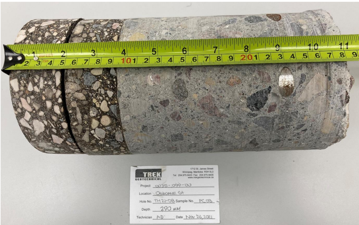
Photo 8: Pavement Core Sample at Test Hole TH21-08
