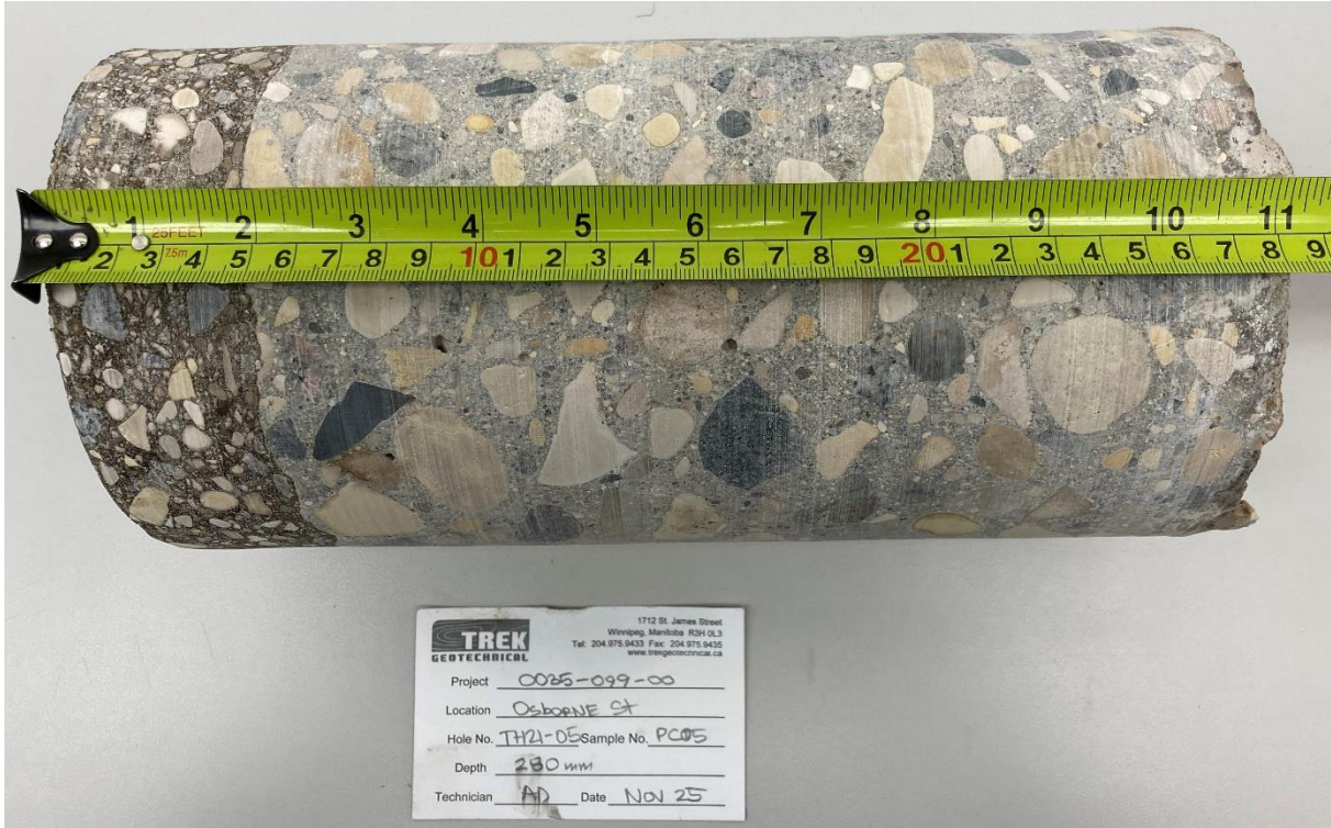
Photo 5: Pavement Core Sample at Test Hole TH21-05
