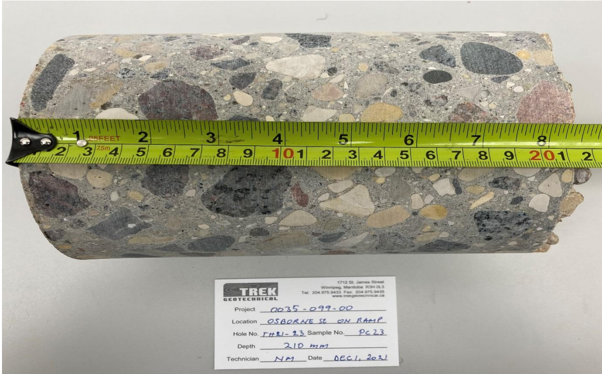
Photo 23: Pavement Core Sample at Test Hole TH21-23
