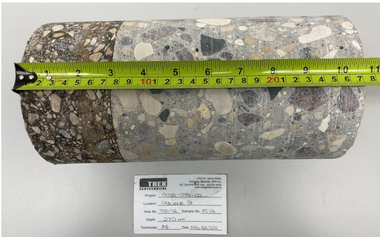
Photo 12: Pavement Core Sample at Test Hole TH21-12
