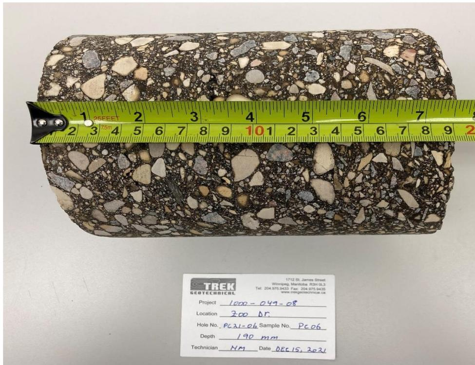
Photo 2: Pavement Core Sample at PC21-06
