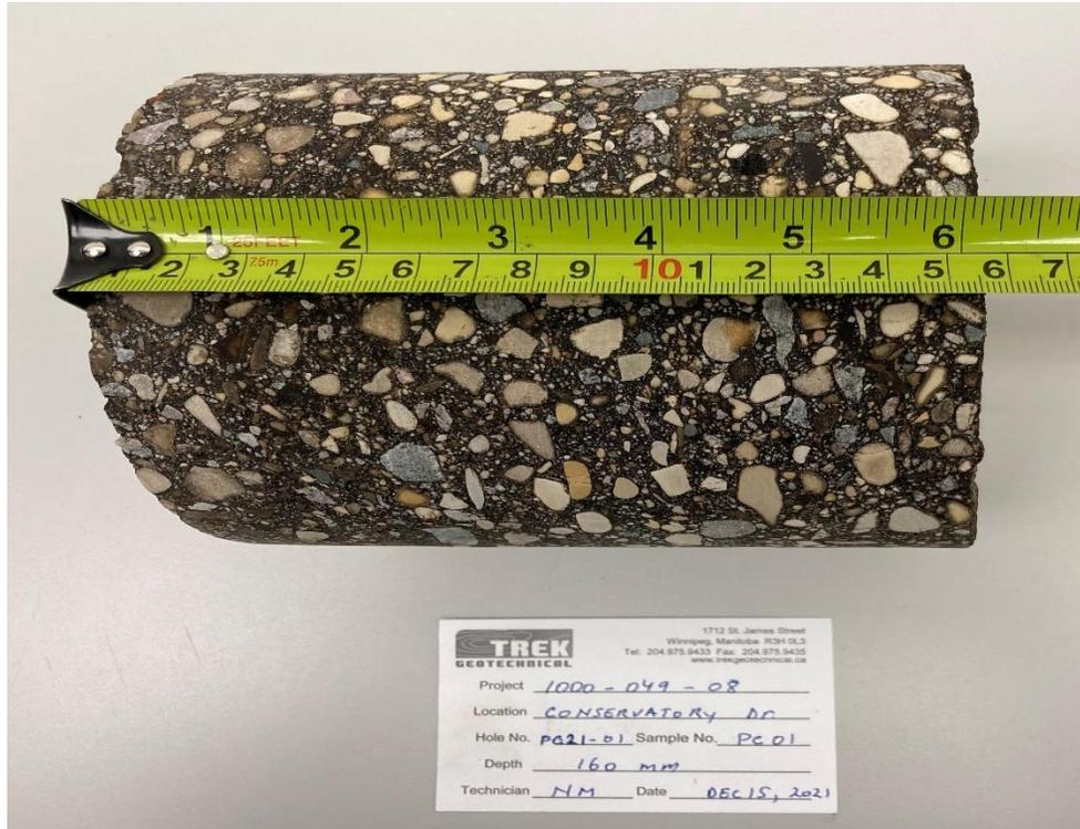
Photo 1: Pavement Core Sample at PC21-01
