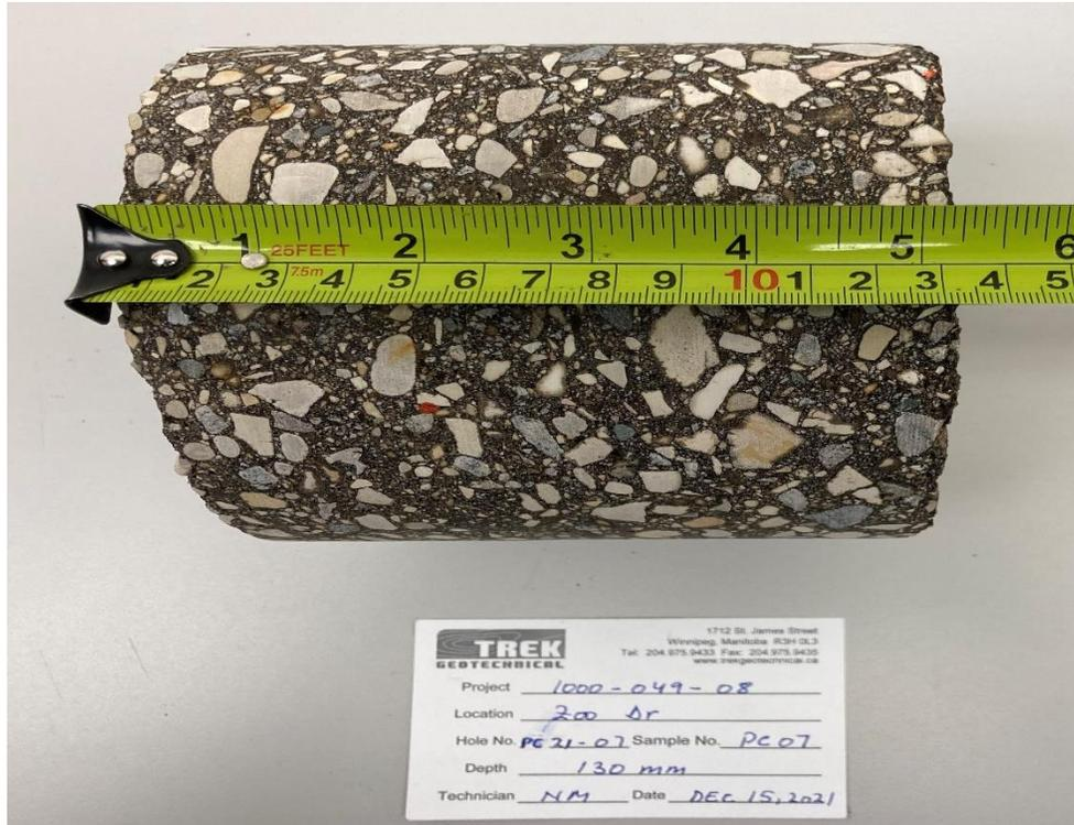
Photo 3: Pavement Core Sample at PC21-07
