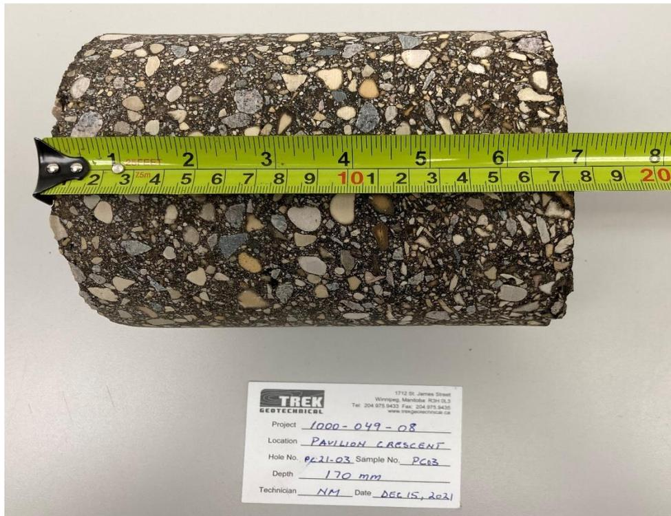
Photo 2: Pavement Core Sample at PC21-03
