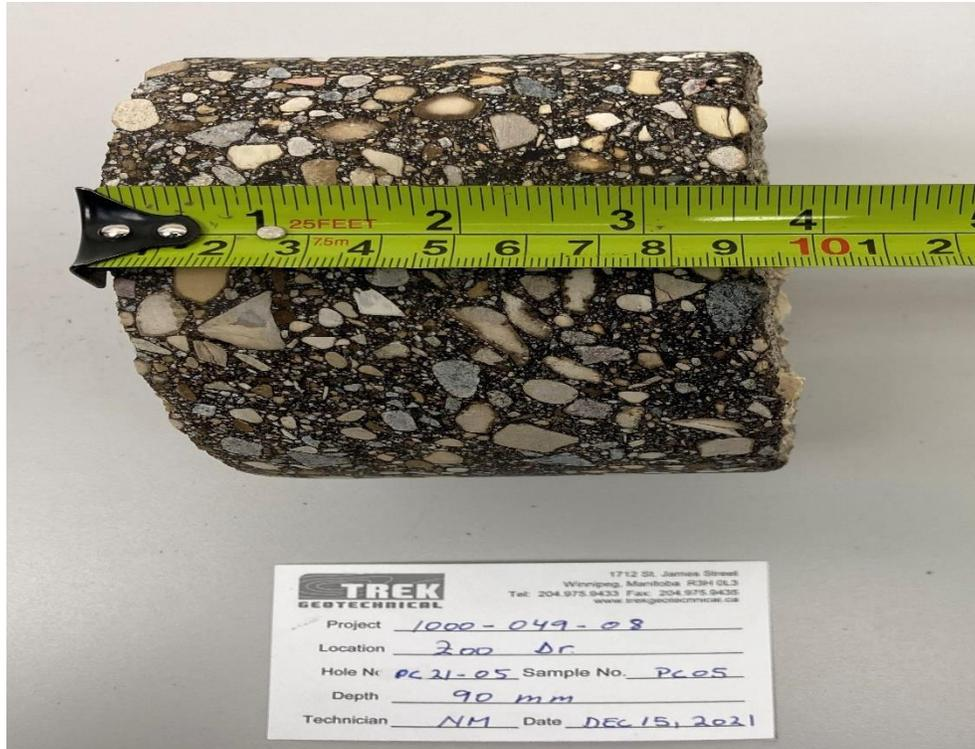
Photo 1: Pavement Core Sample at PC21-05
