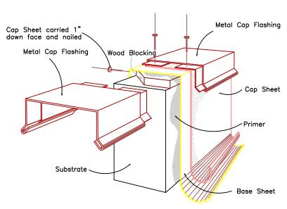
26 Gauge counter flashing complete with approx. 1/2" 45 degreee bottom kick out is to be installed over all membrane stripping. Terminate flashing about 1" above top of new roofing. Do not install any fasteners behind the cap flashing and use only lap joints. This is to allow easy removal for future repairs.
