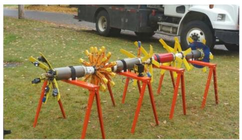
Figure A 3 - PipeDiver EM Inspection Platform (courtesy of Pure).
