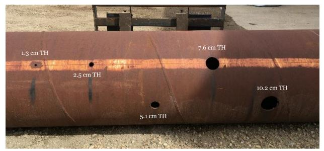
Figure 27. Through holes machined into the 24in calibration pipe. Defects measured 1.3 cm, 2.5 cm, 5.1 cm, 7.6 cm, and 10.2 cm (0.5in, 1.0in, 2.0in, 3.0in, and 4.0in) in diameter.
