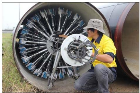
Figure A 6 - Recently Developed 1200mm Pipe Inspection Tool (courtesy of Pure).
