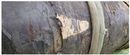
Figure 48: Localized Coating Damage on the Charleswood-Assiniboia Feeder Main
