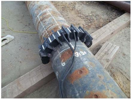
Figure A 7 - Bracelet Probe Pipe Wall Inspection System (courtesy of PICA).
