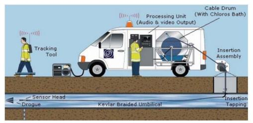
Figure A 11 - Sahara Inspection System (courtesy of Pure).
