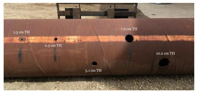
Figure 37. Through holes machined into the 24in calibration pipe. Defects measured 1.3 cm, 2.5 cm, 5.1 cm, 7.6 cm, and 10.2 cm (0.5in, 1.0in, 2.0in, 3.0in, and 4.0in) in diameter.
