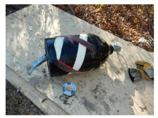
Figure 3 - Modified Cleaning Pig with Steel Cable Pull Ropes
