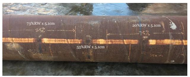
Figure 35. Calibration pipe with 73% RW, 53% RW, and 20% RW 5.1cm diameter flat bottom defects.
