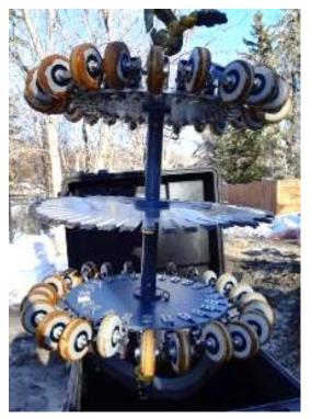
Figure 5. PICA's custom gauge tool assembly shown after being pulled through the Charleswood-Assiniboia Feeder Main
