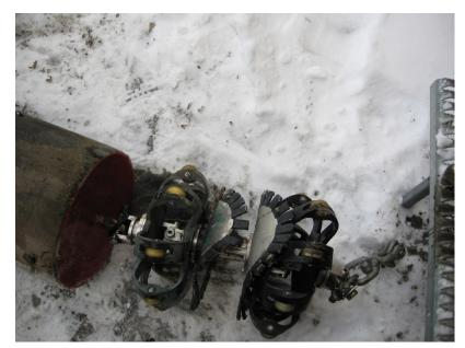
Figure 29: Gauge Pig with Foam Swab
