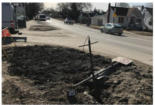
Photo 7 - Acoustic correlator set up on 300 mm gate valve during second setup on April 18
