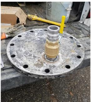
Figure 1: Blind flange with ball valve used for the leakage test.
