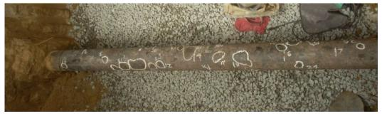
Figure 49: Example of Localized Pit Locations on a Steel Pipeline
