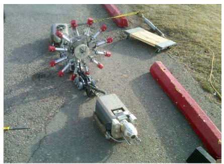
Figure A 4 - PureRobotics Crawler Inspection Platform (courtesy of Pure).
