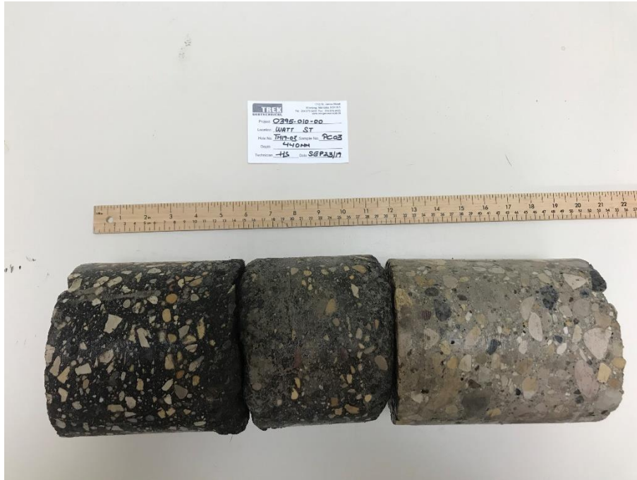
Photo 3: Pavement Core Sample at Test Hole TH19-03
