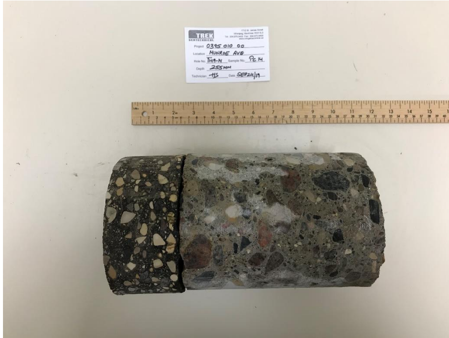
Photo 14: Pavement Core Sample at Test Hole TH19-14
