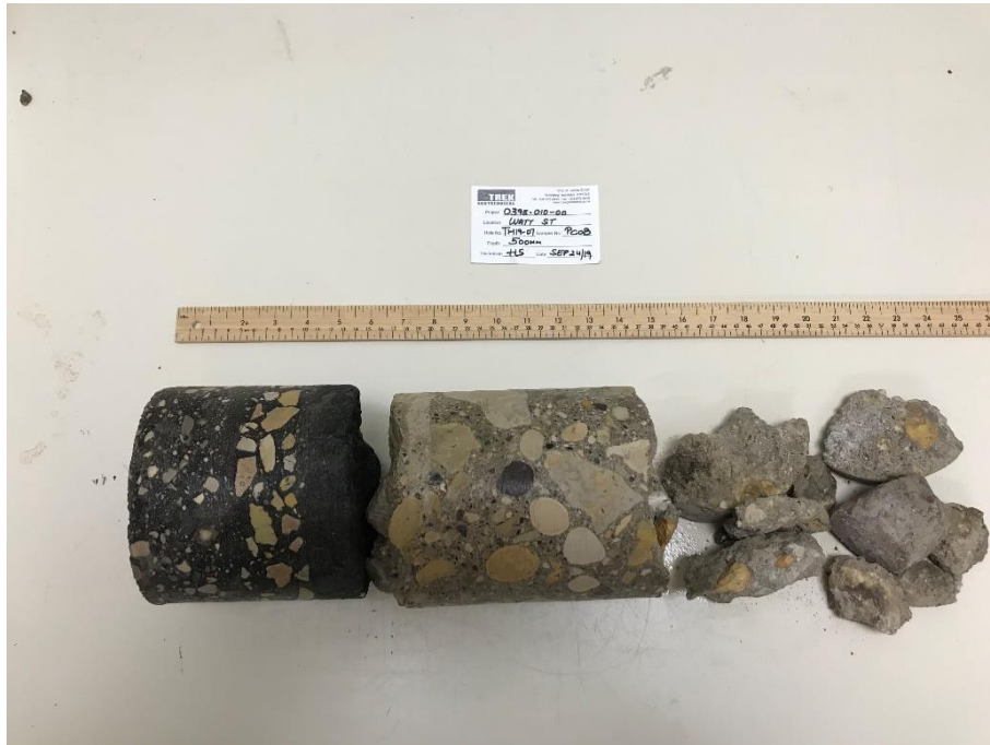
Photo 7: Pavement Core Sample at Test Hole TH19-07
