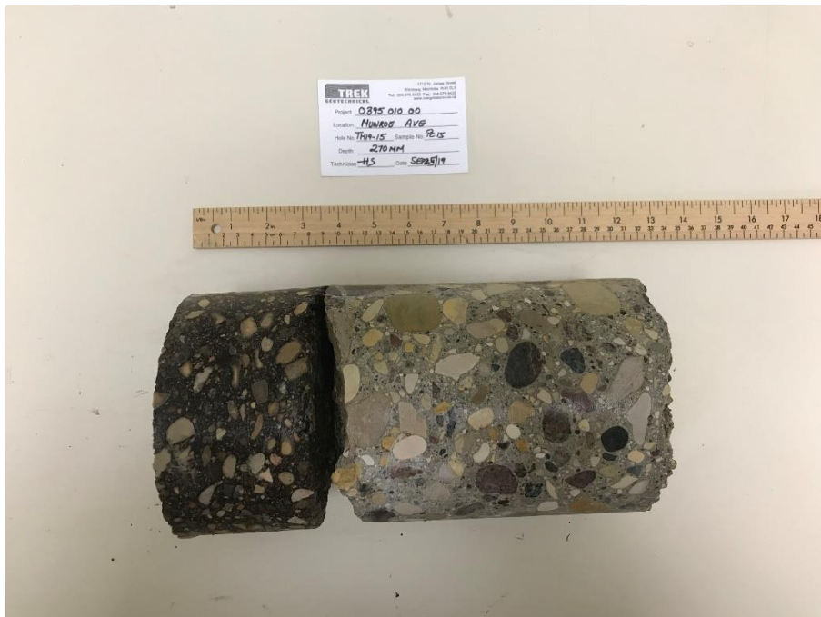
Photo 15: Pavement Core Sample at Test Hole TH19-15
