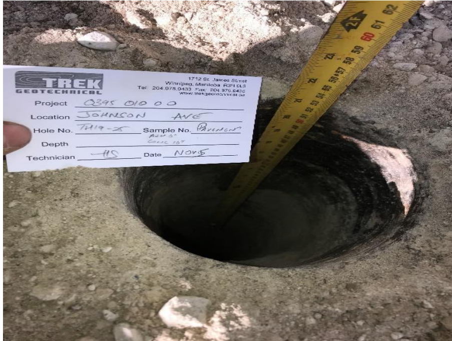
Photo 25: Pavement Core Measurement at Test Hole TH19-25
