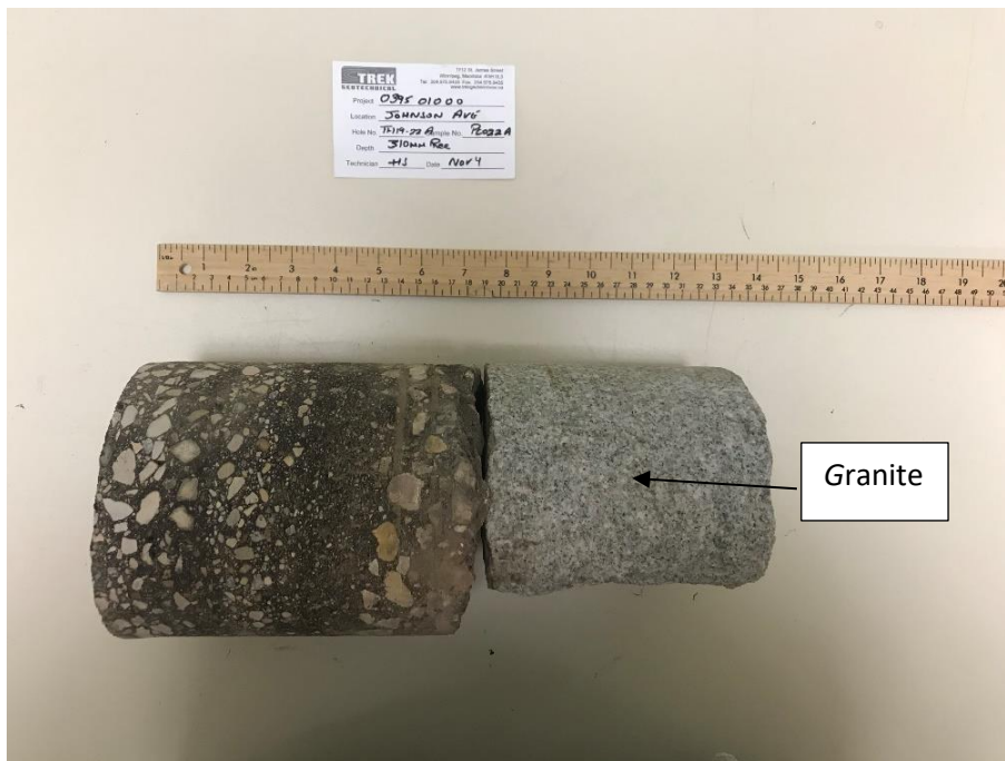
Photo 22: Recovered Pavement Core Sample at Test Hole TH19-22A (1.5 m West of TH19-22)
