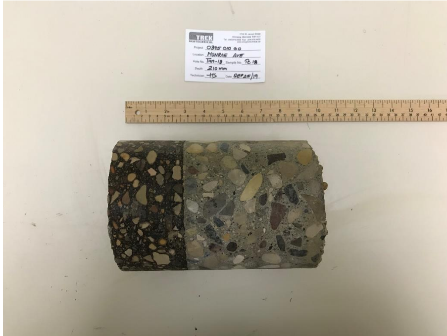
Photo 18: Pavement Core Sample at Test Hole TH19-18
