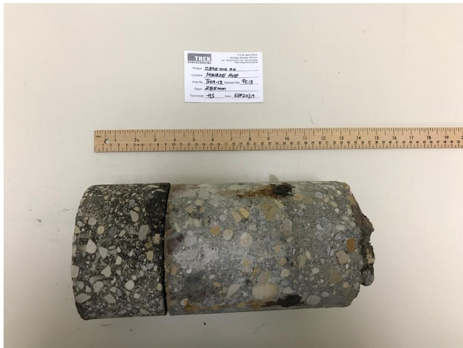
Photo 13: Pavement Core Sample at Test Hole TH19-13
