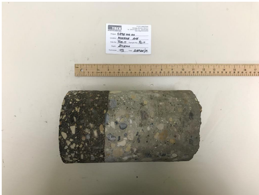
Photo 17: Pavement Core Sample at Test Hole TH19-17
