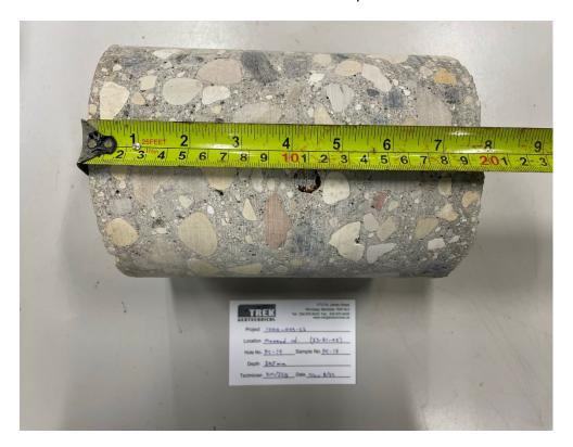
Photo 2: Pavement Core Sample PC-14
