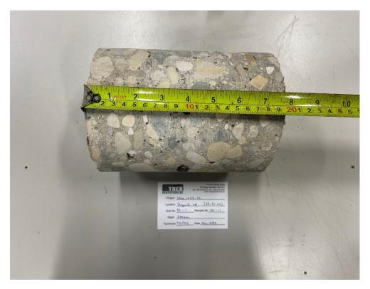
Photo 1: Pavement Core Sample PC-11
