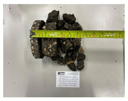
Photo 3: Pavement Core Sample at TH22-08
