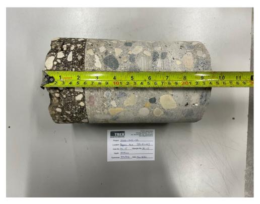
Photo 1: Pavement Core Sample PC-15
