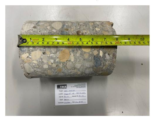
Photo 2: Pavement Core Sample PC-10
