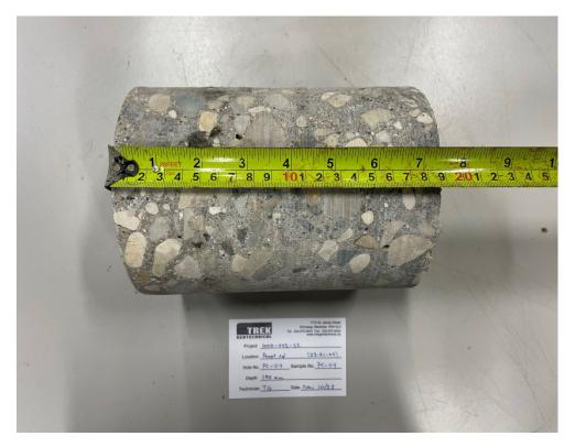
Photo 1: Pavement Core Sample PC-04
