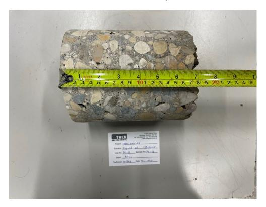
Photo 2: Pavement Core Sample PC-12
