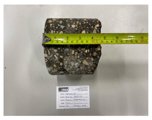
Photo 3: Pavement Core Sample at TH22-03
