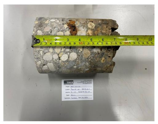
Photo 1: Pavement Core Sample PC-09
