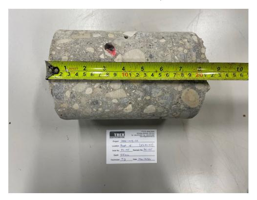
Photo 2: Pavement Core Sample PC-05
