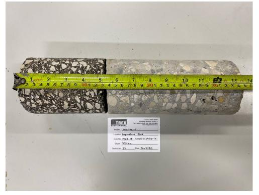
Photo 13: Pavement Core Sample PC-13
