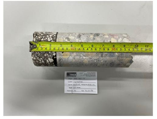
Photo 3: Pavement Core Sample PC-03
