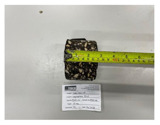
Photo 6: Pavement Core Sample PC-06
