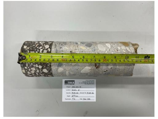
Photo 1: Pavement Core Sample PC-20
