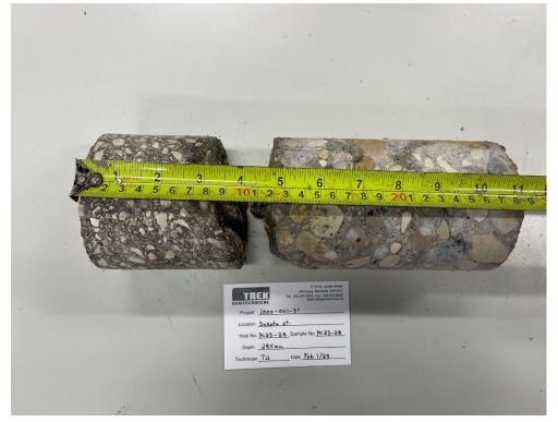
Photo 9: Pavement Core Sample PC-28
