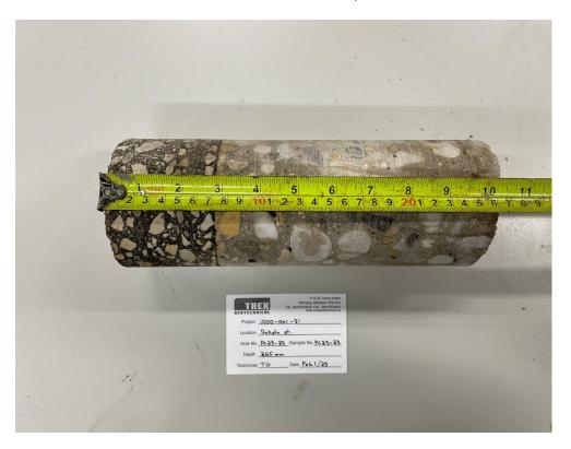
Photo 4: Pavement Core Sample PC-23
