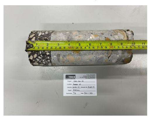
Photo 12: Pavement Core Sample PC-31
