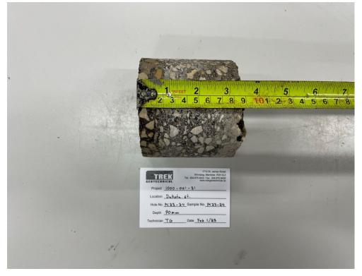
Photo 5: Pavement Core Sample PC-24
