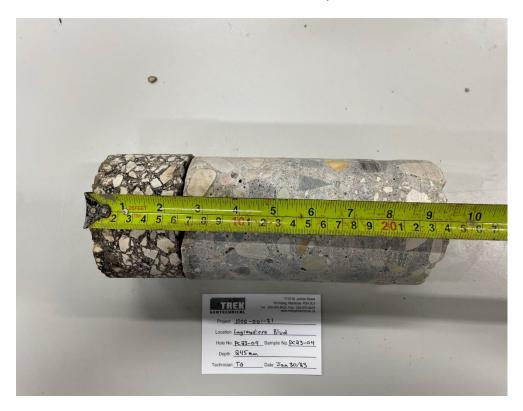
Photo 4: Pavement Core Sample PC-04
