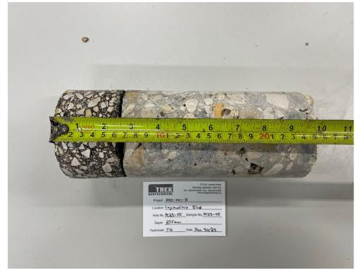
Photo 5: Pavement Core Sample PC-05
