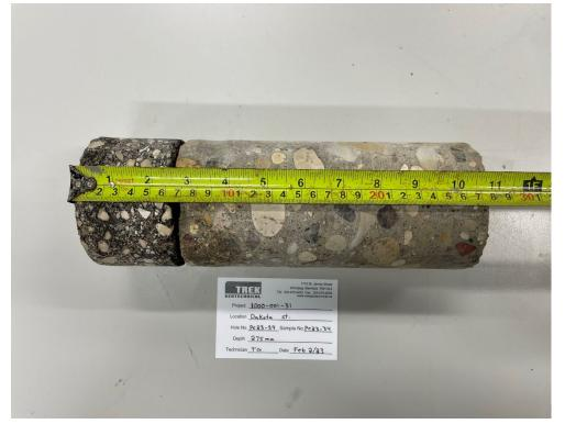
Photo 15: Pavement Core Sample PC-34
