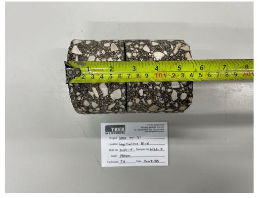
Photo 15: Pavement Core Sample PC-15
