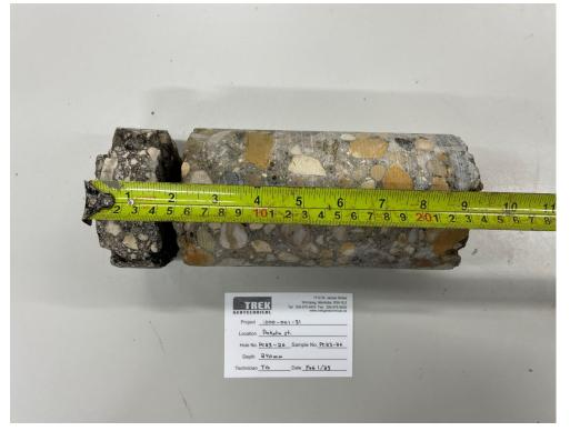
Photo 7: Pavement Core Sample PC-26
