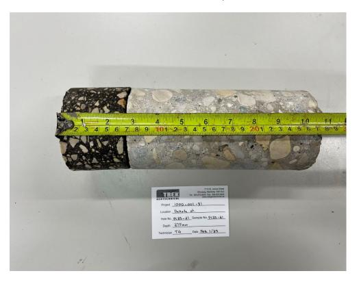
Photo 2: Pavement Core Sample PC-21
