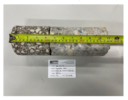
Photo 8: Pavement Core Sample PC-08
