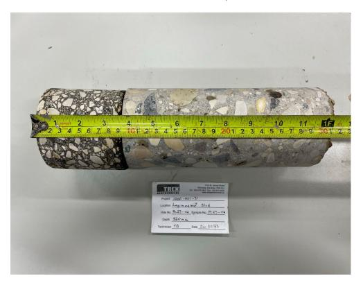
Photo 2: Pavement Core Sample PC-02
