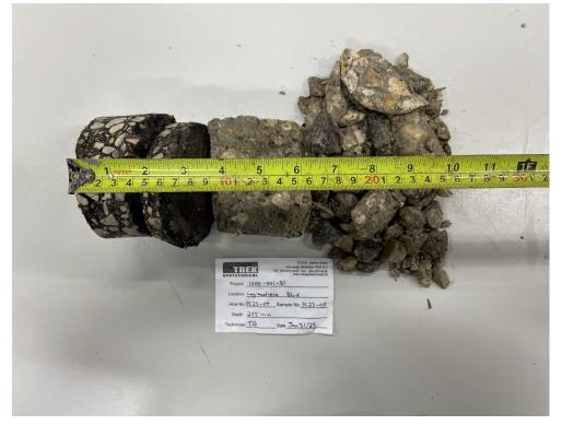
Photo 9: Pavement Core Sample PC-09
