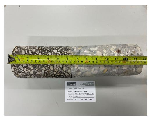
Photo 14: Pavement Core Sample PC-14
