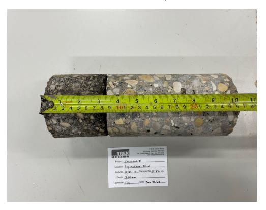
Photo 10: Pavement Core Sample PC-10
