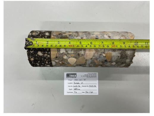
Photo 11: Pavement Core Sample PC-30
