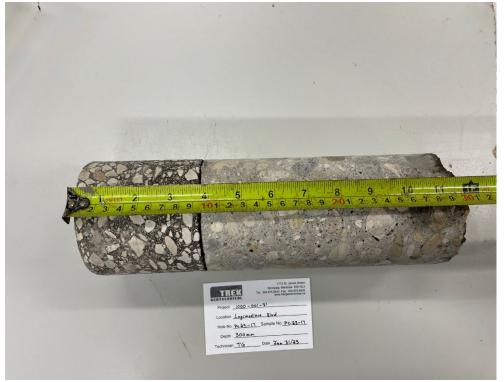
Photo 17: Pavement Core Sample PC-17
