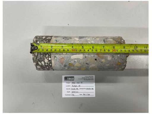
Photo 13: Pavement Core Sample PC-32
