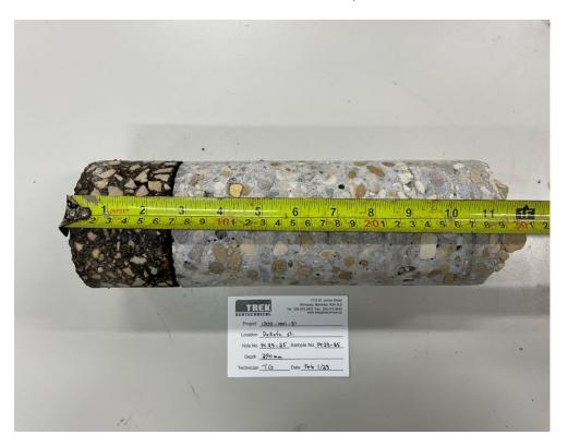
Photo 6: Pavement Core Sample PC-25
