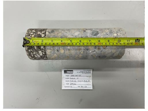
Photo 3: Pavement Core Sample PC-22
