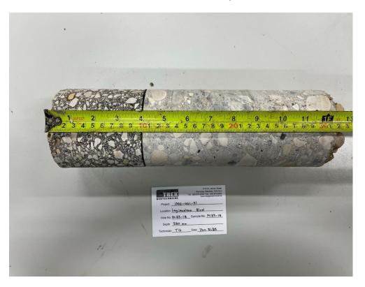
Photo 18: Pavement Core Sample PC-18
