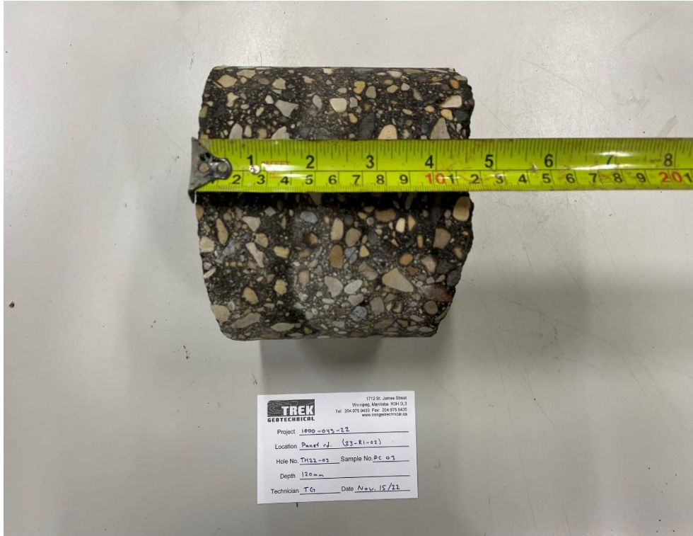
Photo 3: Pavement Core Sample at TH22-03
