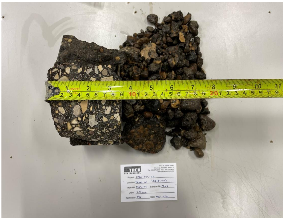
Photo 2: Pavement Core Sample at TH22-02
