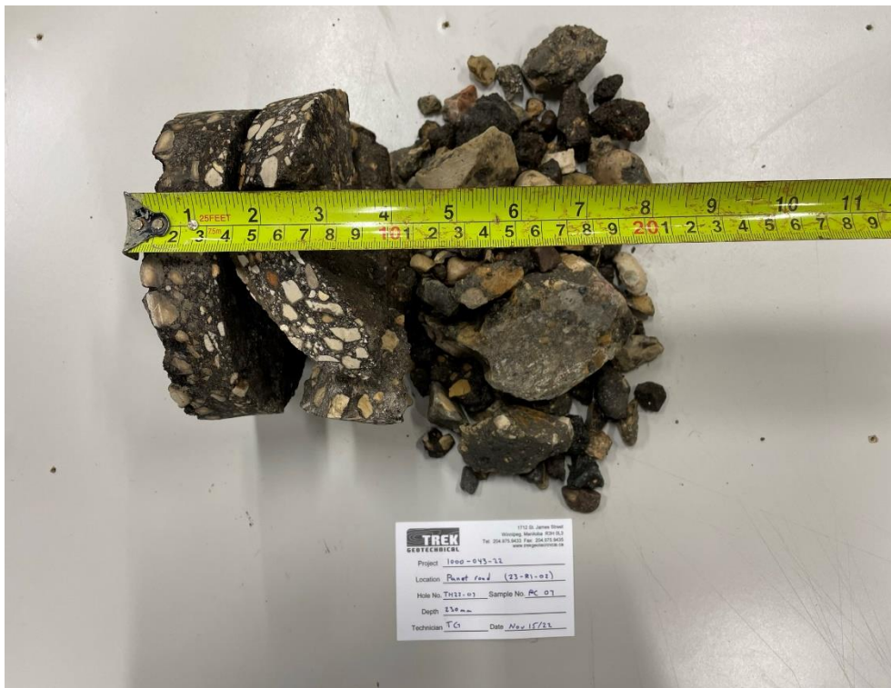
Photo 5: Pavement Core Sample at TH25-07
