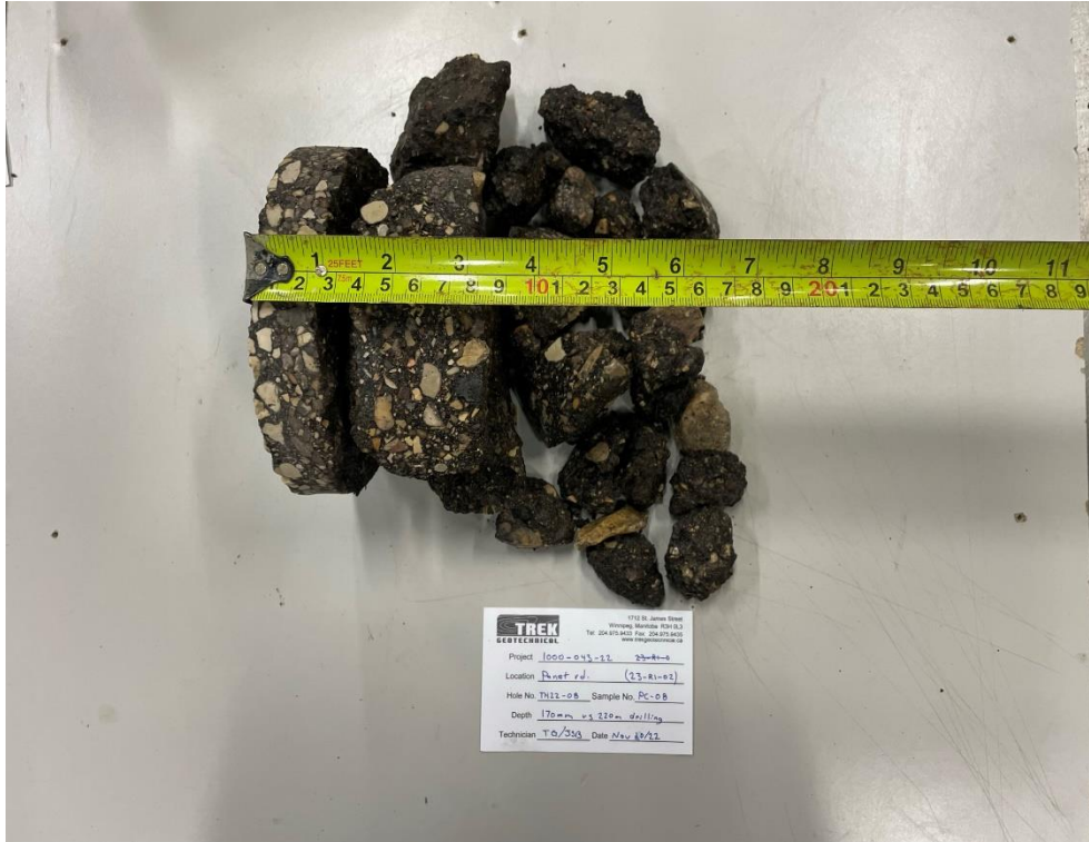
Photo 3: Pavement Core Sample at TH22-08
