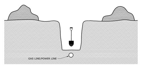
Dig a hole with a shovel directly above the line location until the line is exposed. Take care not to damage the line or coating. Mechanical excavation equipment MUST NOT be used to widen or deepen the hole before exposing the line.
