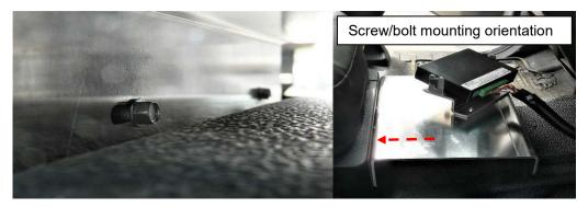
Mounted to the frame on the center console base. <u>DO NOT mount through center console base transmission tunnel.</u>
