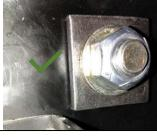
Bolt/nut assembly through chassis frame. If hole is where a transition occurs or on a curved surface in the frame the hole should not be used as a mounting location. However, if the hole location is to be used as a mounting location the following must be followed:
