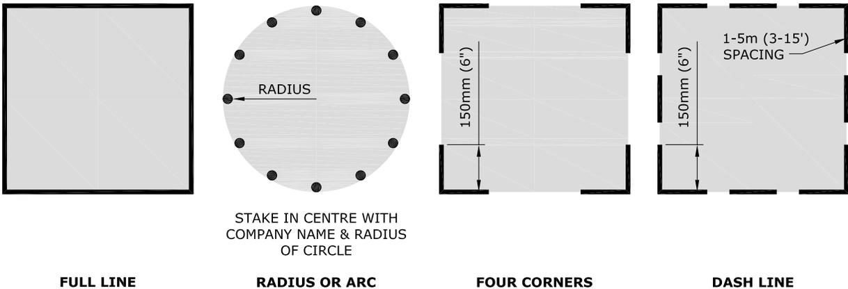
If an excavation is contained within a 5 metre (16 feet) maximum radius then it can be marked with a single white stake at the centre of the excavation. The stake must clearly state the company identifier and the radius of the excavation in black lettering. This information must be conveyed to Manitoba Hydro.
