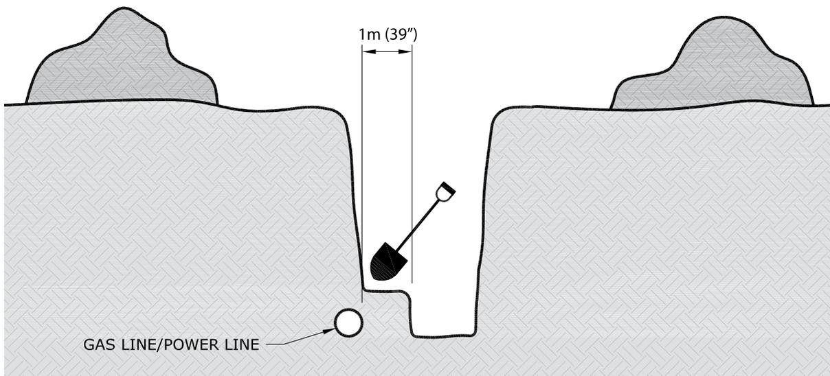
Dig a trench or bell hole 1 metre (39 inches) from the line location, parallel to the line, then hand dig laterally to expose the line.
