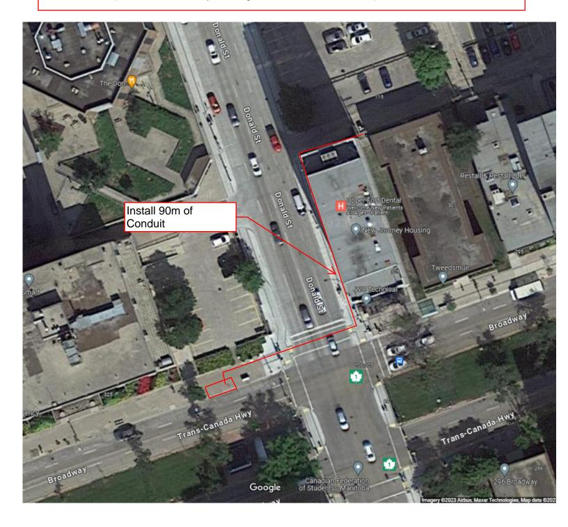
Proposed location of conduit for Connection to Power Source for Smith at Broadway Heated Bus Shelter Power (To be confirmed by Underground Structures Review)
