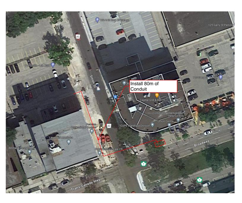
Proposed location of conduit for Connection to existing Power Source for Main at Broadway Heated Bus Shelter Power (To be confirmed by Underground Structures Review)
