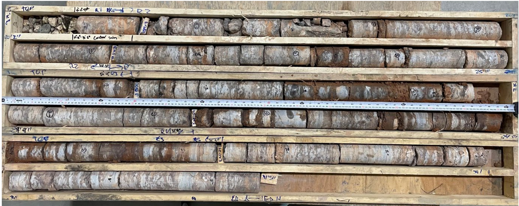
TH23-18 Photo 4: Bedrock core from 4.6 m to 12.4 m (15 ft – 5 in to 41 ft – 5 in)
