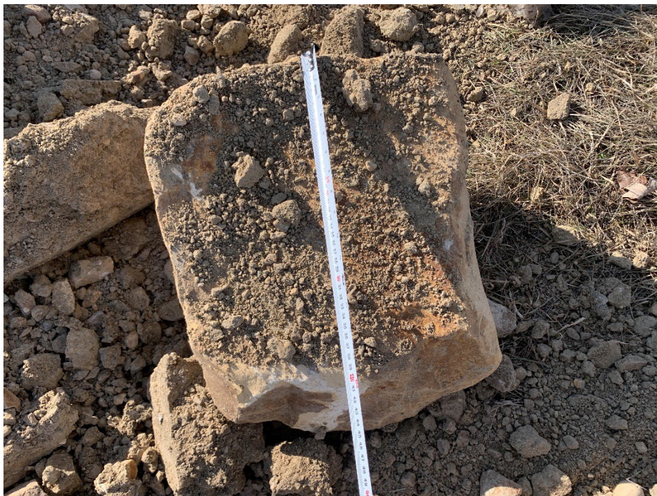
TP24-02 Photo 4: Boulders from silt till (16 inches)
