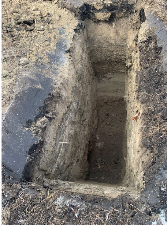
TP24-01 Photo 1: Completed test pit to 5.1 m
