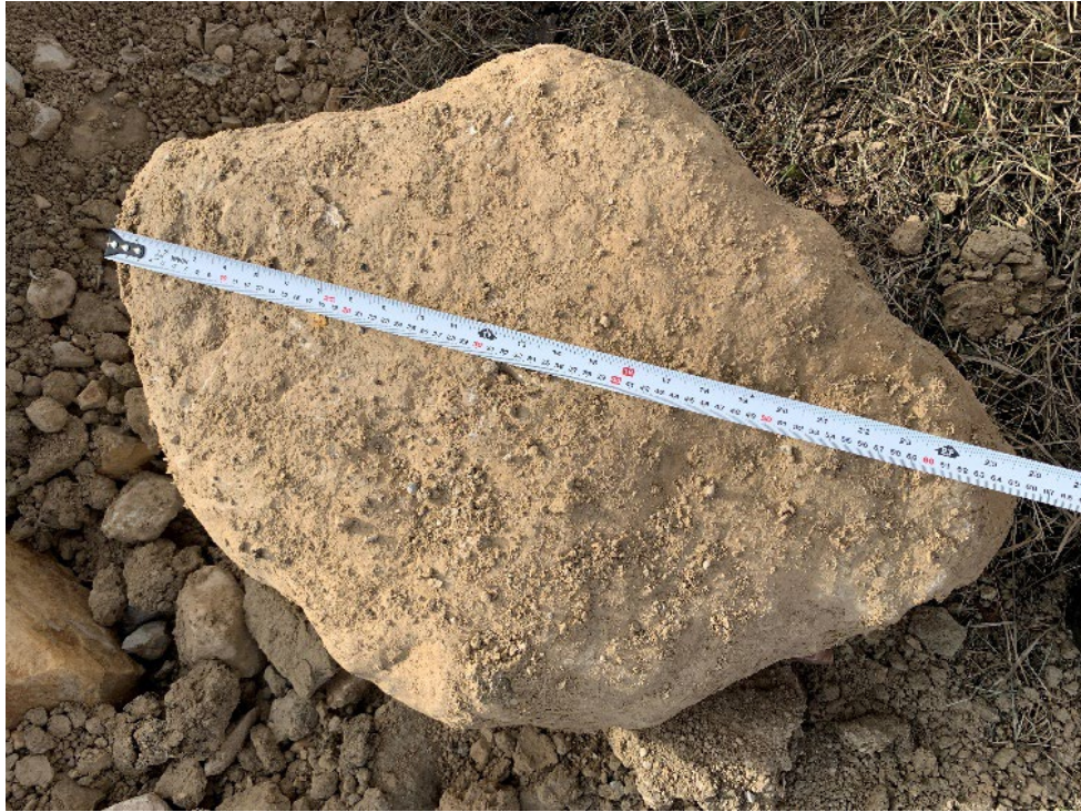
TP24-02 Photo 5: Boulder from silt till (24 inches)
