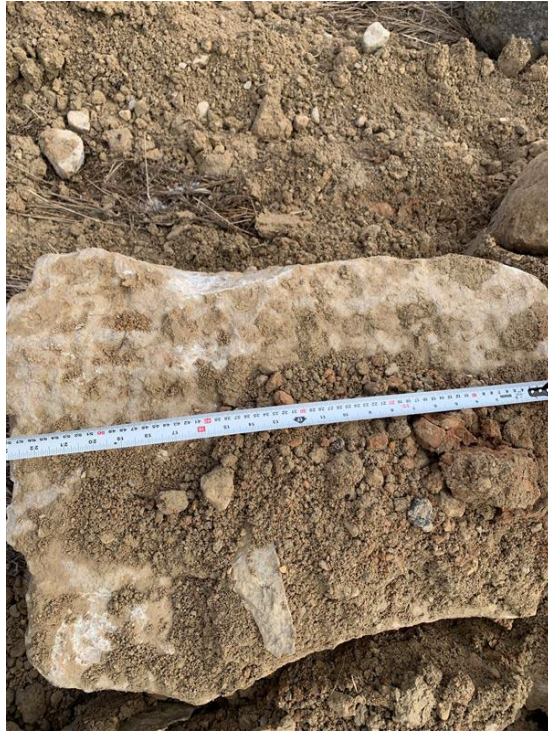
TP24-01 Photo 5: Sedimentary Boulder (22 inches)
