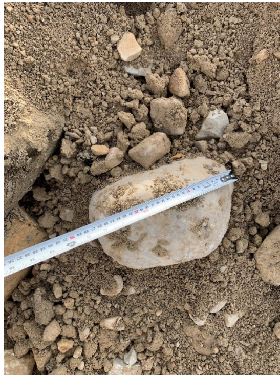
TP24-02 Photo 6: Igneous boulder in silt till
