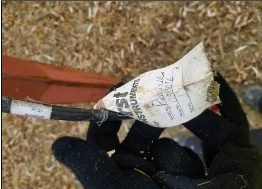
Site 9 - Western Bank Groundwater well near west bridge abutment containing pneumatic piezometer
