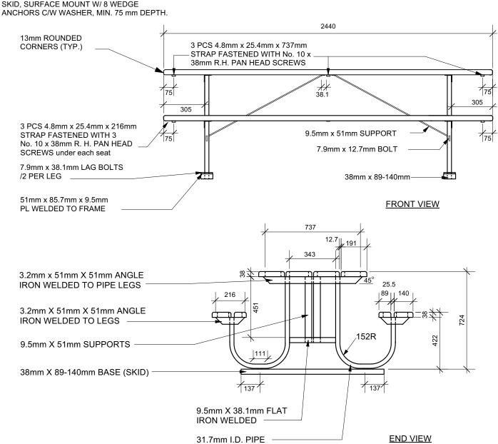
ALL TABLE TOP AND SEAT BOARDS TO BE FASTENED TO ANGLE IRONS WITH 8mm CARRIAGE BOLTS, SECURED WITH WASHER AND NUT.
