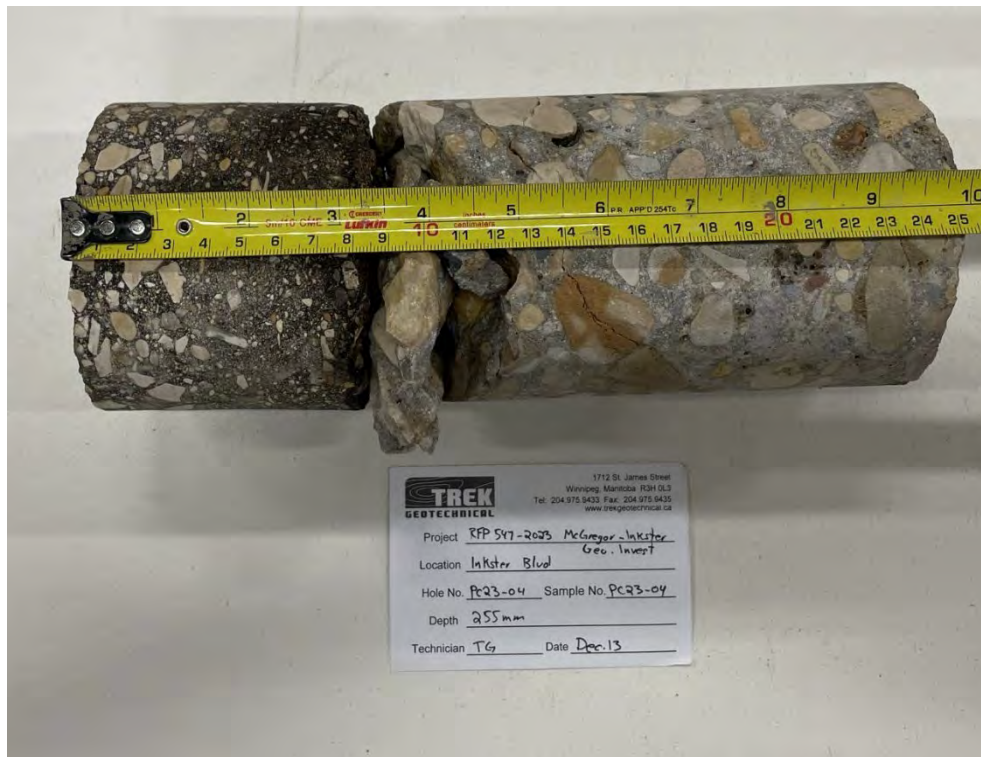
Photo 4: Pavement Core Sample PC23-04
