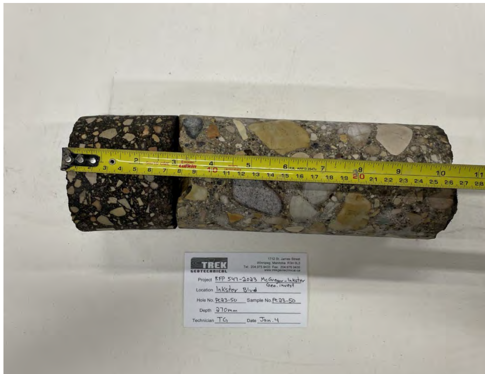
Photo 50: Pavement Core Sample PC23-50
