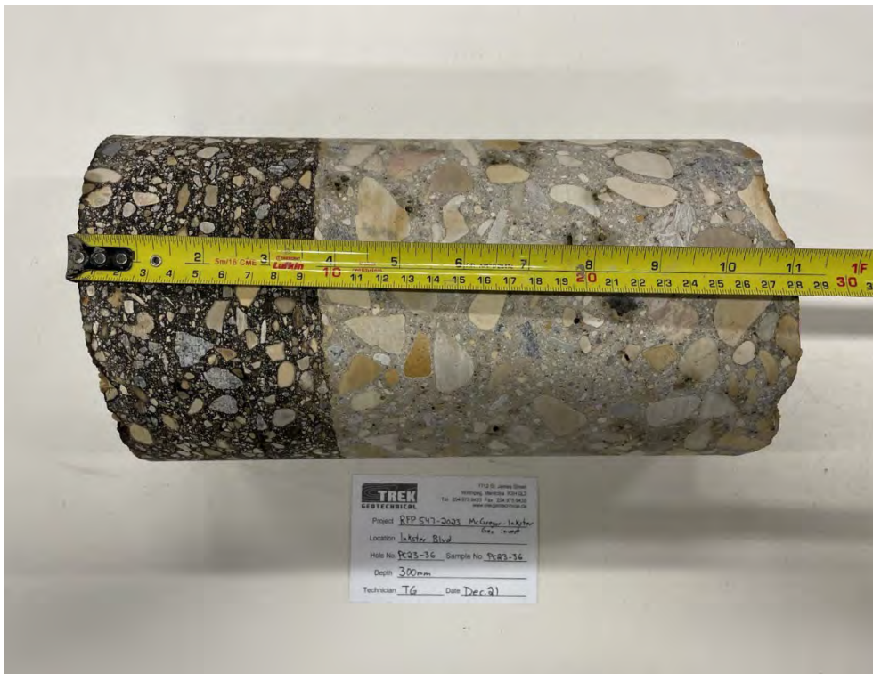
Photo 36: Pavement Core Sample PC23-36
