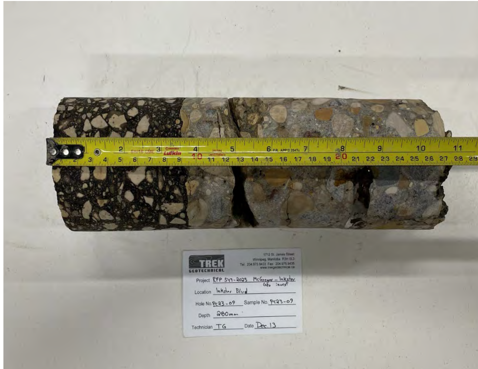
Photo 9: Pavement Core Sample PC23-09
