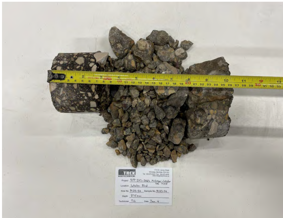
Photo 56: Pavement Core Sample PC23-56
