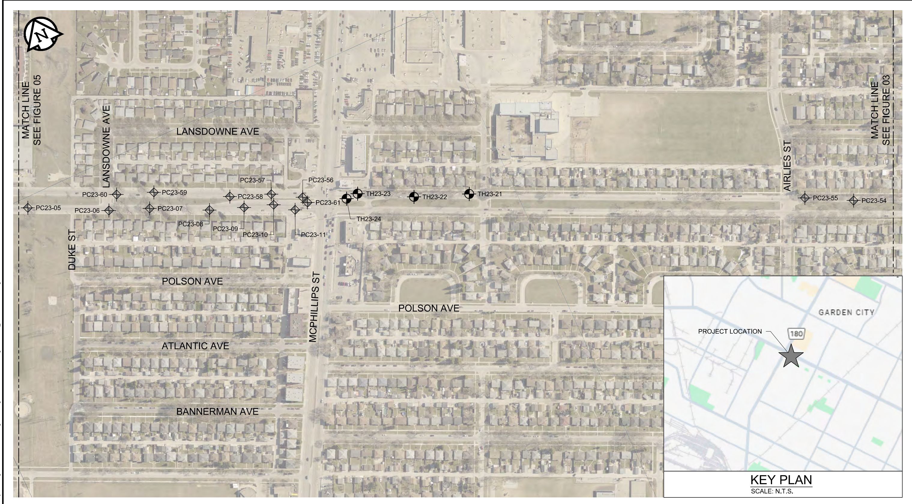
Figure 04 Test Hole and Pavement Core Location Plan
