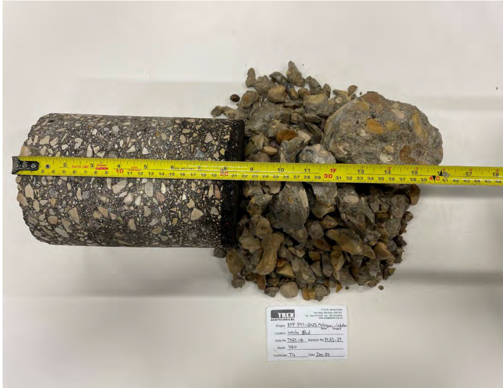
Photo 29: Pavement Core Sample PC23-29
