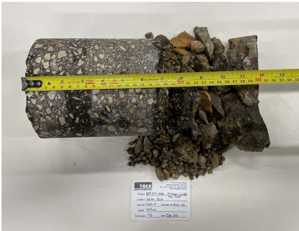
Photo 30: Pavement Core Sample PC23-30
