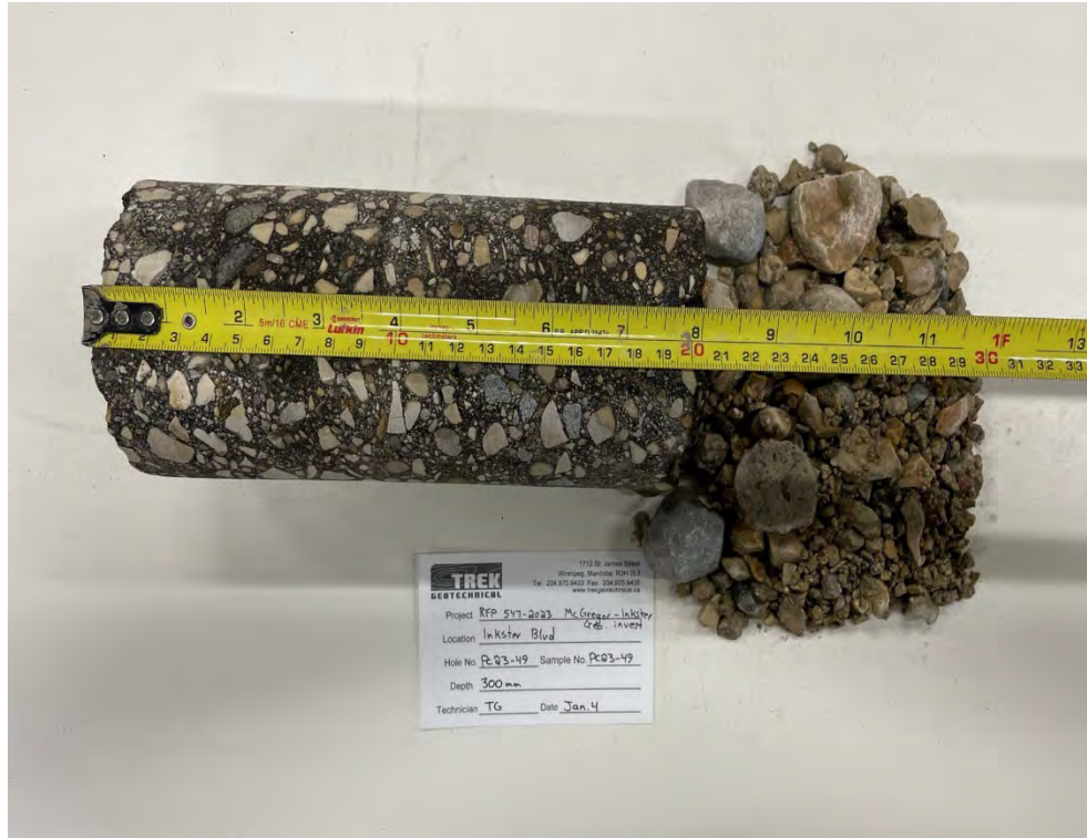
Photo 49: Pavement Core Sample PC23-49
