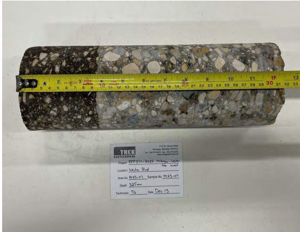
Photo 7: Pavement Core Sample PC23-07
