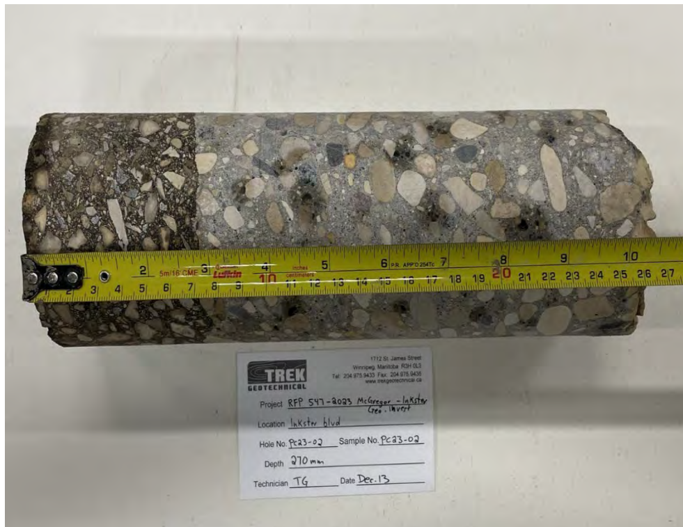
Photo 2: Pavement Core Sample PC23-02
