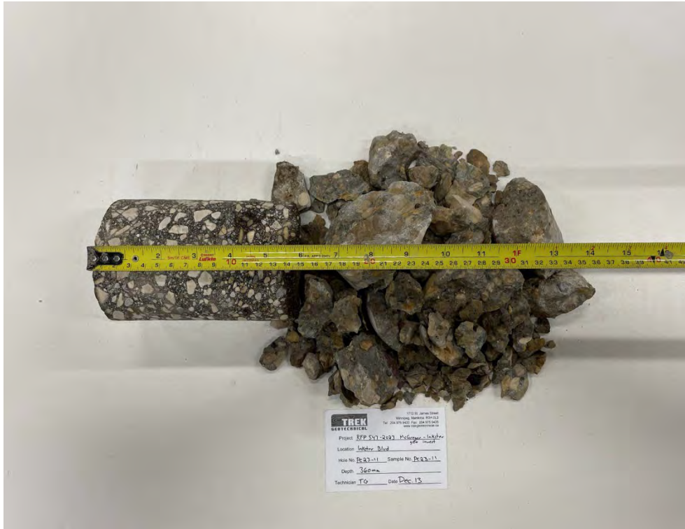
Photo 11: Pavement Core Sample PC23-11
