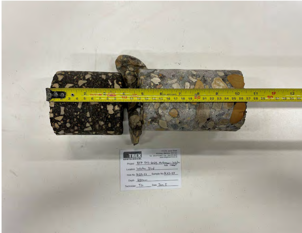
Photo 59: Pavement Core Sample PC23-59
