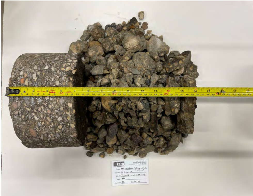
Photo 13: Pavement Core Sample PC23-13
