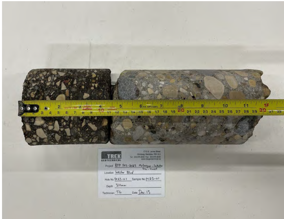
Photo 1: Pavement Core Sample PC23-01
