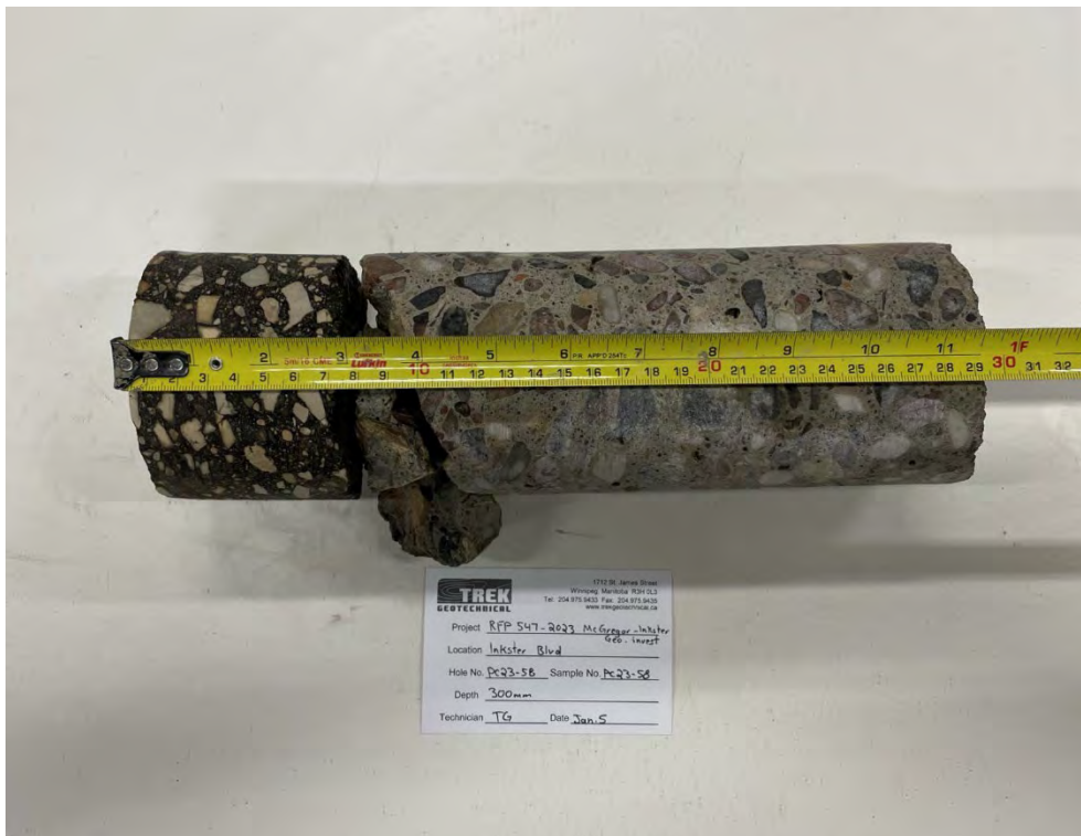
Photo 58: Pavement Core Sample PC23-58
