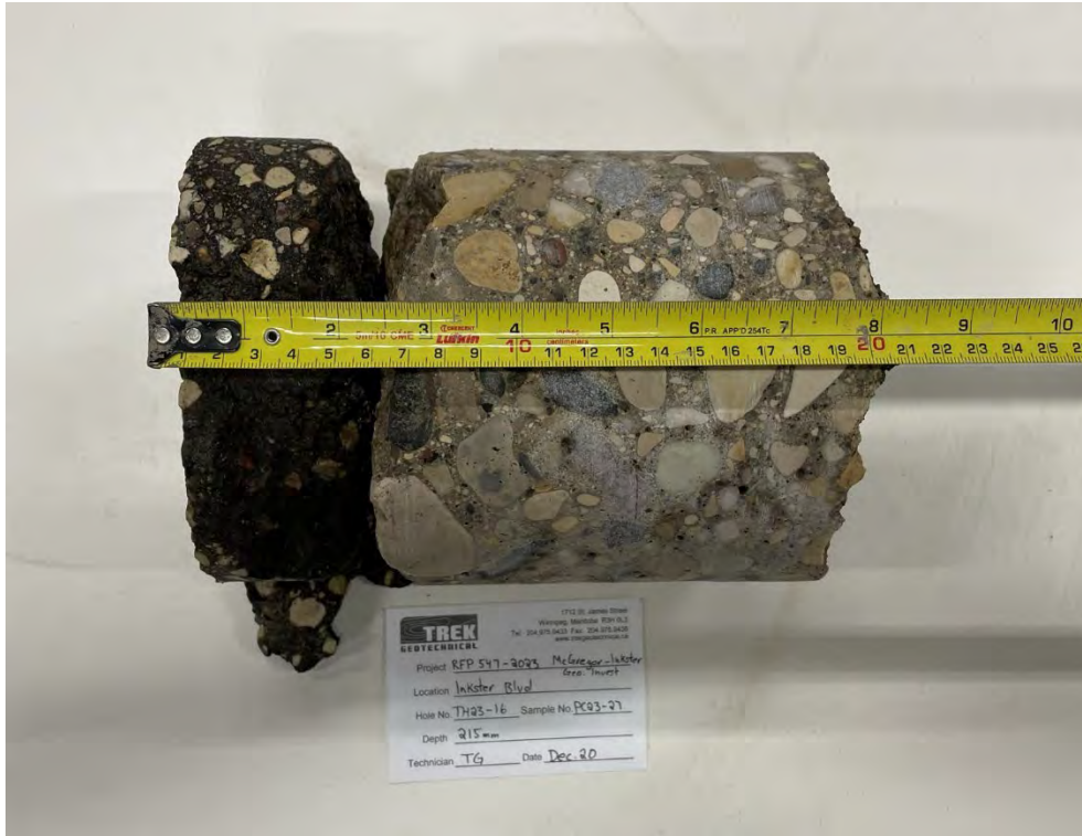
Photo 27: Pavement Core Sample PC23-27
