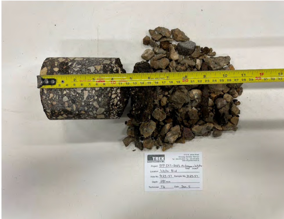
Photo 57: Pavement Core Sample PC23-57
