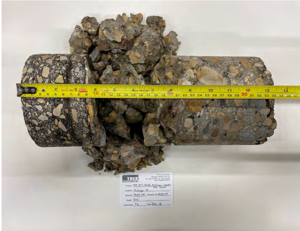
Photo 19: Pavement Core Sample PC23-19
