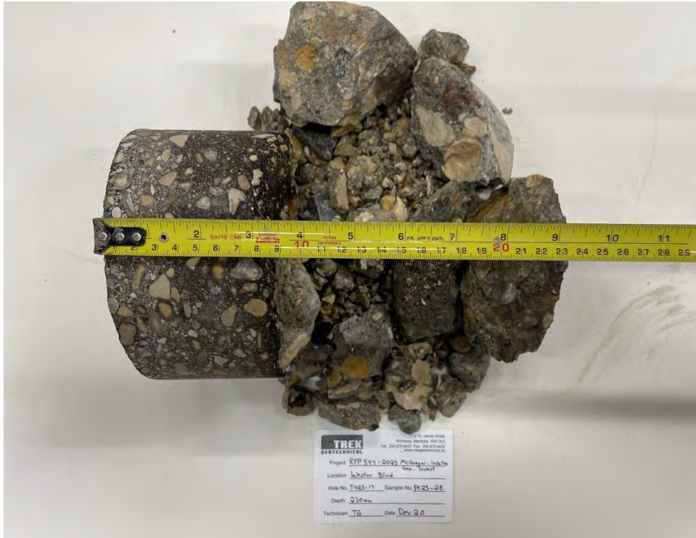
Photo 7: Pavement Core Sample at Test Hole TH23-17
