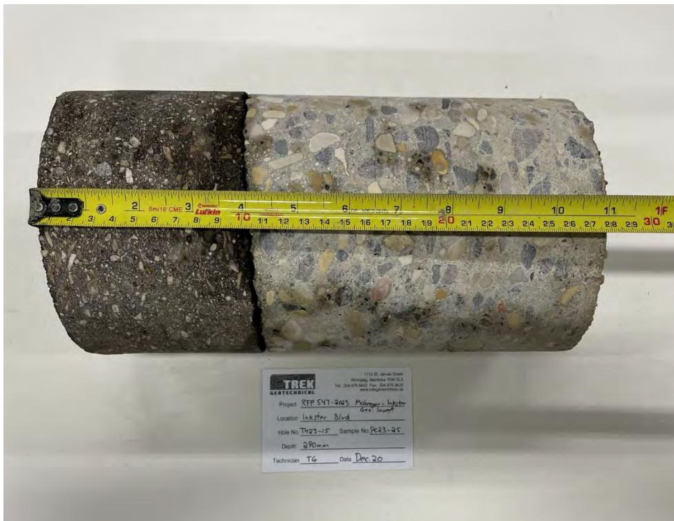
Photo 4: Pavement Core Sample at Test Hole TH23-14
