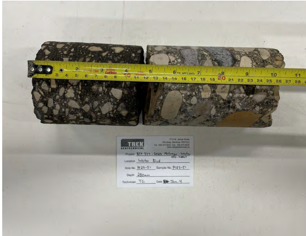
Photo 51: Pavement Core Sample PC23-51
