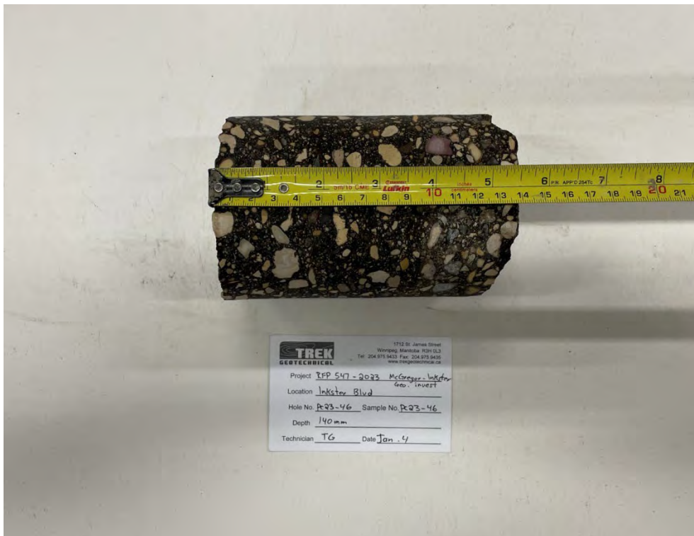
Photo 46: Pavement Core Sample PC23-46
