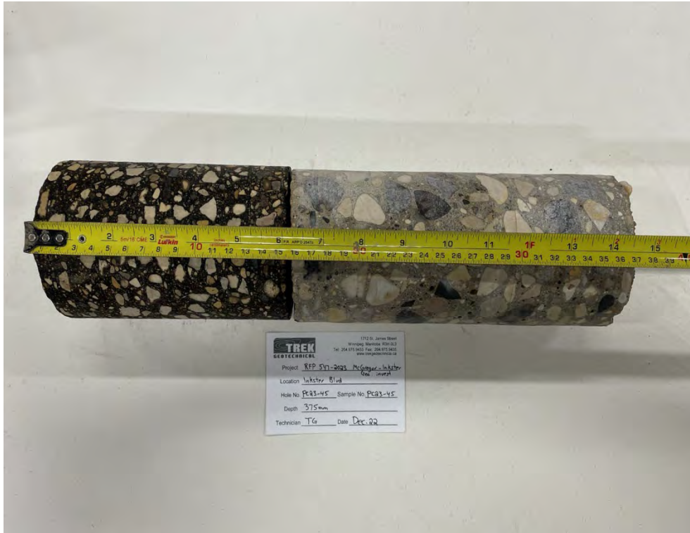
Photo 45: Pavement Core Sample PC23-45
