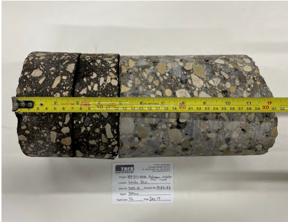
Photo 23: Pavement Core Sample PC23-23
