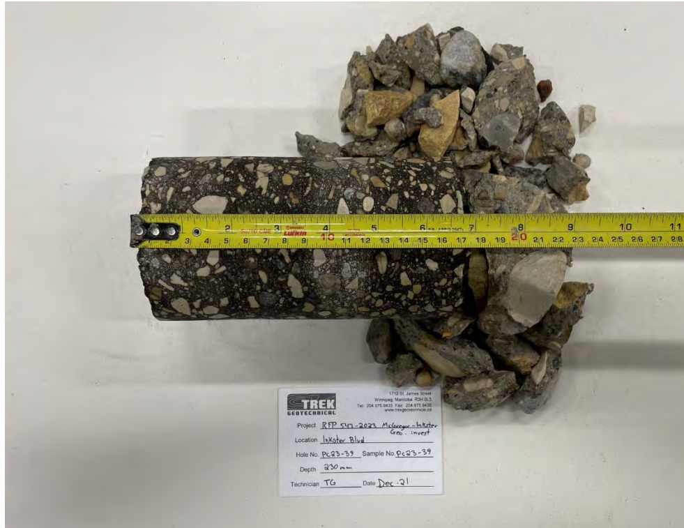
Photo 39: Pavement Core Sample PC23-39
