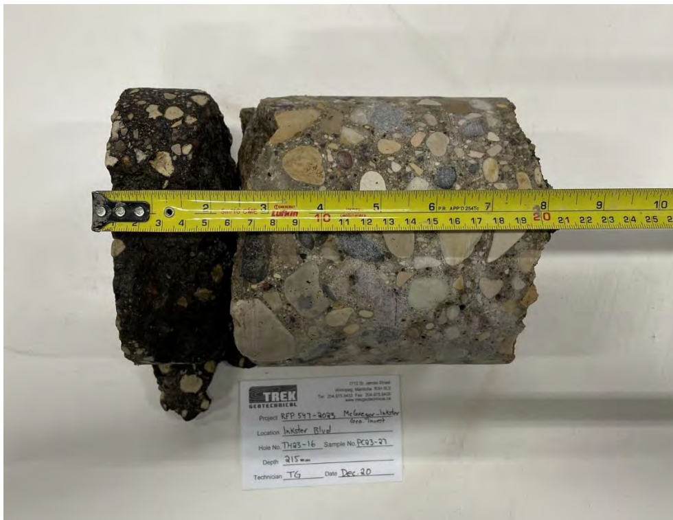
Photo 6: Pavement Core Sample at Test Hole TH23-16
