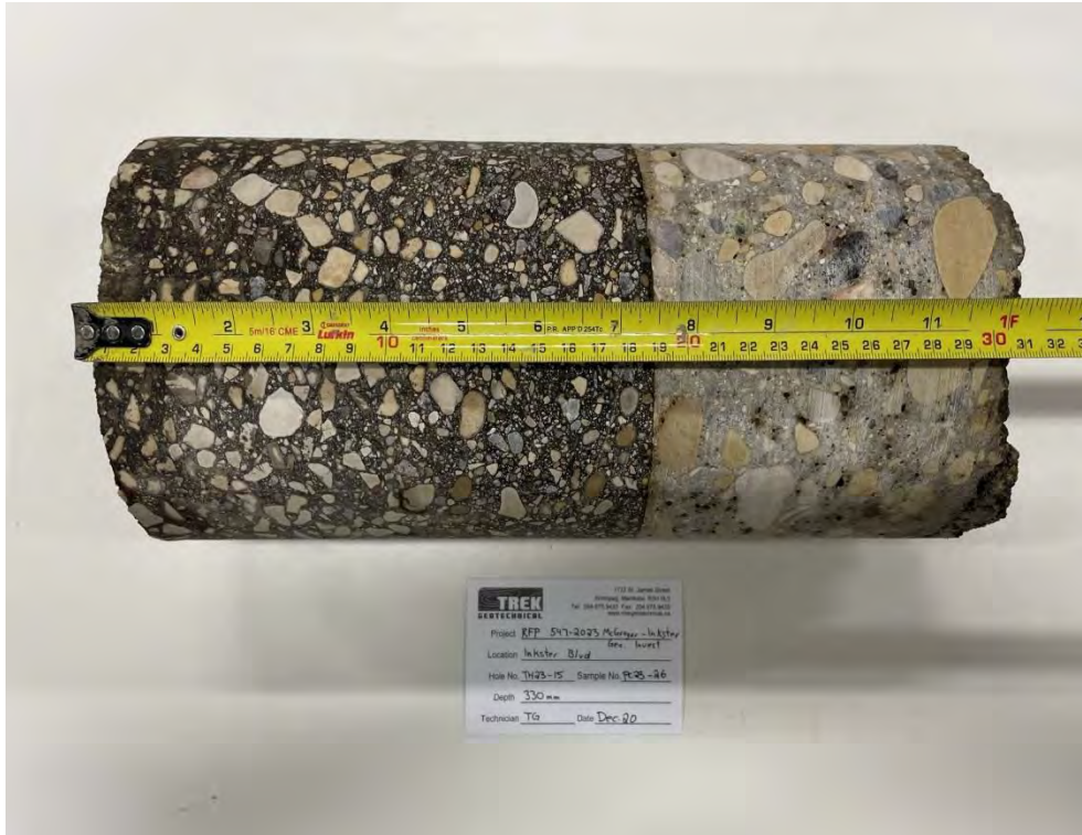
Photo 5: Pavement Core Sample at Test Hole TH23-15
