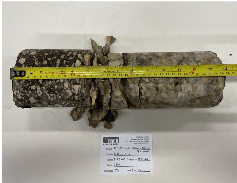
Photo 8: Pavement Core Sample PC23-08
