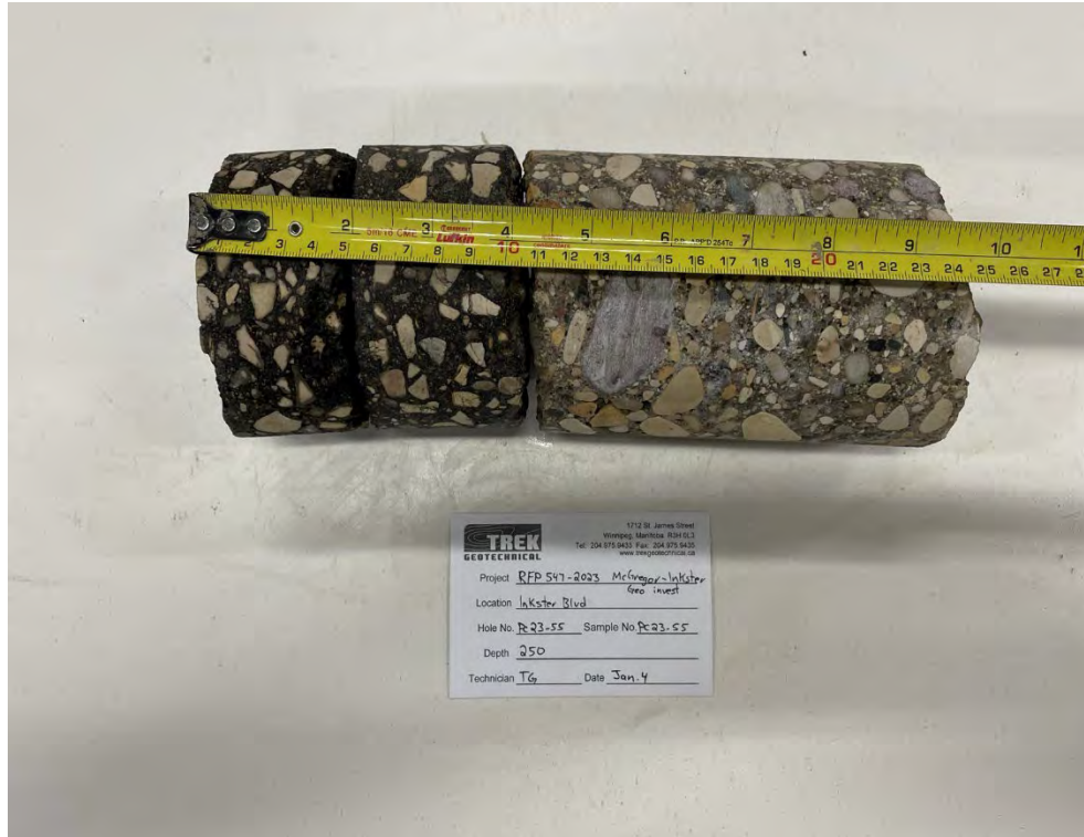
Photo 55: Pavement Core Sample PC23-55
