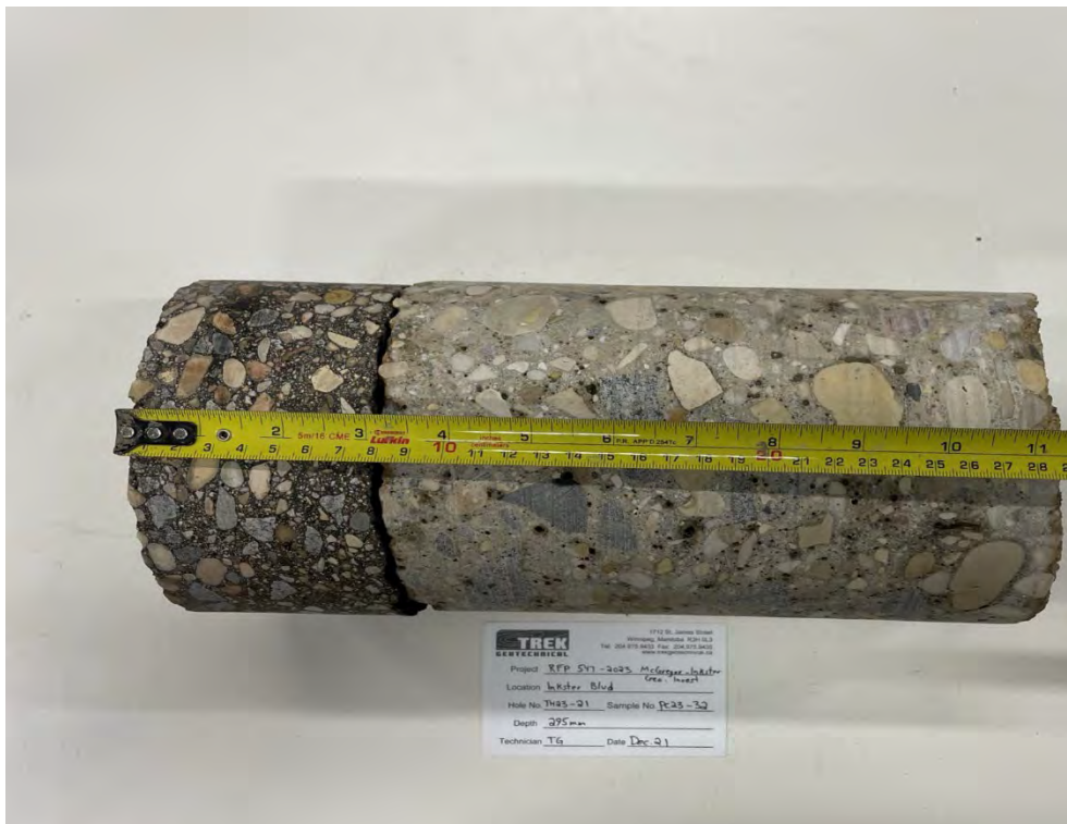
Photo 32: Pavement Core Sample PC23-32
