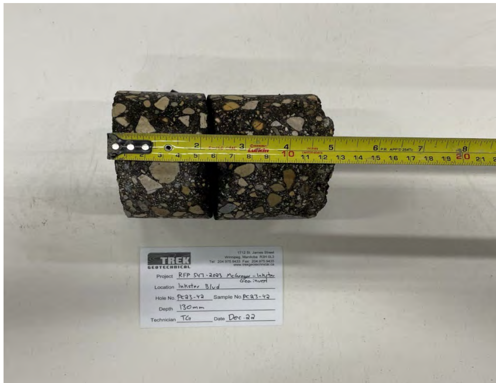
Photo 42: Pavement Core Sample PC23-42
