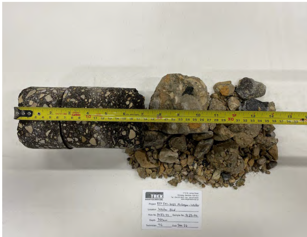
Photo 44: Pavement Core Sample PC23-44
