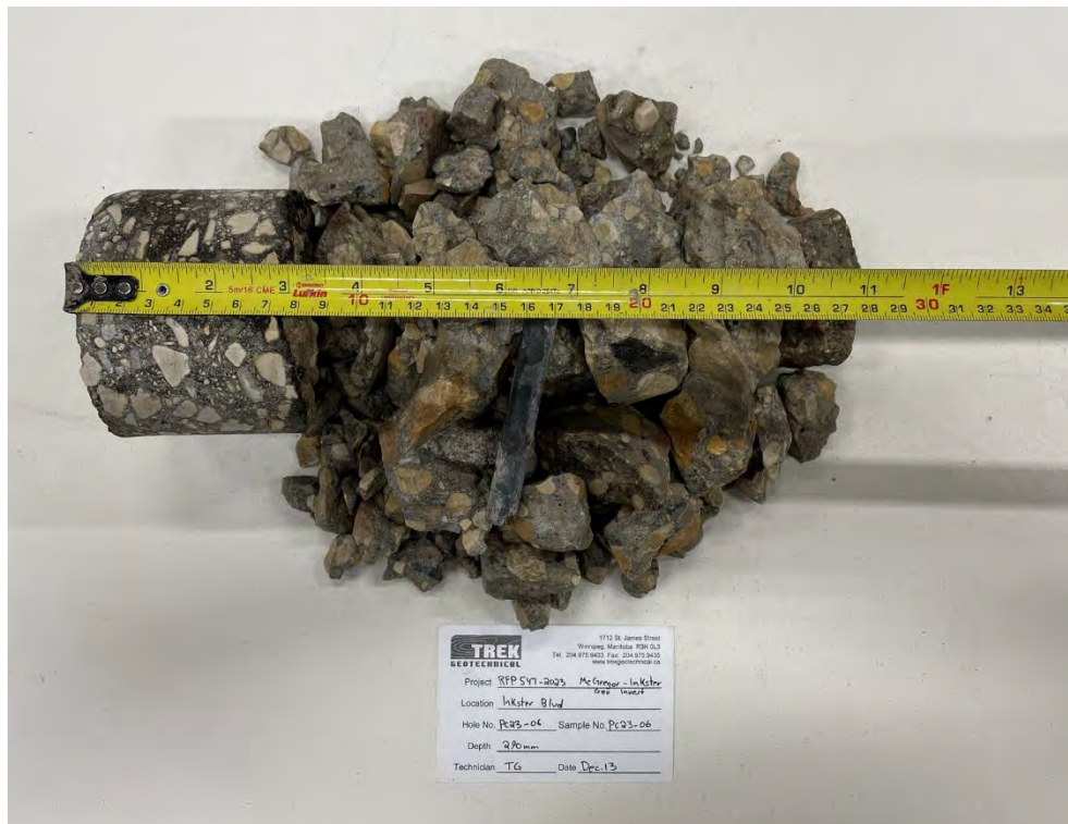
Photo 6: Pavement Core Sample PC23-06
