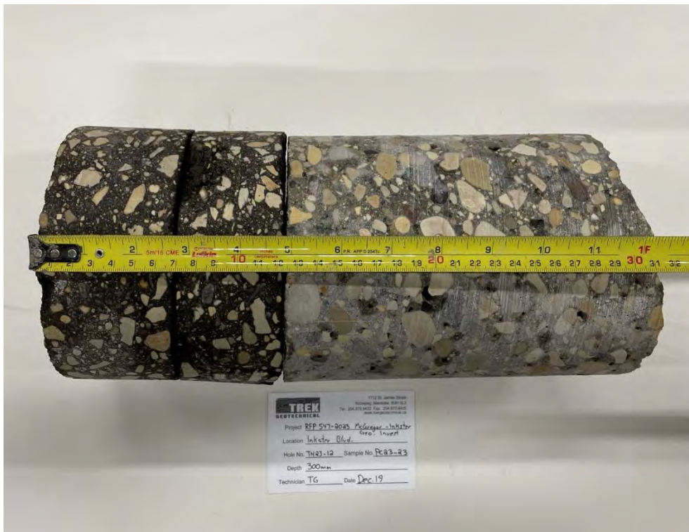
Photo 2: Pavement Core Sample at Test Hole TH23-12
