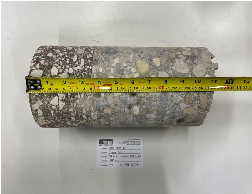
Photo 1: Pavement Core Sample at TH24-01
