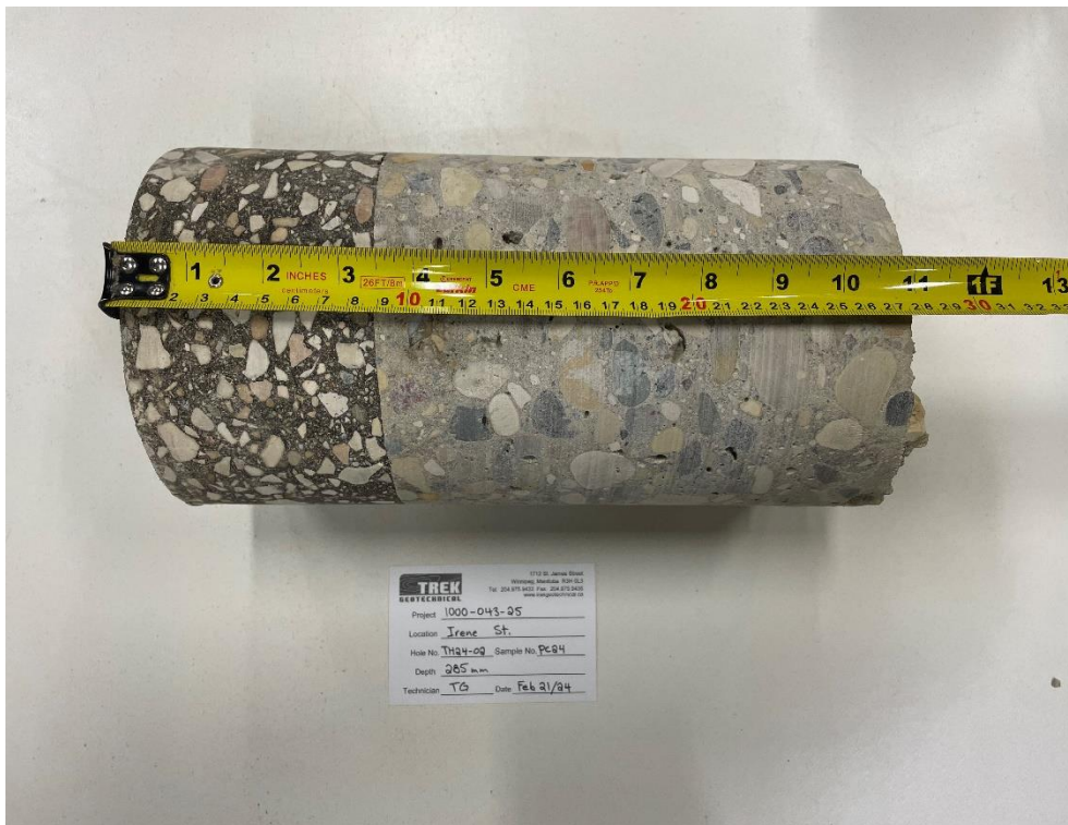
Photo 2: Pavement Core Sample at TH24-02
