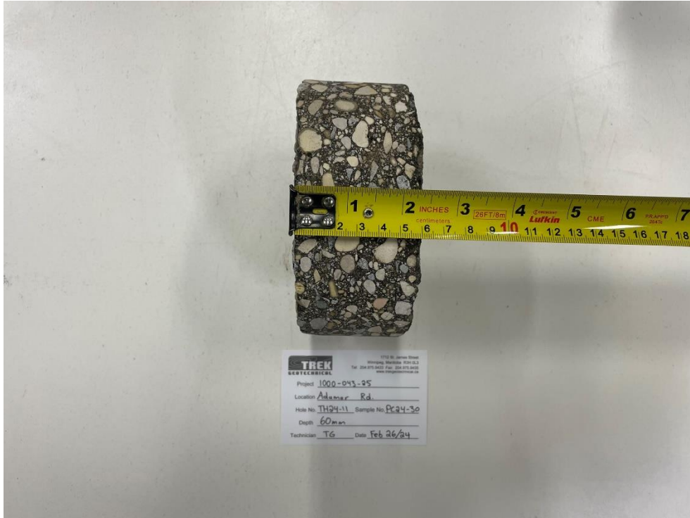
Photo 3: Pavement Core Sample at TH24-11
