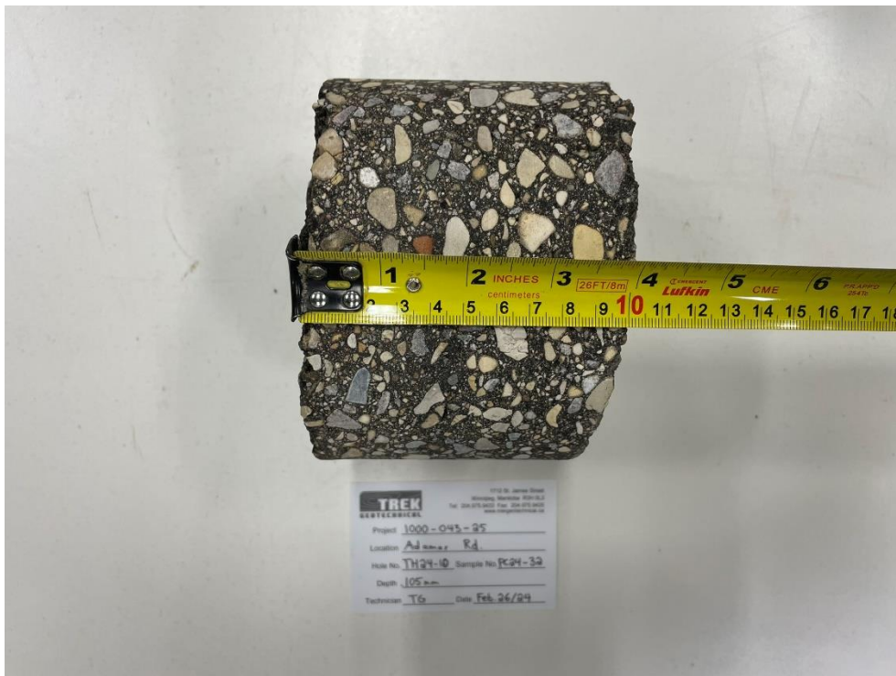
Photo 2: Pavement Core Sample at TH24-10
