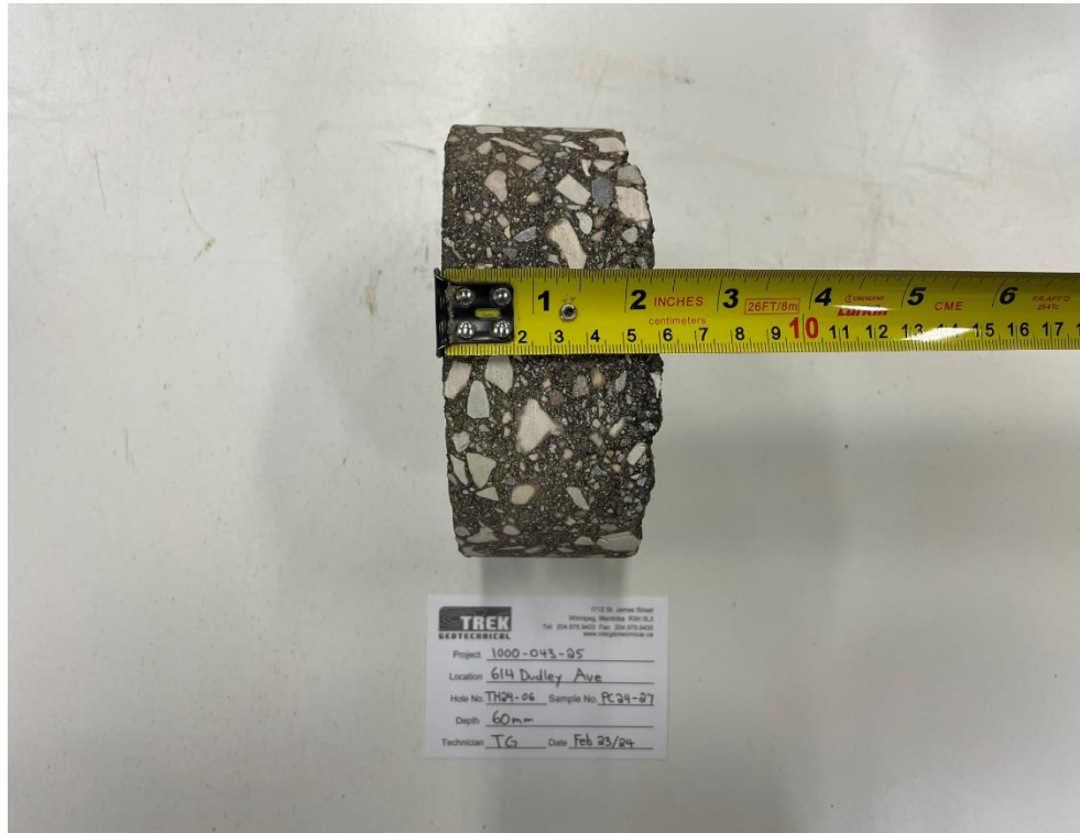
Photo 1: Pavement Core Sample at TH24-06
