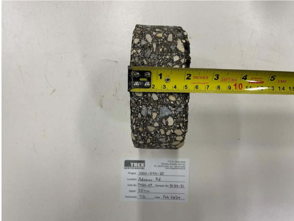
Photo 1: Pavement Core Sample at TH24-09
