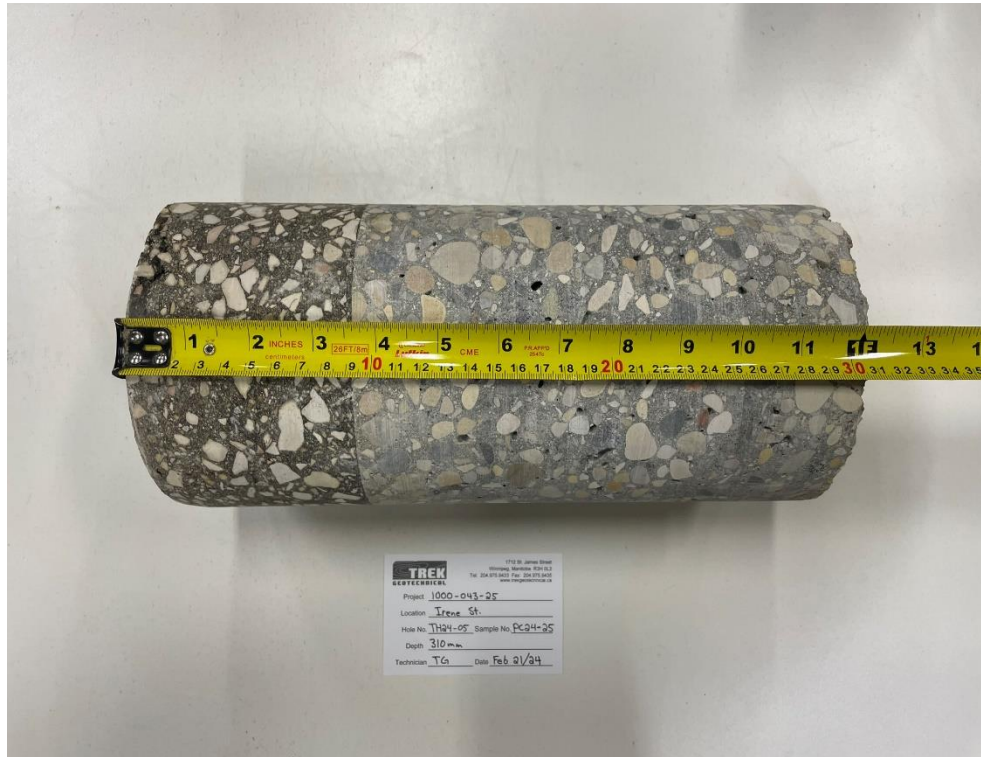
Photo 5: Pavement Core Sample at TH24-05
