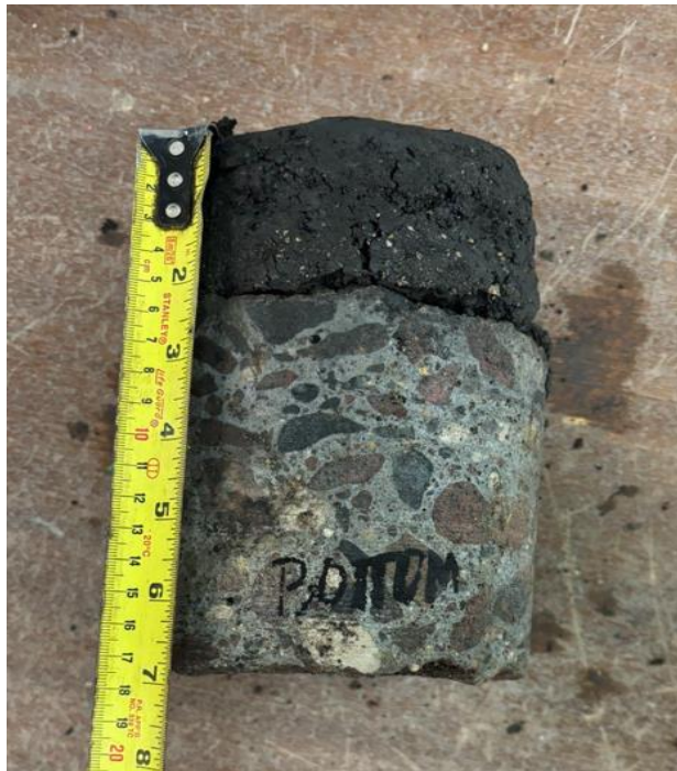
Hartford Ave, EBL, Core 25 (Asphalt Thk 50.8mm, Conc Thk 127mm)
