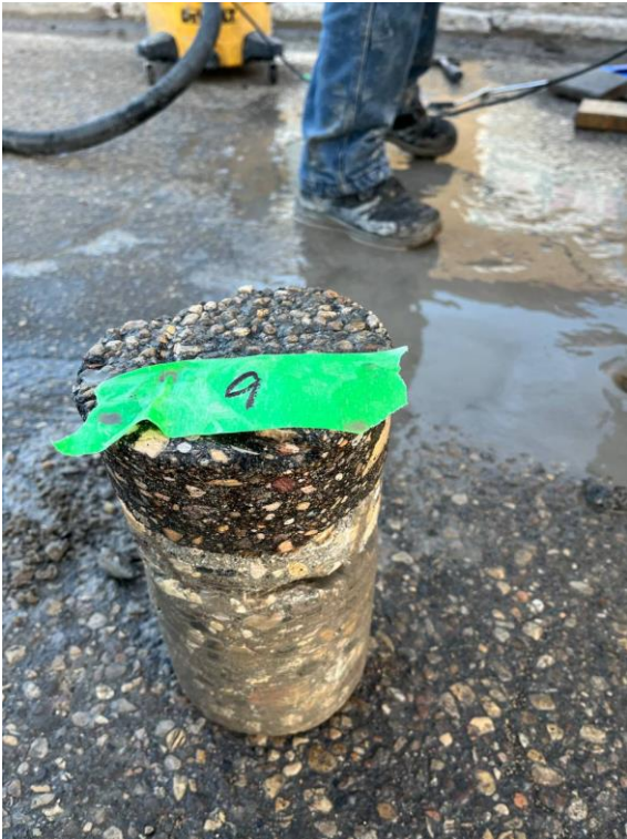
Figure 9. Photo showing core 9 showing deterioration of asphalt and concrete at joint
