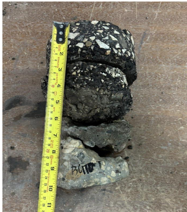
Hartford Ave, WBL, Core 30 (Asphalt Thk 114.3mm; Conc Thk 139.7)
