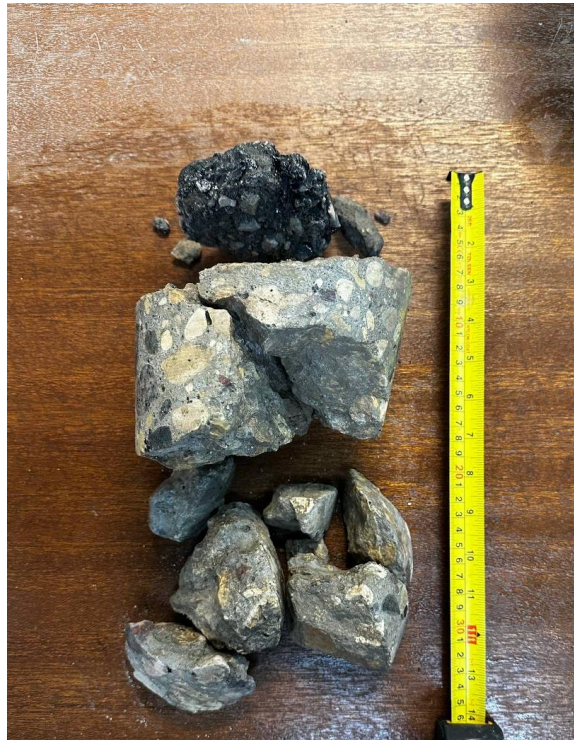
Figure 13. Core 13 showing deterioration of asphalt cold mix was present and concrete presented shear deterioration. Void existed between the pavement and base surface
