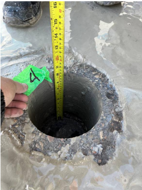
Figure 4. Photos showing Core 4 pavement for compressive strength test. Rebar present in concrete core. Compressive strength can not be done in this core.
