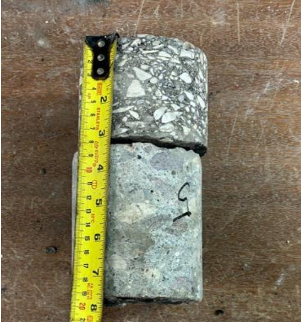
Hartford Ave, WBL, Core 23 (Asphalt Thk 76.2mm, Conc Thk 120.7mm)
