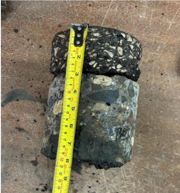
Hartford Ave, WBL, Core 27 (Asphalt Thk 63.5mm; Conc Thk 139.7mm)
