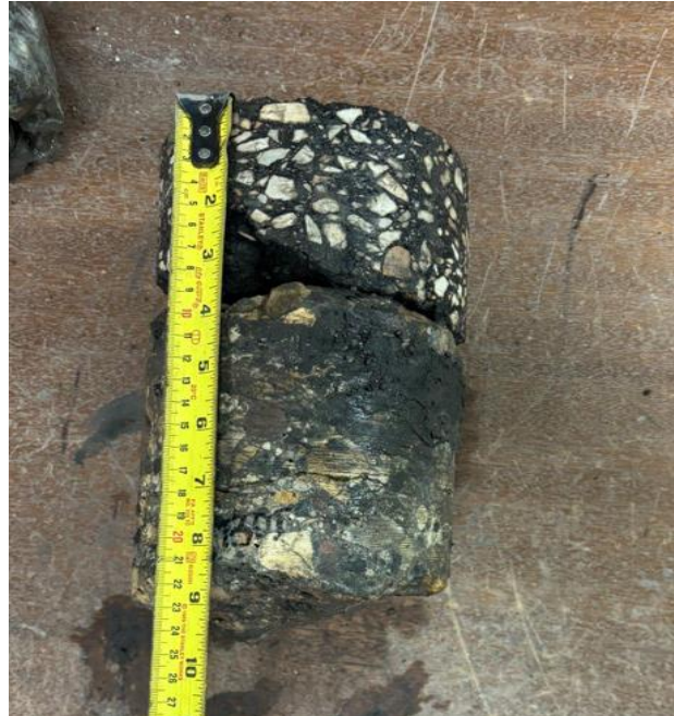
Hartford Ave, WBL, Core 28 (Asphalt Thk 82.6mm; Conc Thk 158.7mm)
