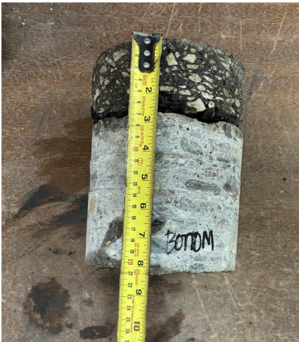
Hartford Ave, WBL, Core 29 (Asphalt Thk 63.5mm; Conc Thk 146.1mm)
