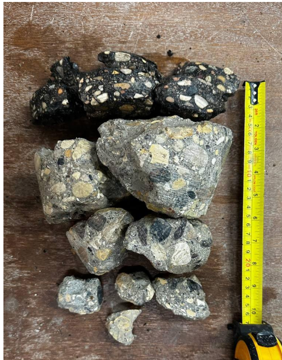
Figure 10. Photo showing core 10 showing deterioration and void space of asphalt and concrete. Void existed between the pavement and base surface
