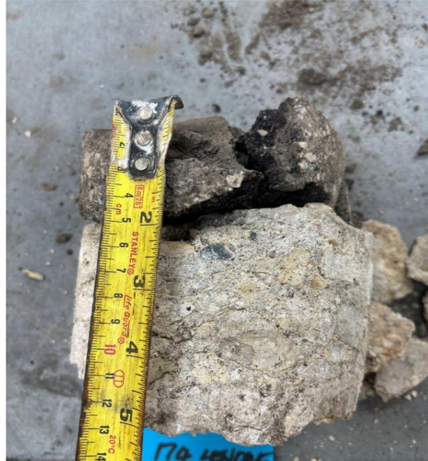
Ruby St - Lenore St Backlane, NBL, Core 38 (Asphalt Thk 51mm; Conc Thk 102)
