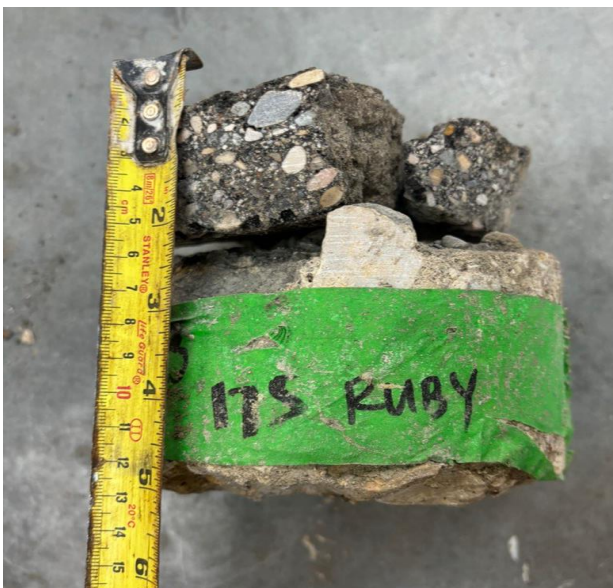
Ruby St - Lenore St Backlane, SBL, Core 39 (Asphalt Thk 40mm; Conc Thk 80)
