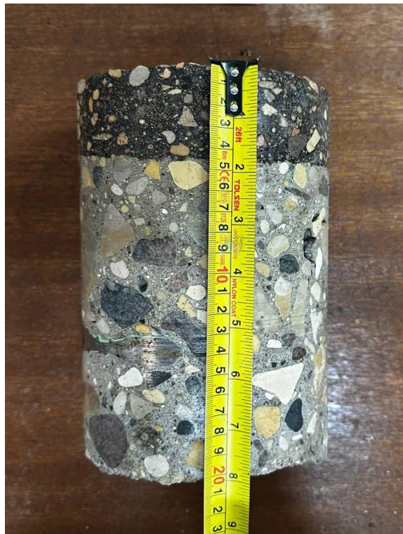
Figure 4. Photos showing Core 4 pavement for compressive strength test. Rebar present in concrete core. Compressive strength can not be done in this core.
