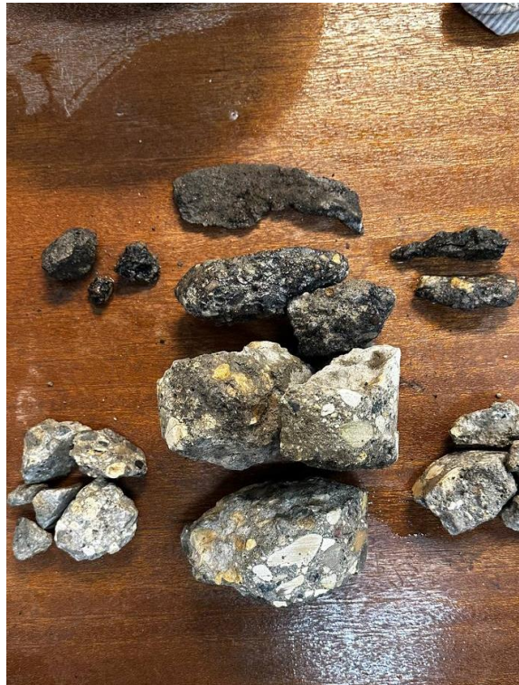
Figure 11. Photo showing core 11 showing deterioration and void space of asphalt and concrete at joint
