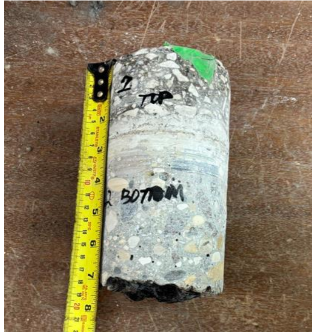
Hartford Ave, WBL, Core 20 (Asphalt Thk 69.9mm; Conc Thk 87.93)
