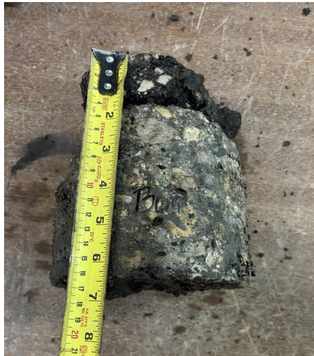
Hartford Ave, WBL, Core 26 (Asphalt Thk 50.8mm, Conc Thk 127mm)
