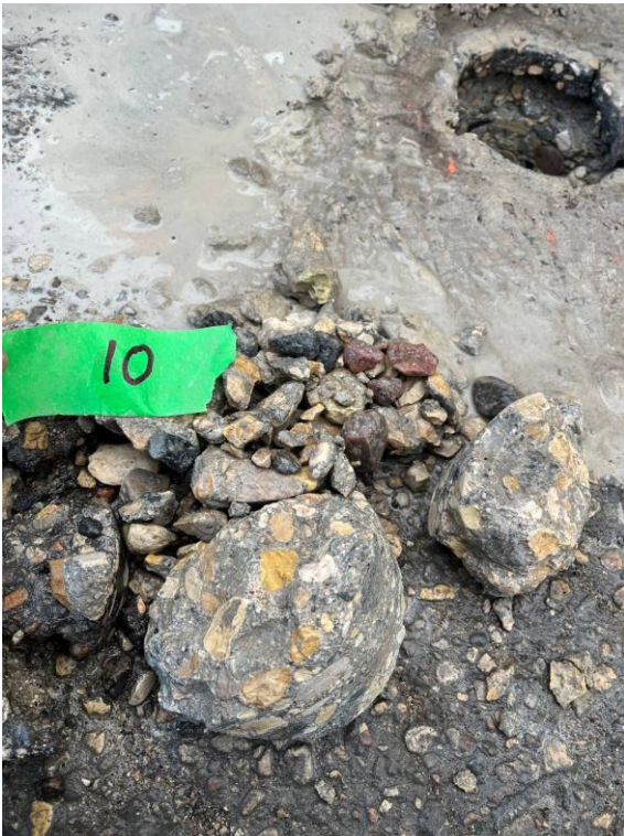
Figure 10. Photo showing core 10 showing deterioration and void space of asphalt and concrete. Void existed between the pavement and base surface
