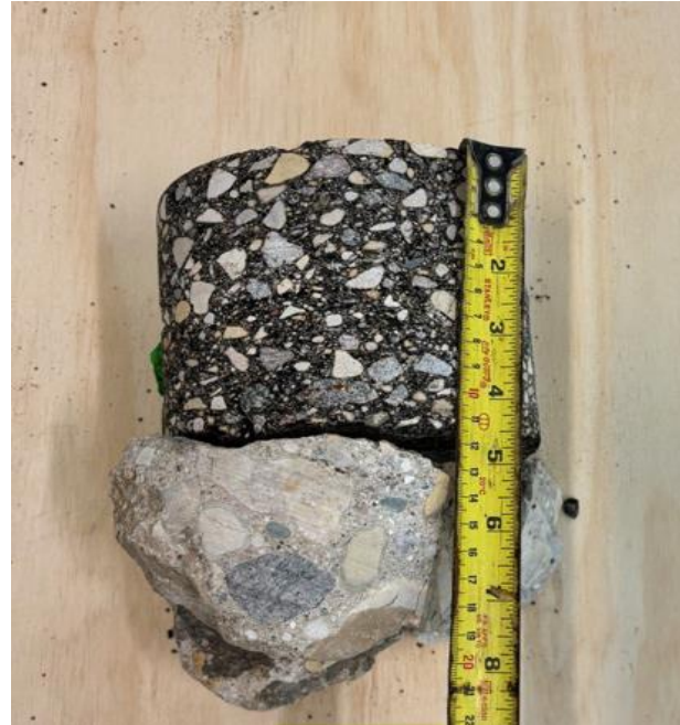
Lipton St, SBL, Core 32 (Asphalt Thk 100.4mm; Conc Thk 128.2mm)
