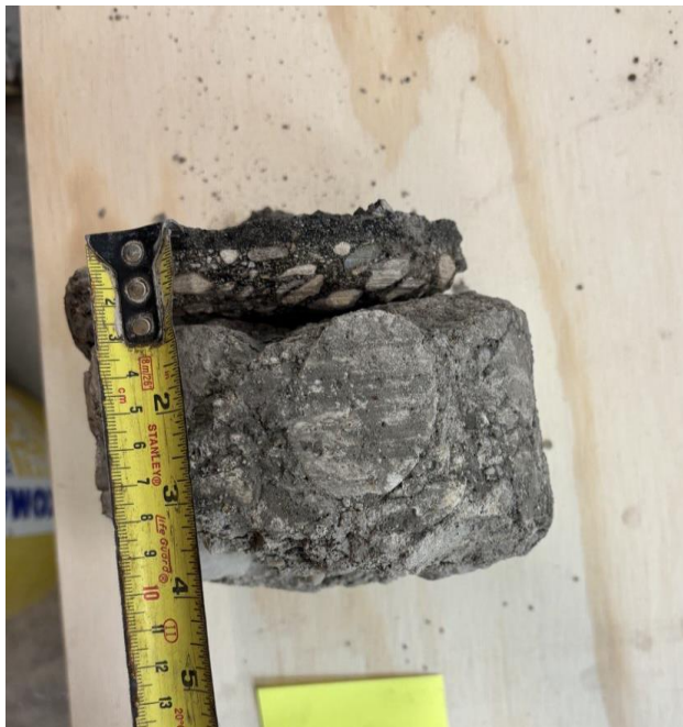
Lipton St, NBL, Core 35 (Asphalt Thk 51mm; Conc Thk 114.1mm)
