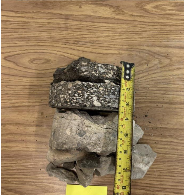
Lipton St, NBL, Core 31 (Asphalt Thk 63.5mm; Conc Thk 165.1mm)
