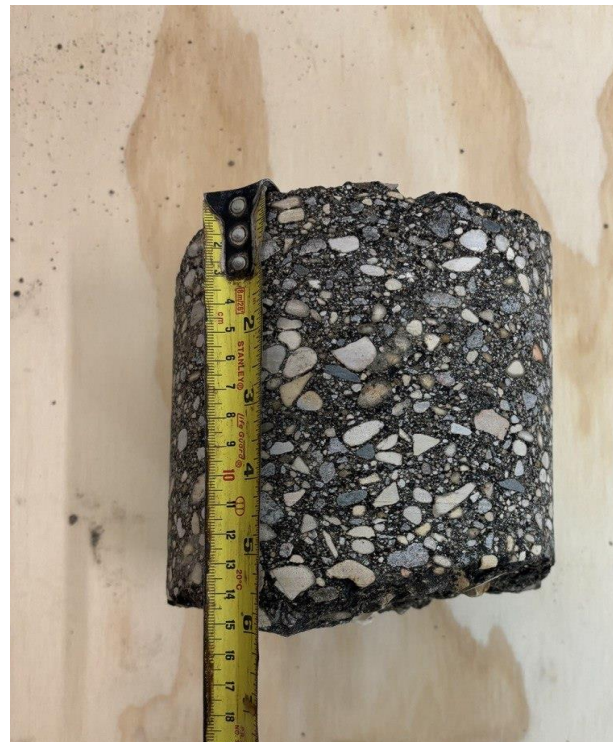
Lipton St, SBL, Core 34 (Asphalt Thk 150mm)
