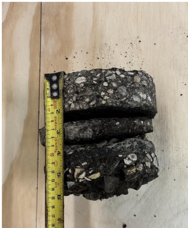
Lipton St, NBL, Core 33 (Asphalt Thk 152.4mm)
