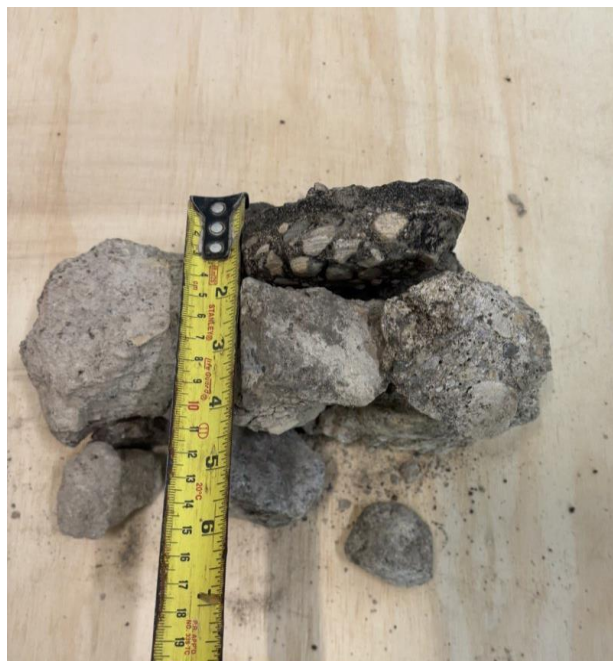
Lipton St, SBL, Core 36 (Asphalt Thk 52mm; Conc Thk 100.4mm)
