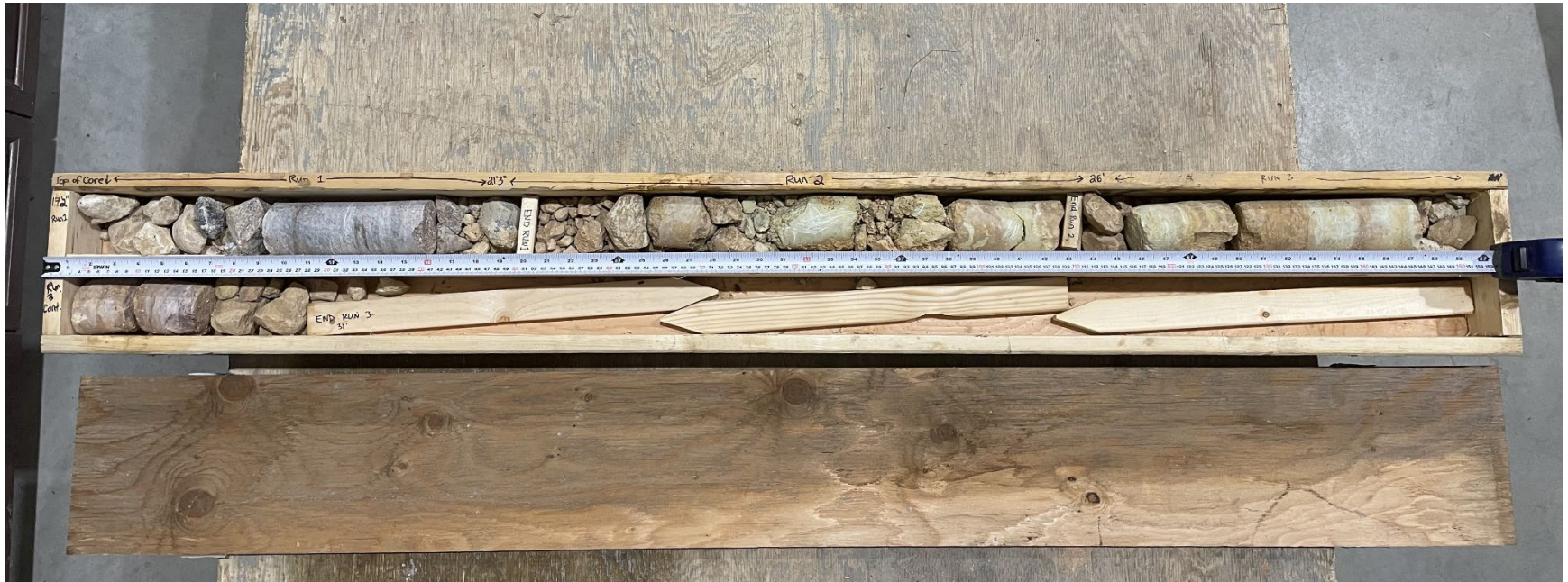
TH23-09 Photo 6: Bedrock Core, 6.45 m to 9.75 m (21 ft-3 in to 32 ft)
