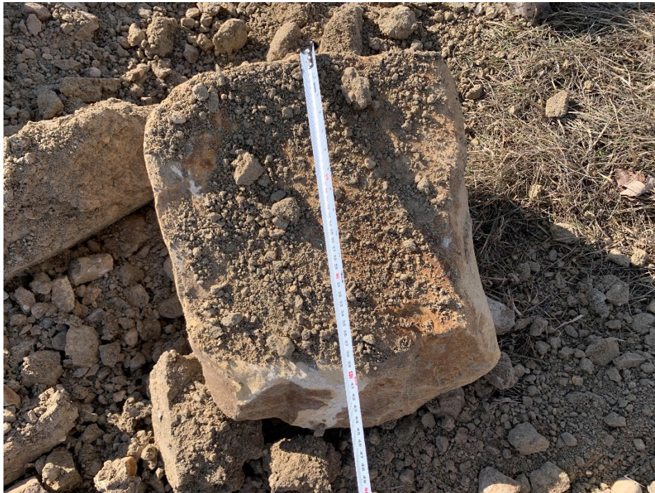
TP24-02 Photo 4: Boulders from silt till (16 inches)
