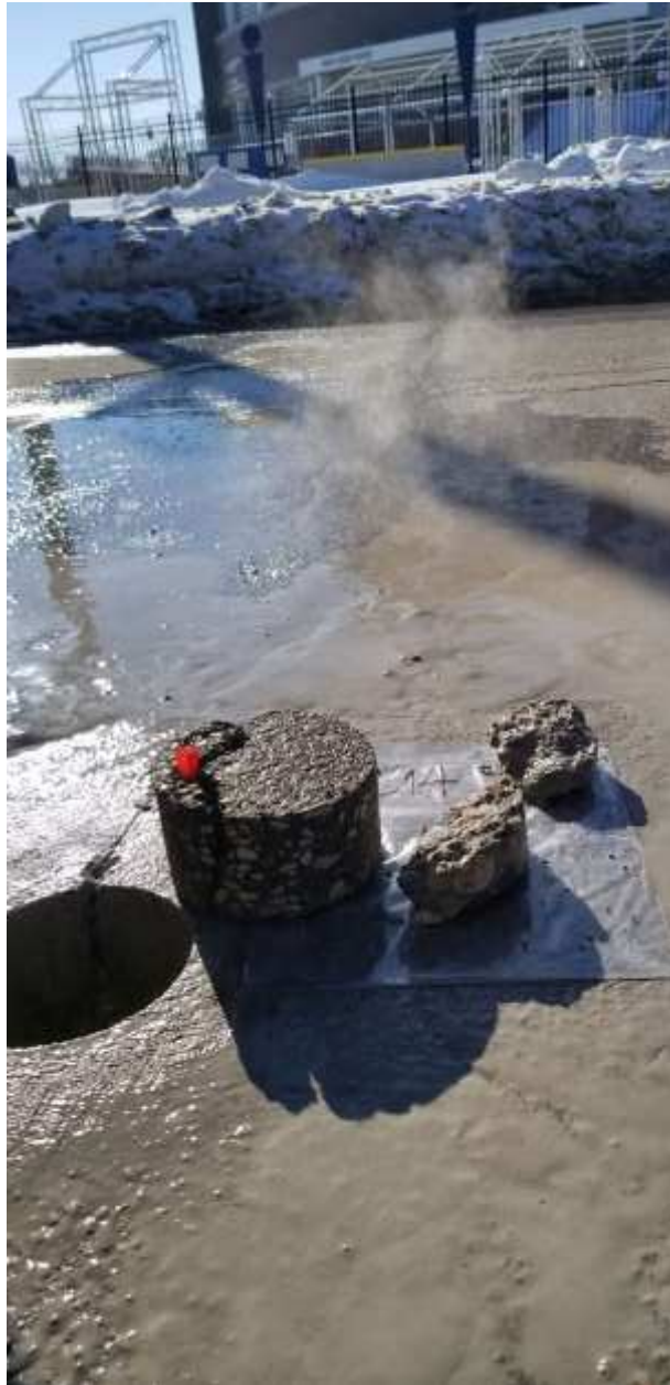
South bound transvers joint, Sta. 0+233. Could not extract concrete core due to crumbling
