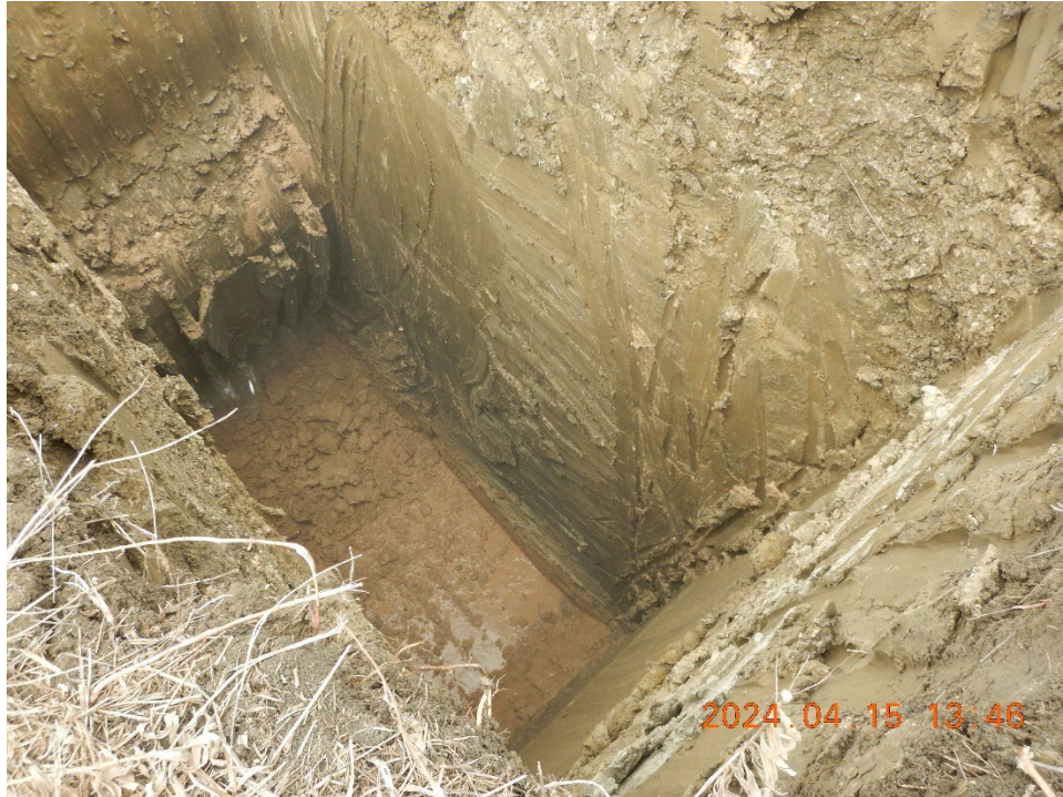
TP24-03 Photo 1: Top of bedrock encountered at 4.6 m
