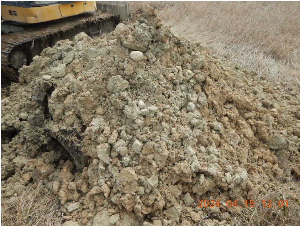
TP24-04 Photo 2: Gravel and cobbles encountered in silt till
