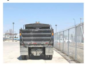
Beacon centered on lip of box with protective cage (recommended), providing 360° visibility in combination with strobe lights amber and blue on rear of vehicle (blue - snow removal operations only)
