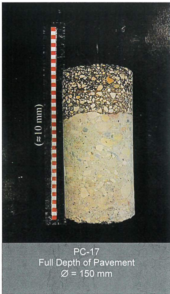
Photograph 17: Specimen from Sargent Avenue, Westbound Median Lane
