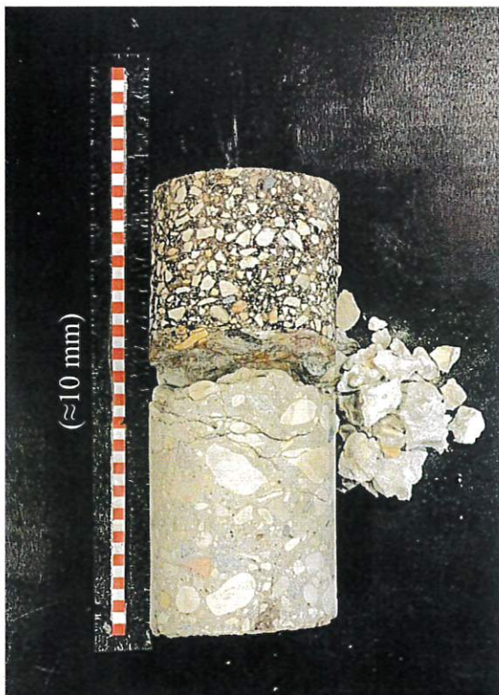
PC-20 Full Depth of Pavement Ø = 150 mm
