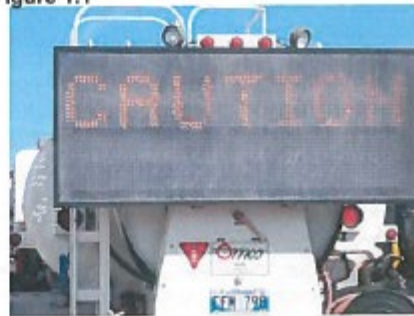
Figure 1.0 and 1.1: Tanker equipped with 4 beacons, retro-reflective striping and combined directional lighting/caution signage.
