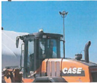
Figure 2.0: Articulating Loader with roof mounted dual function, amber/blue LED beacon.
