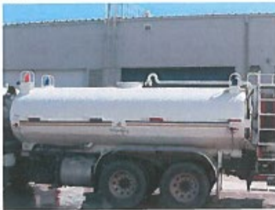
Figure 1.0 and 1.1: Tanker equipped with 4 beacons, retro-reflective striping and combined directional lighting/caution signage.
