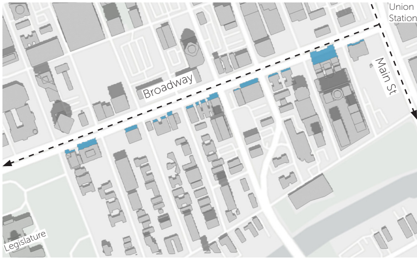
Figure 8. Summer solstice (December 22) shade study at 12 pm. Blue indicates shady spots, opportunities to encourage outdoor lunches on boulevard.
