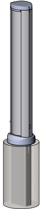
BASE TYPE B4 REMOVABLE FROM SLEEVE - PG. 13: BOLLARD IS REMOVABLE, POST IS SET PERMANENTLY INTO CONCRETE & PROTRUDES FROM SURFACE. BOLLARD SLIDES OVER POST & IS HELD IN PLACE WITH A PIN
