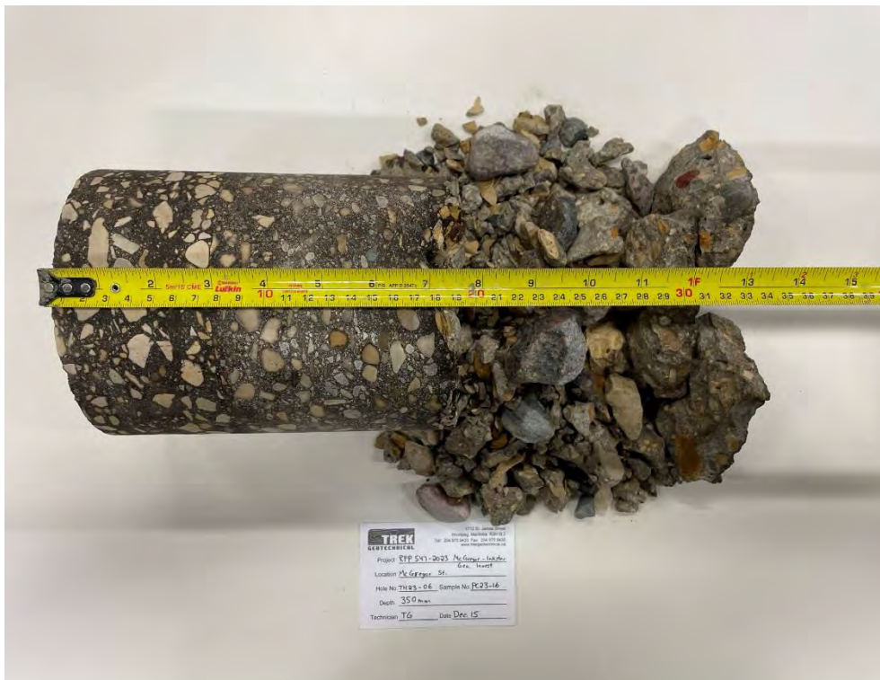
Photo 6: Pavement Core Sample at Test Hole TH23-06
