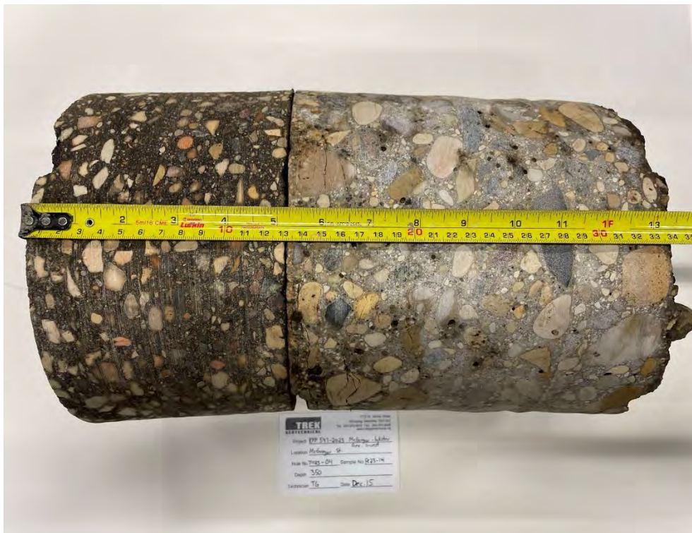
Photo 4: Pavement Core Sample at Test Hole TH23-04
