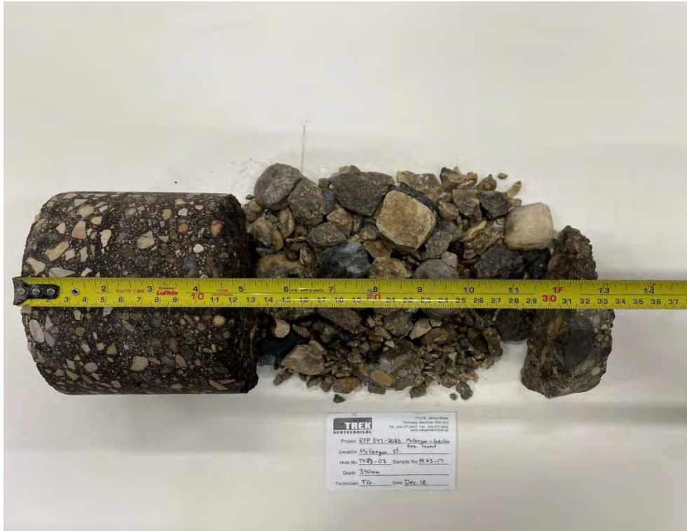
Photo 3: Pavement Core Sample at Test Hole TH23-03
