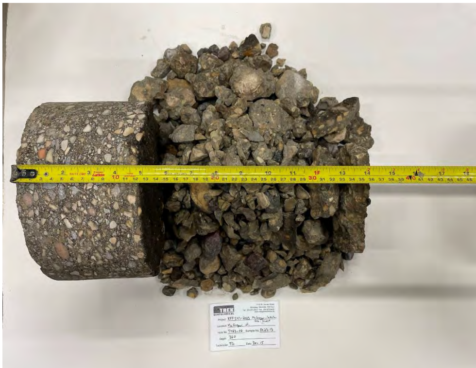
Photo 2: Pavement Core Sample at Test Hole TH23-02
