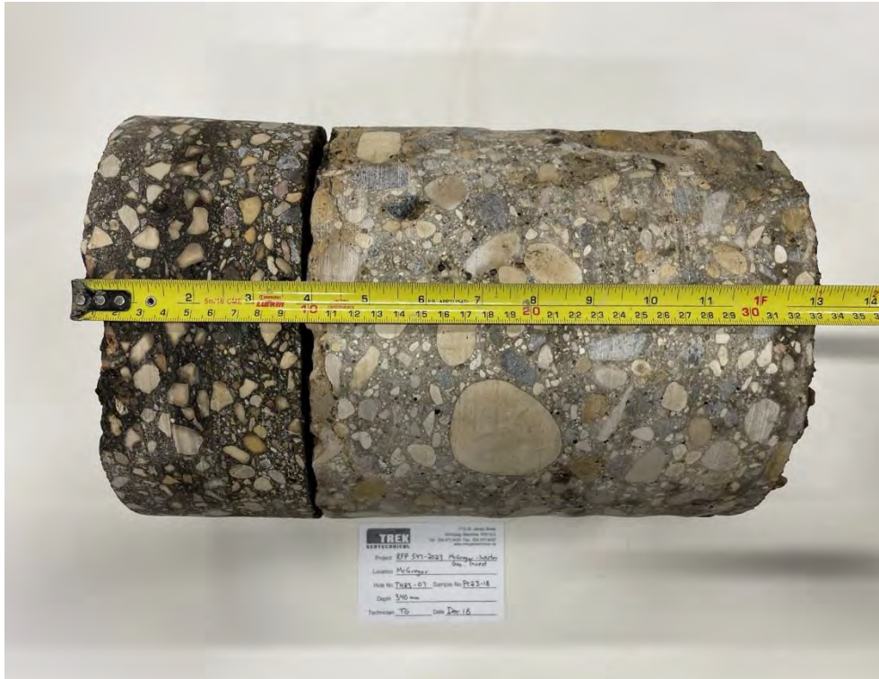
Photo 7: Pavement Core Sample at Test Hole TH23-07
