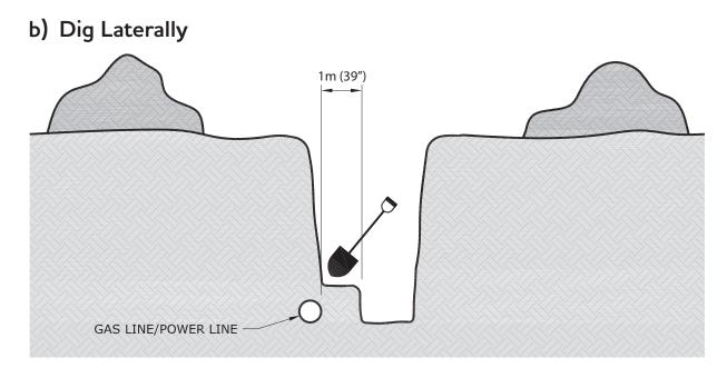
Dig a trench or bell hole 1 metre from the line location, parallel to the line, then hand dig laterally to expose the line.
